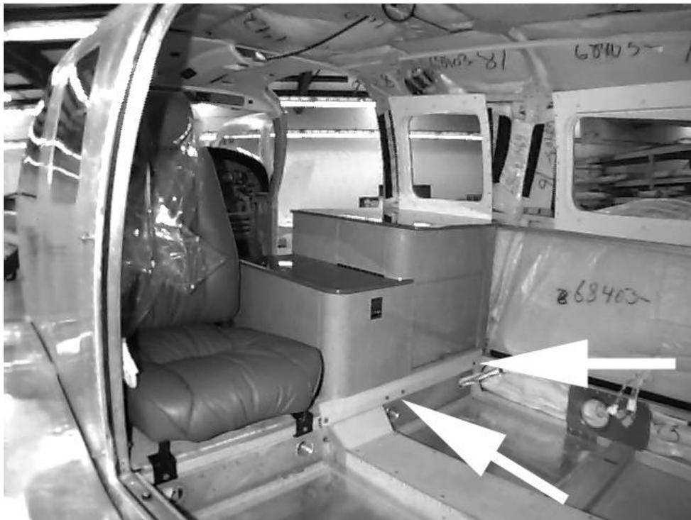
Figure 25-4. Console Mounting Bolts
