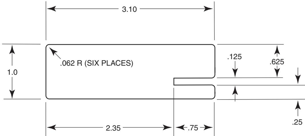
Figure 95-4. Fabricated Aileron Bellcrank Rigging Tool
