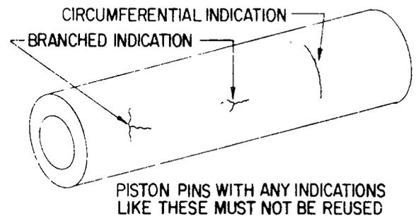
If any piston pins are found to have magnetic indications, the quantity of such pins and serial number of the engine from which they were removed should be promptly sent to Avco Lycoming by wire, or cable, collect, and ship the properly identified pins, via air shipment collect to Avco Lycoming and mark the package for the attention of the Service Department.
