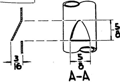
1. REMOVE BURRS THAT MAY BE FORMED AT END OF SAW SLOT.
