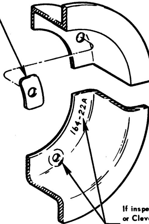
If inspection reveals .562 spot face, or Cleveland Aircraft Products Part No. 164-22A, no further action is required.
