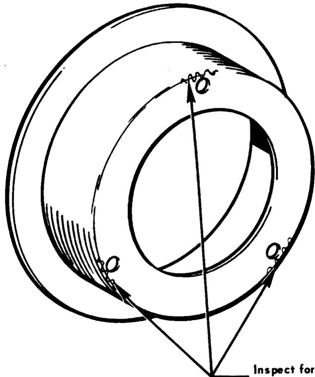
Inspect for cracks with 10 power glass or equivalent in these areas.
