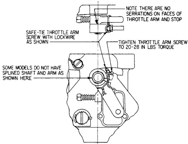
Figure 1. Previous Throttle Arm Configuration Showing Clamping Screw and Lockwire
