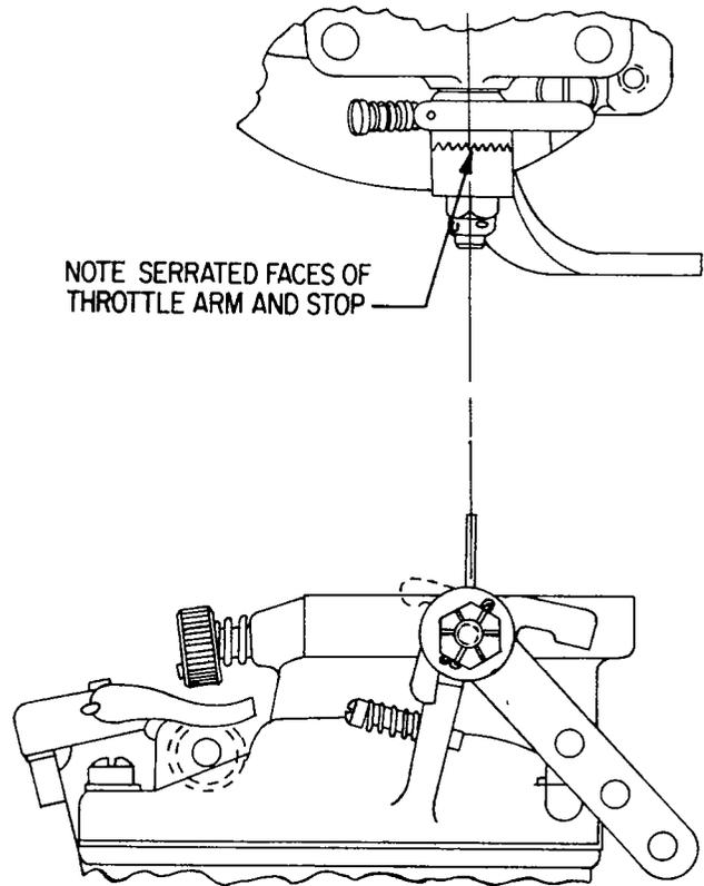
Figure 2. New Throttle Arm Configuration Showing Serrated Faces of Arm and Stop Levers
