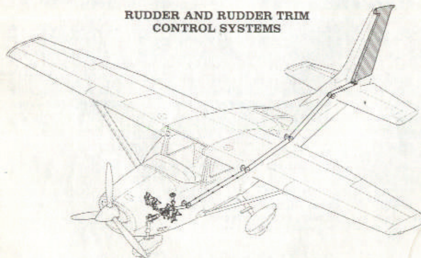
Figure 7-1. Flight Control and Trim Systems (Sheet 1 of 2)
