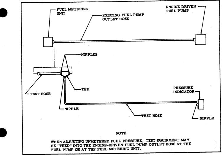
Figure 12-8. Fuel Injection Pump Adjustment Test Harness
