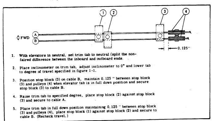
Figure 9-5. Elevator Trim Tab Travel Stop Adjustment
