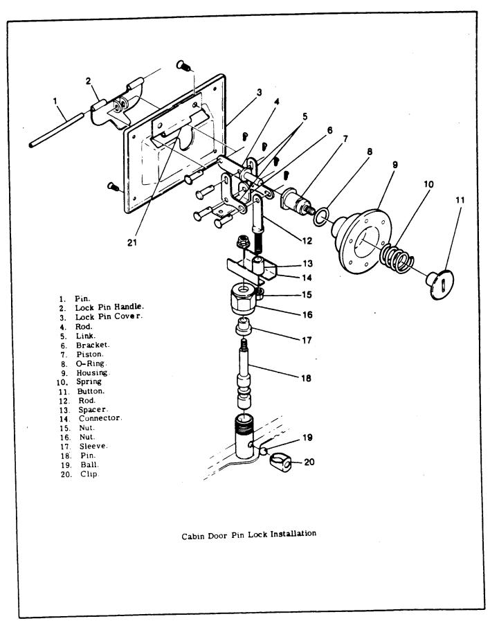
Figure 3-5. Door Latch Mechanism (Sheet 2 of 4).
