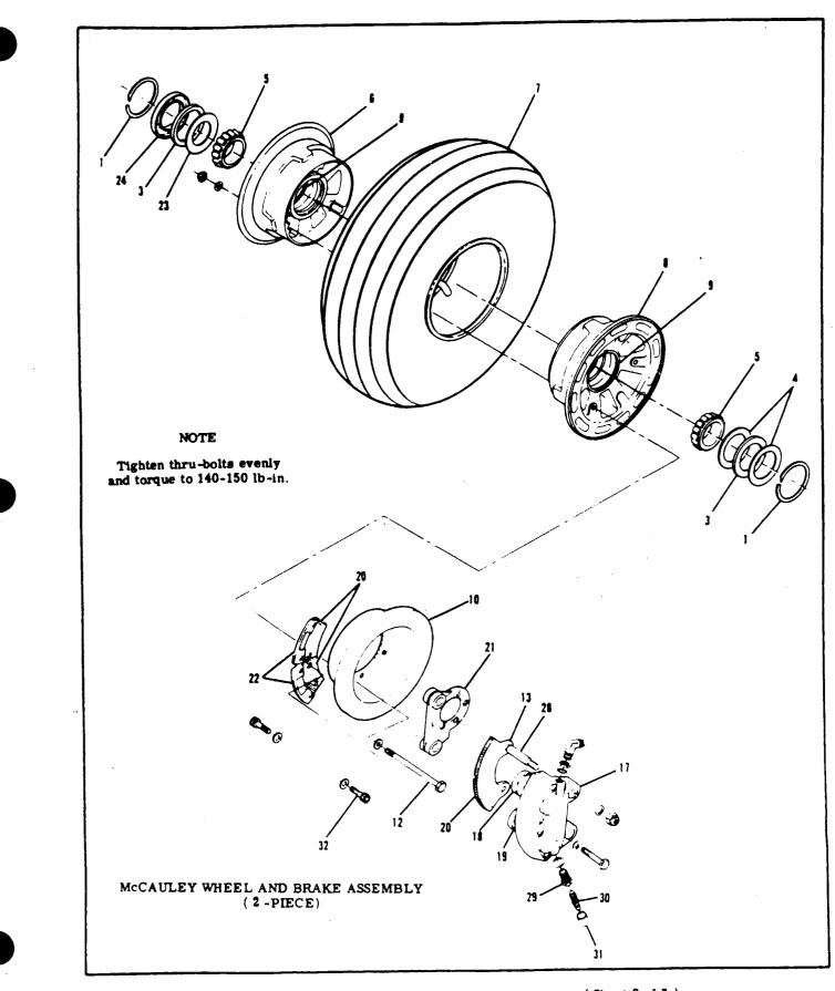
Figure 5-10 Main Landing Gear, Tire and Brake Assembly (Sheet 2 of 3 )
