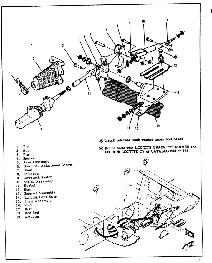
Figure 5-6. Main Landing Gear Downlock Installation
