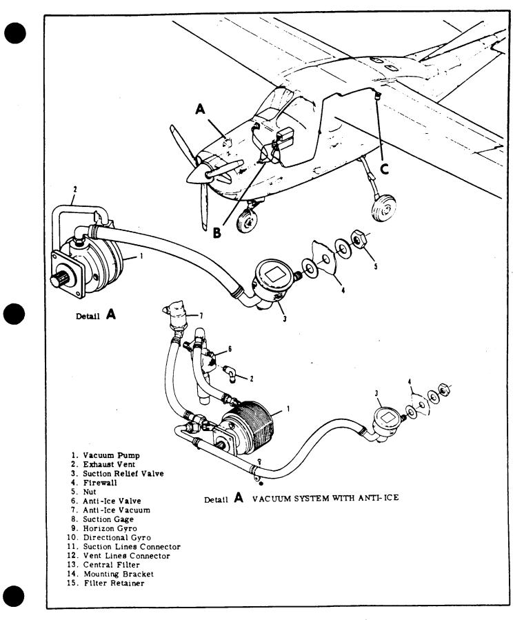
Figure 16-4. Vacuum System (Sheet 1 of 3)
