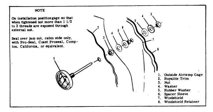
Figure 16-8. Outside Air Temperature Gage
