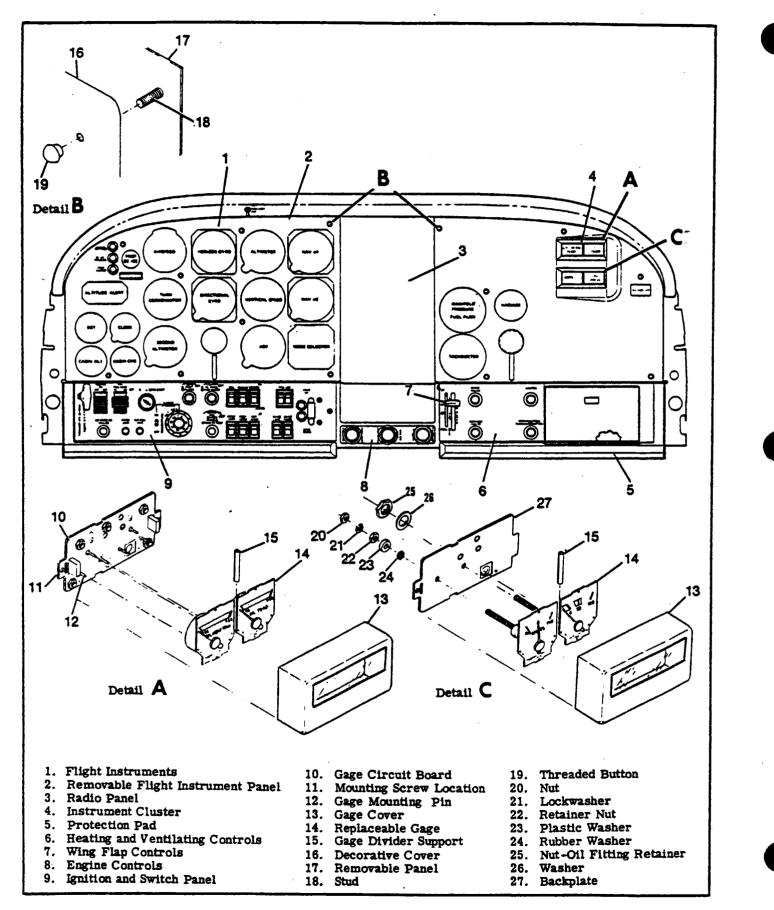
Figure 16-1. Instrument Panel (Typical)
