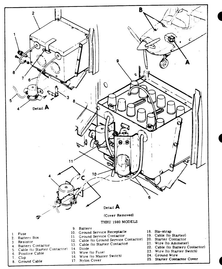
Figure 17-2. Battery and Electrical Equipment Installation (Sheet 1 of 4)
