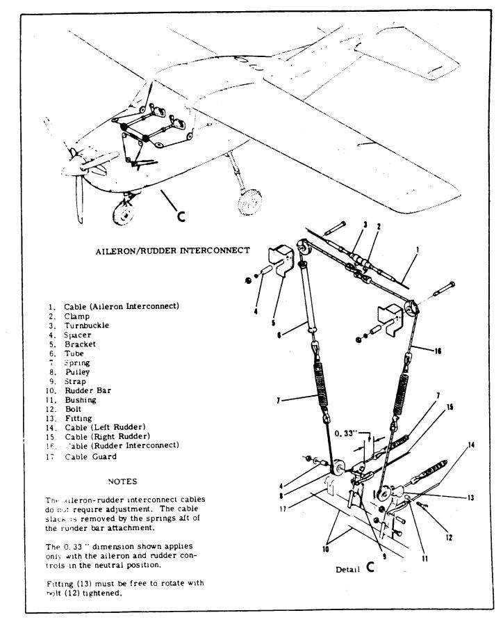
Figure 6-2. Control Column Installation (Sheet 5 of 5)
