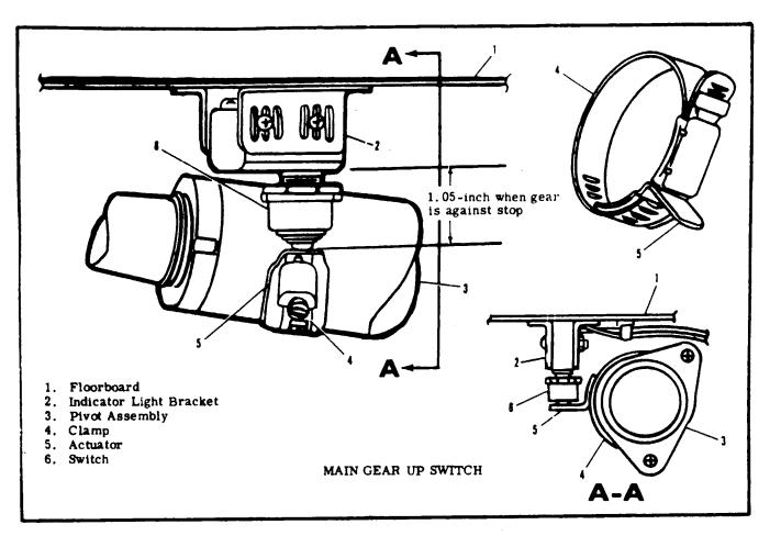
Figure 5A-10. Rigging Main Landing Gear (Sheet 3 of 3)
