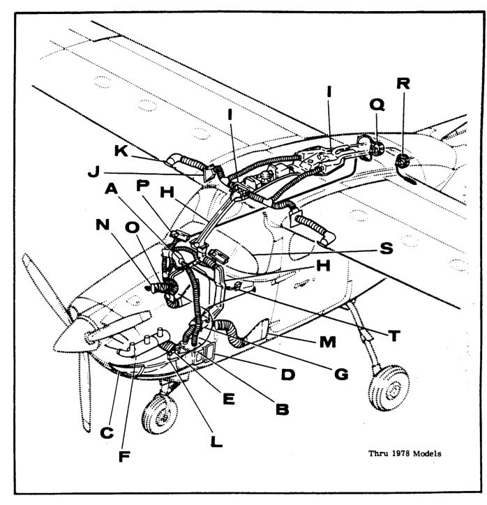
Figure 15-1. Heating, Ventilating and Pressurization System (Sheet 1 of 5)
