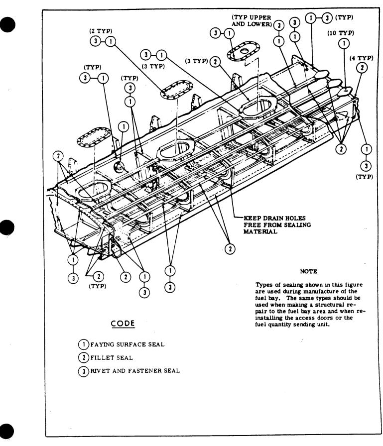
Figure 13-4. Fuel Bay Sealing (Sheet 1 of 2)
