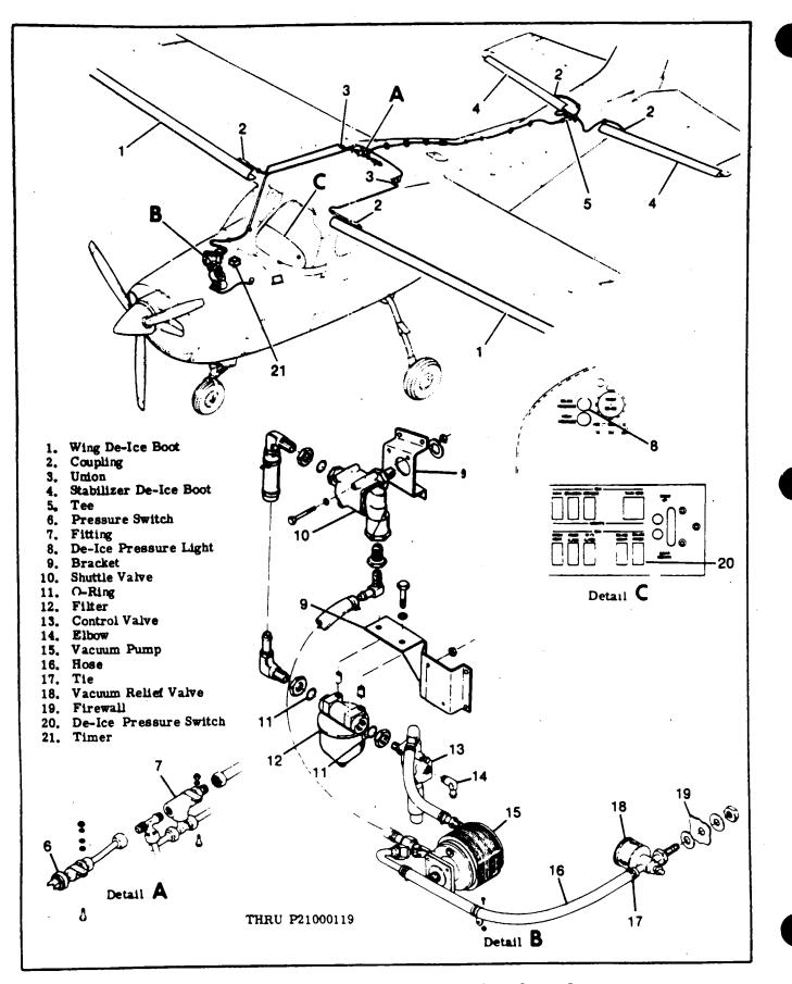
Figure 15-3. Wing and Horizontal Stabilizer One-Cycle De-ice System
