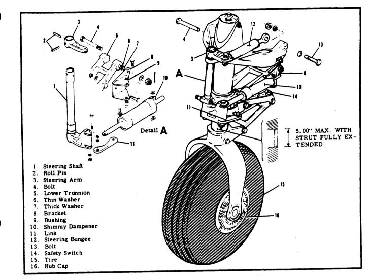
Figure 5-15. Nose Gear Installation
