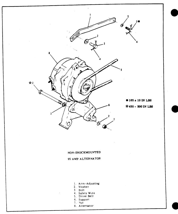
Figure 17-4. Alternator Installation (Sheet 3 of 3)
