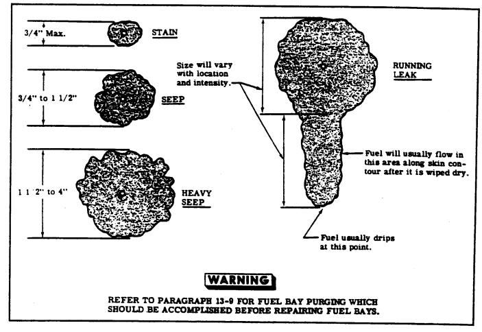
Figure 13-3. Classification of Fuel Leaks.
