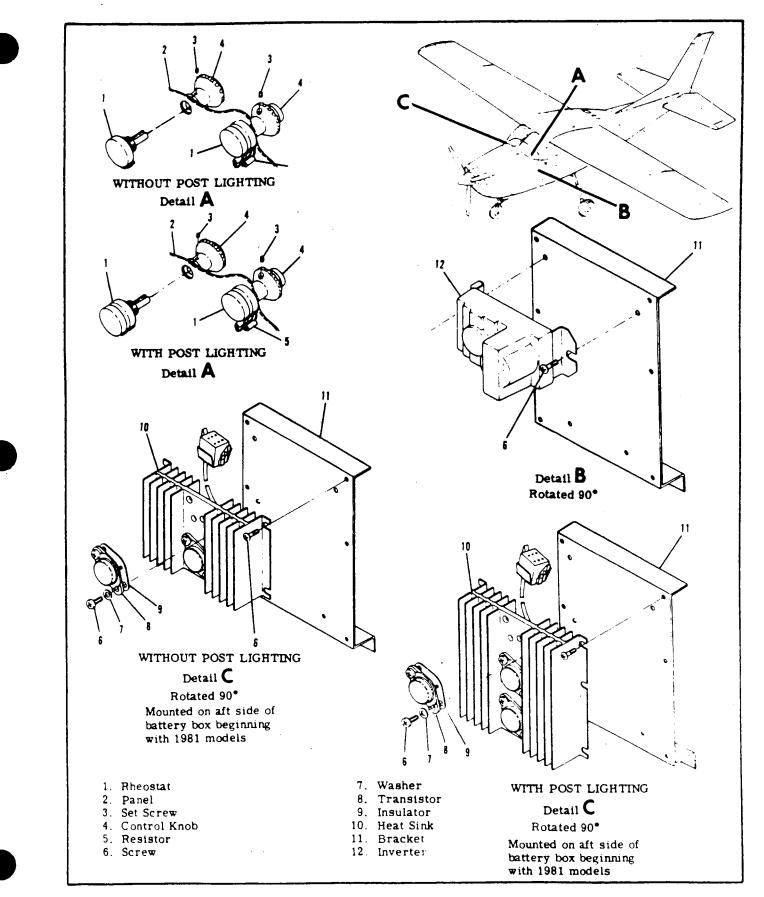
Figure 17-12. Transistorized Light Dimming and Electroluminescent Inverter Installation
