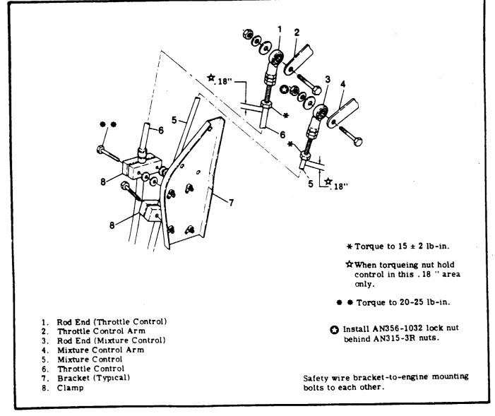
Figure 12-12. Engine Controls
