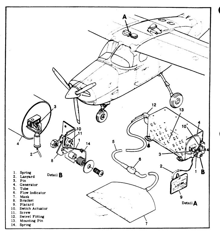
Figure 15-7. Emergency Oxygen System.
