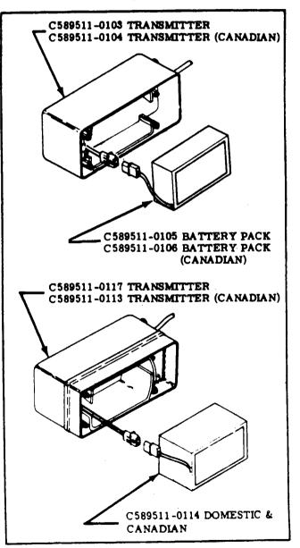
Figure 17-23. Battery Pack Installation.
