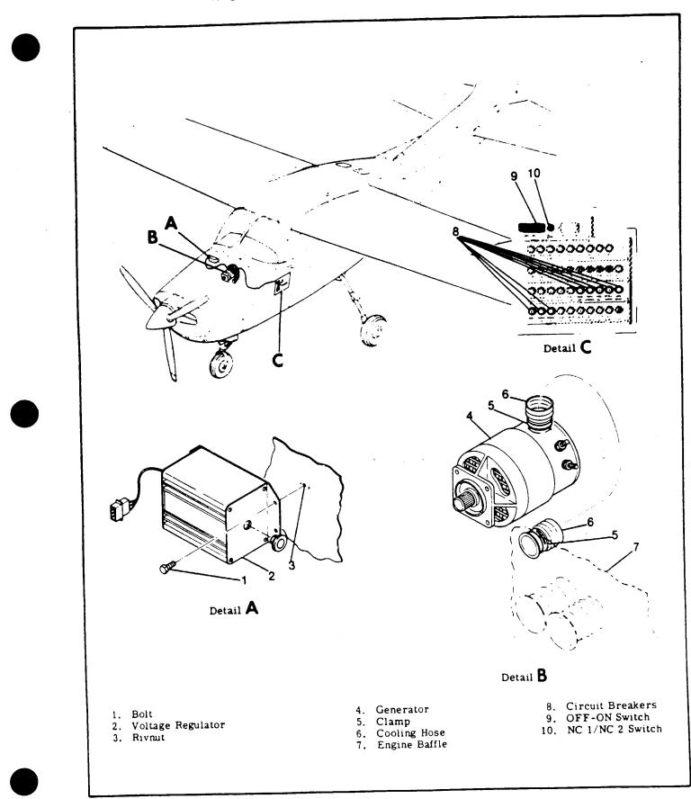
Figure 17-6A. Standby Generator System Installation.
