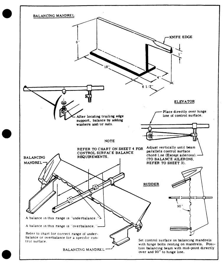
Figure 18-2. Control Surface Balancing (Sheet 1 of 4).
