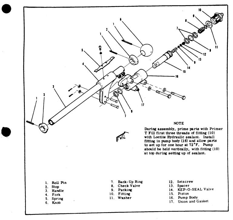
Figure 5-31. Landing Gear Hand Pump
