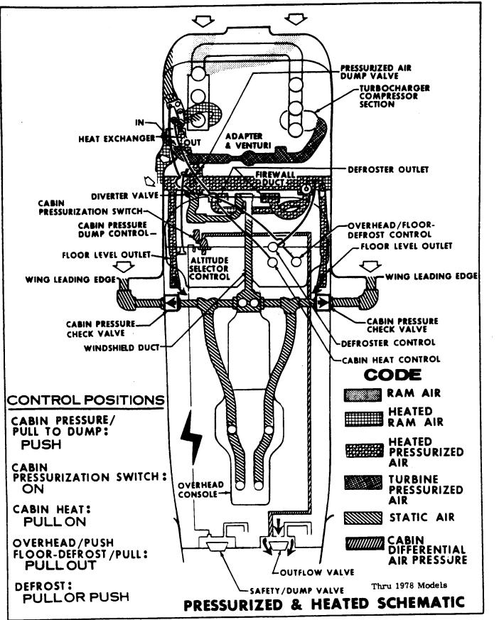
Figure 15-2. Cabin Air Flow Schematic (Sheet 3 of 6)
