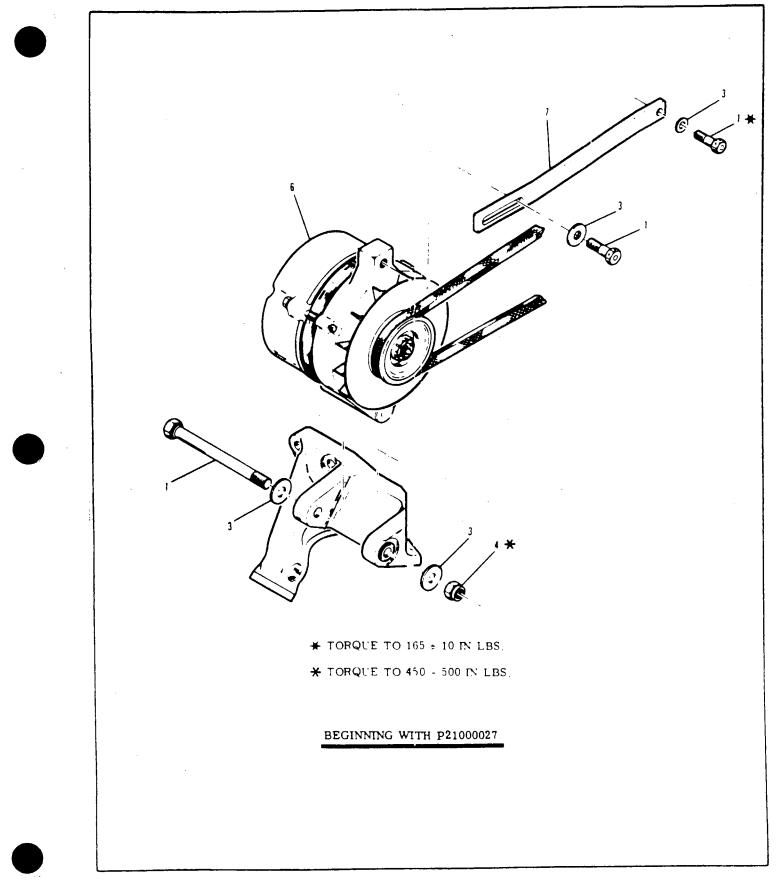
Figure 17-4. Alternator Installation (Sheet 2 of 3)
