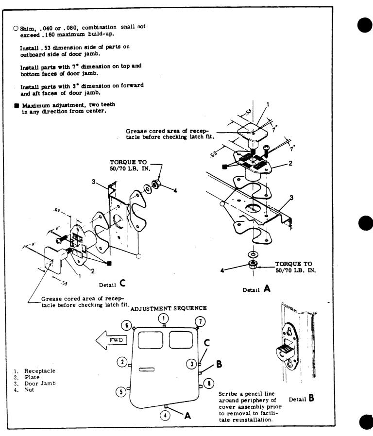
Figure 3-5A. Main Door Receptacle Installation (Sheet 2 of 2).
