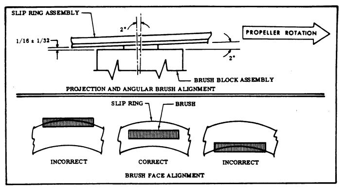
Figure 15-6. Brush Face Alignment and Projection and Angular Brush Alignment
