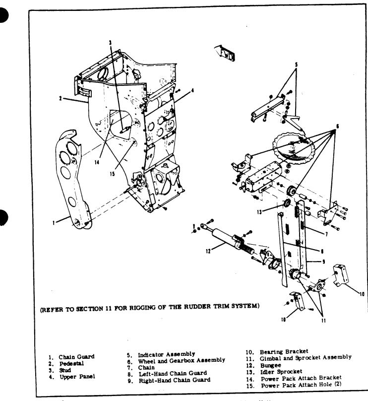
Figure 5-26. Power Pack Removal and Installation
