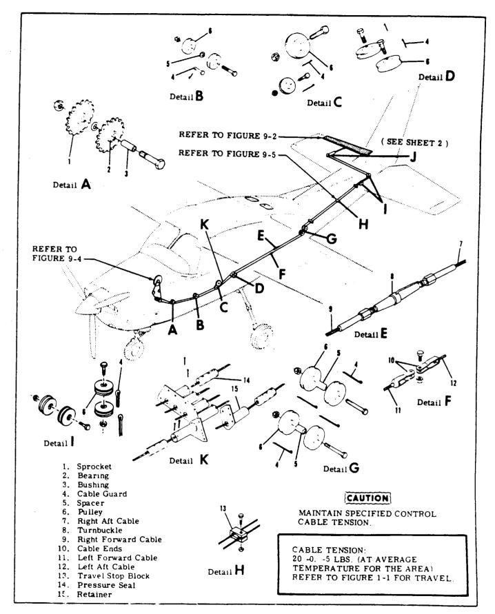
Figure 9-1. Elevator Trim Tab Control System (Sheet 1 of 2)
