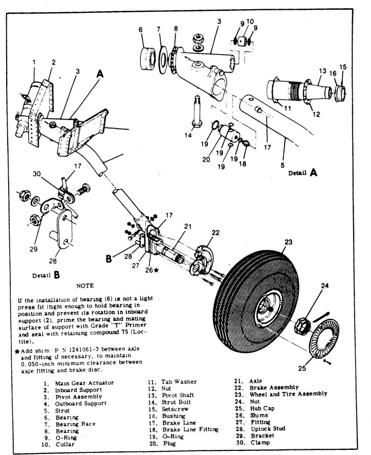
Figure 5-1 Main Landing Gear Installation.
