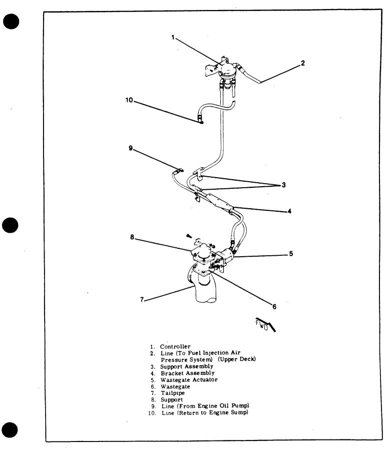
Figure 12-16. Controller and Waste-Gate Installation
