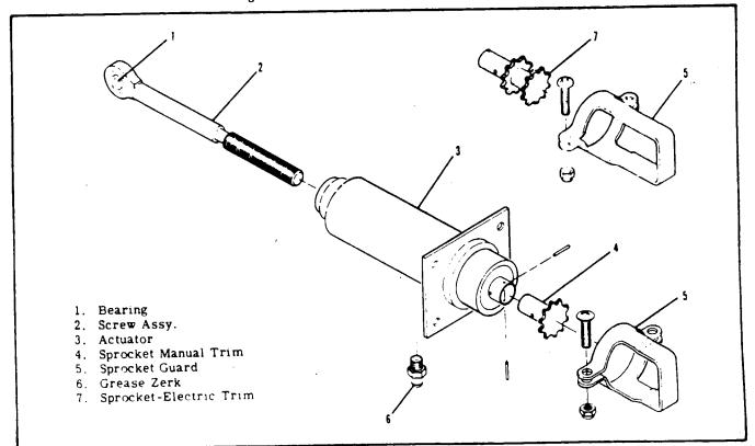
Figure 9-3. Elevator Trim Tab Actuator Assembly
