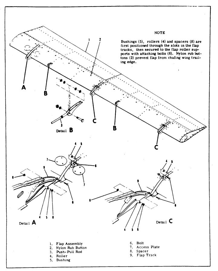
Figure 7-2. Flap Installation
