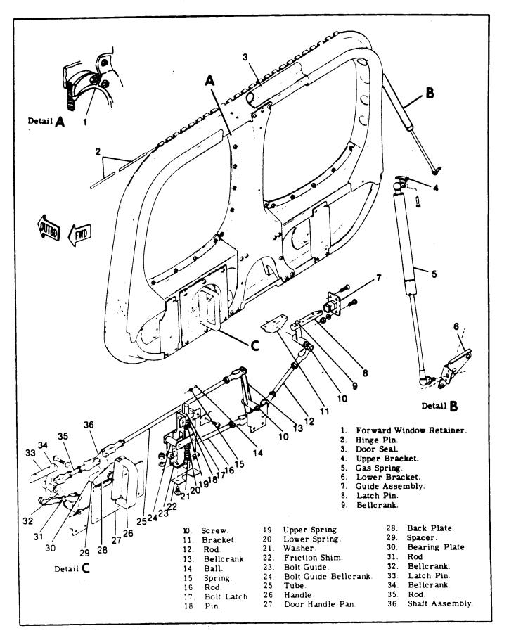
Figure 3-6. Emergency Exit Door Installation (Sheet 2 of 2).
