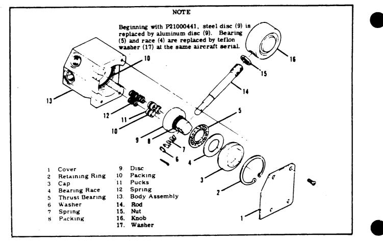
Figure 5A-7. Landing Gear Position Selector Valve
