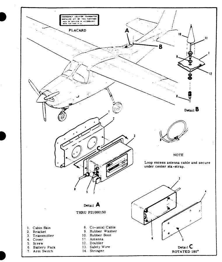
Figure 17-22. Emergency Locator Transmitter Installation (Sheet 1 of 3)
