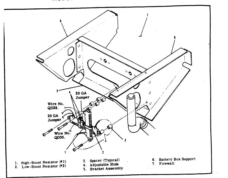
Figure 13-8. Auxiliary Fuel Pump Resistors
