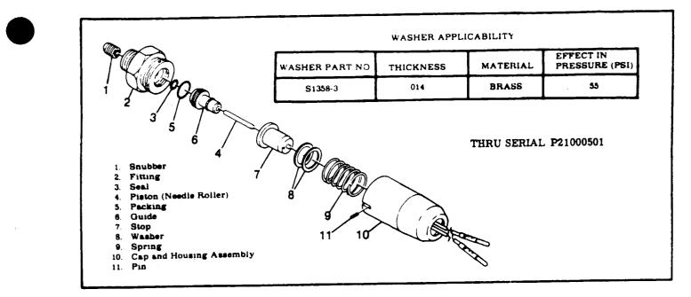
Figure 5A-5. Pressure Switch
