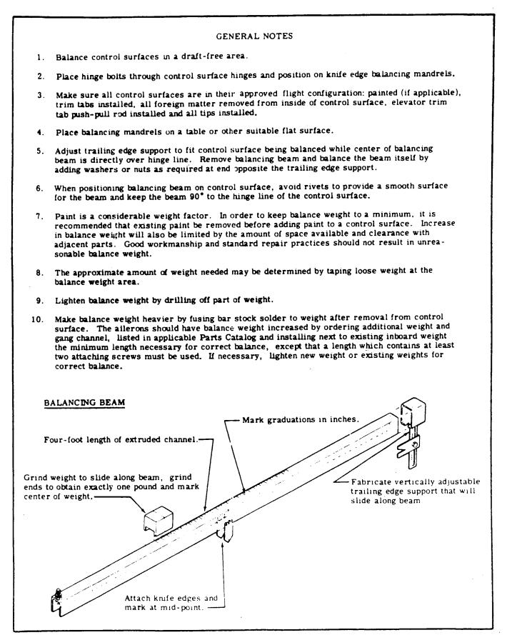
Figure 18-2. Control Surface Balancing (Sheet 3 of 4).
