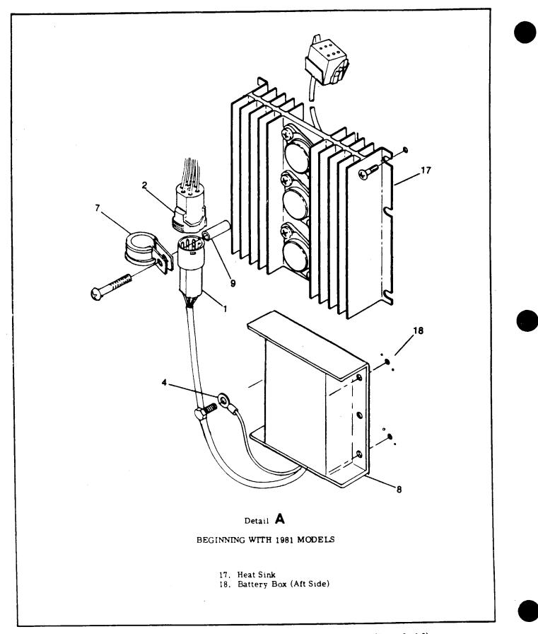
Figure 17-5. Voltage Regulator Alternator Control Unit Installation (Sheet 3 of 3)
