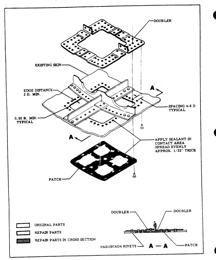
Figure 18-11. Over Structure Repair of Pressure Cabin
