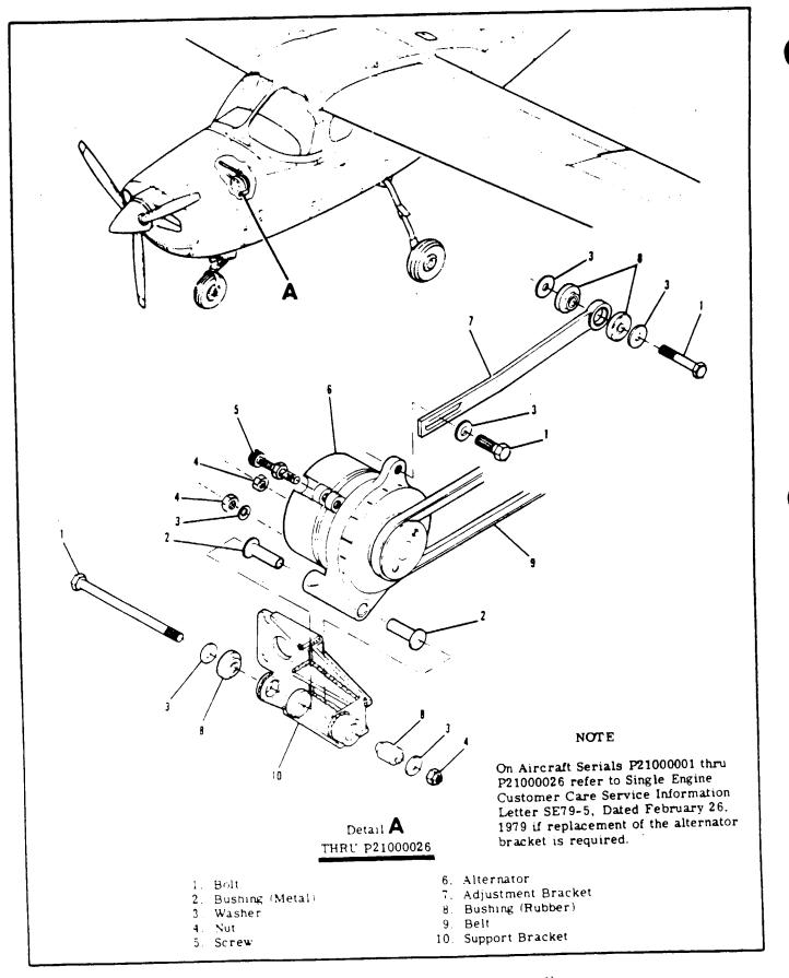
Figure 17-4. Alternator Installation (Sheet 1 of 3)
