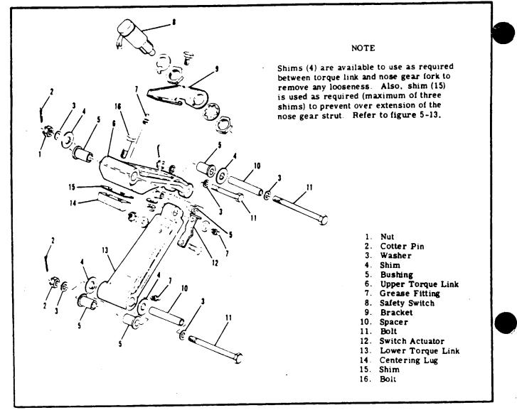
Figure 5-18. Nose Gear Torque Links
