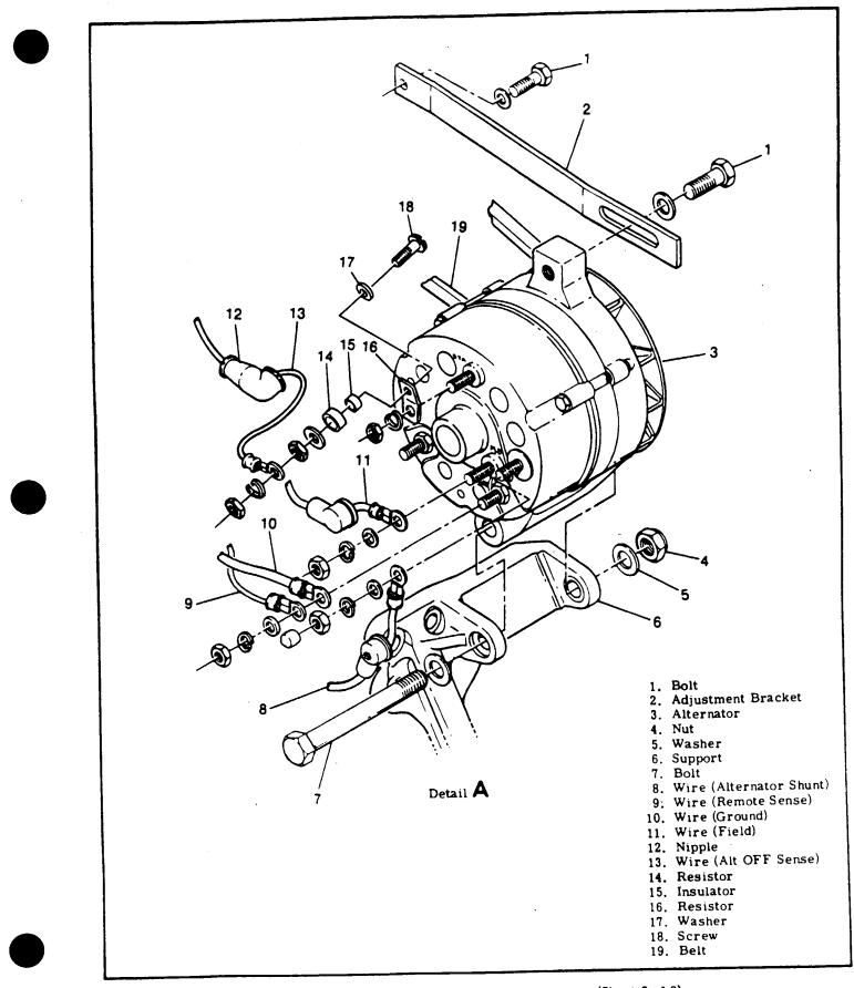
Figure 17-6B. Dual Alternator System Installation (Sheet 2 of 8)
