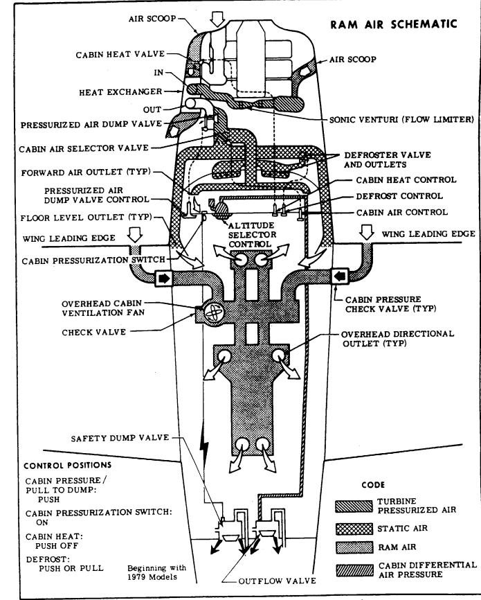
Figure 15-2. Cabin Air Flow Schematic (Sheet 4 of 6)
