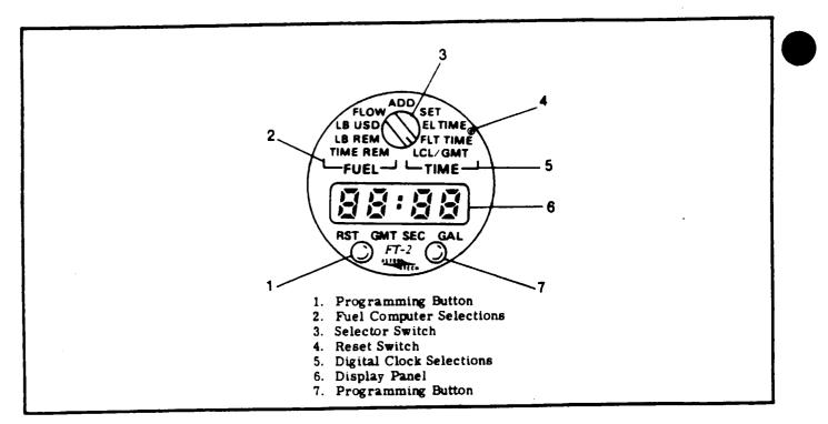
Figure 16-9. Fuel Computer/Digital Clock.
