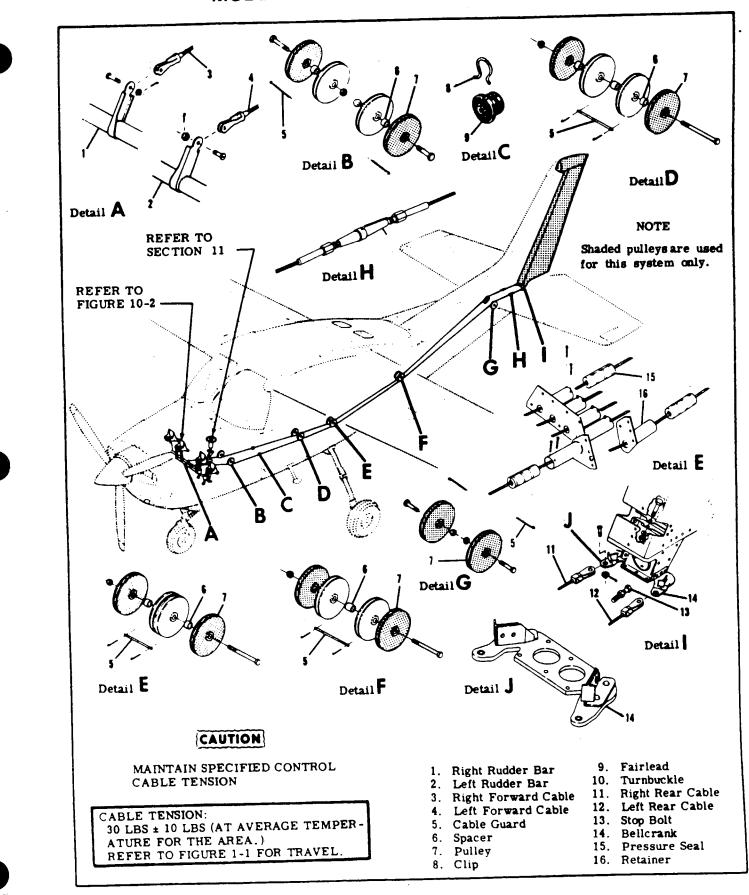
Figure 10-1. Rudder Control System
