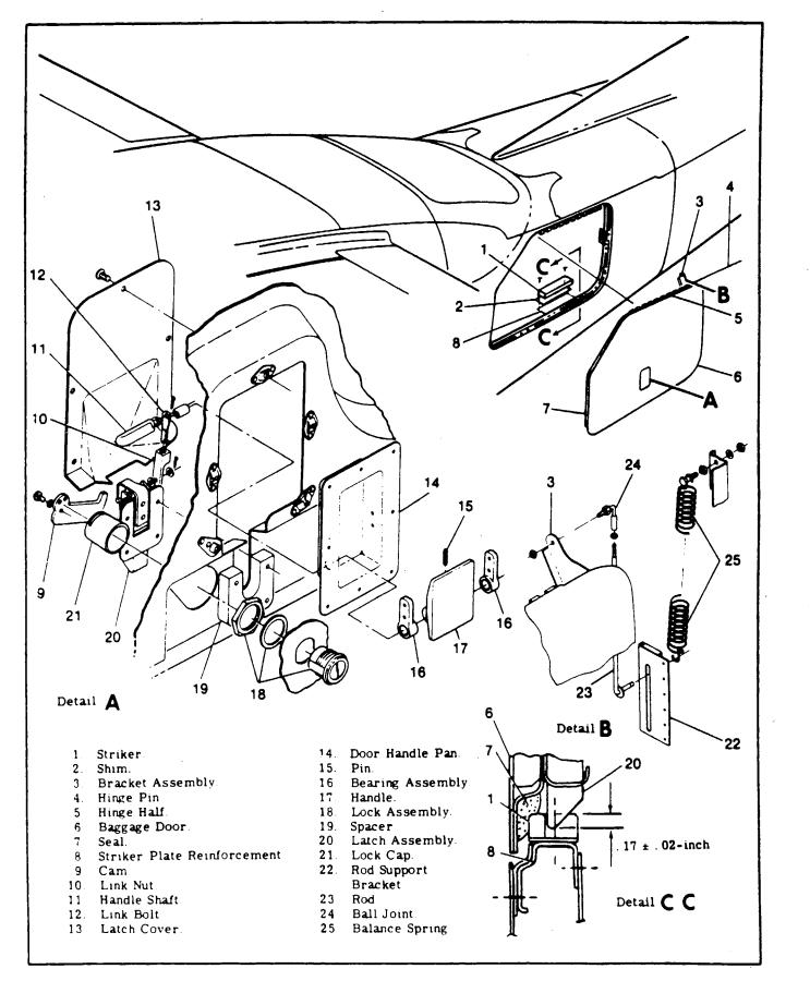
Figure 3-7A. Baggage Door Installation
