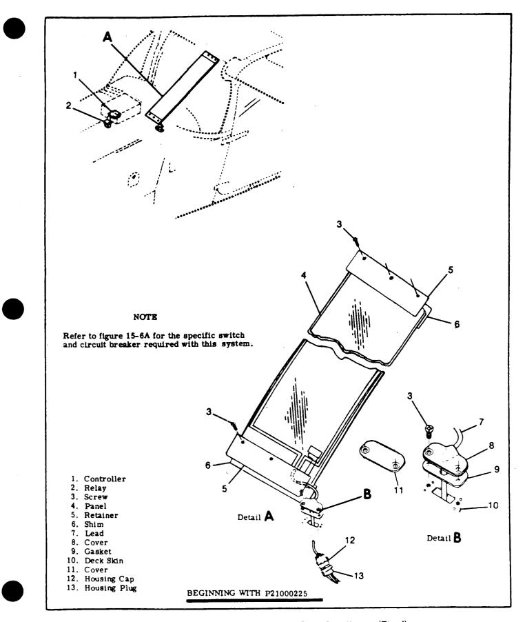
Figure 15-6C. Windshield Anti-Ice Panel Installation (Fixed)
