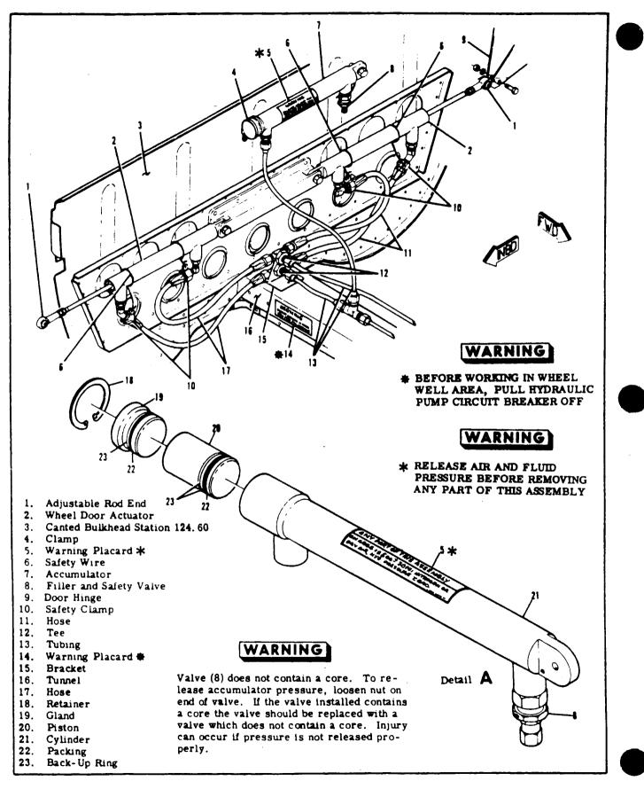
Figure 5-11. Main Landing Gear Wheel Door Close System Accumulator
