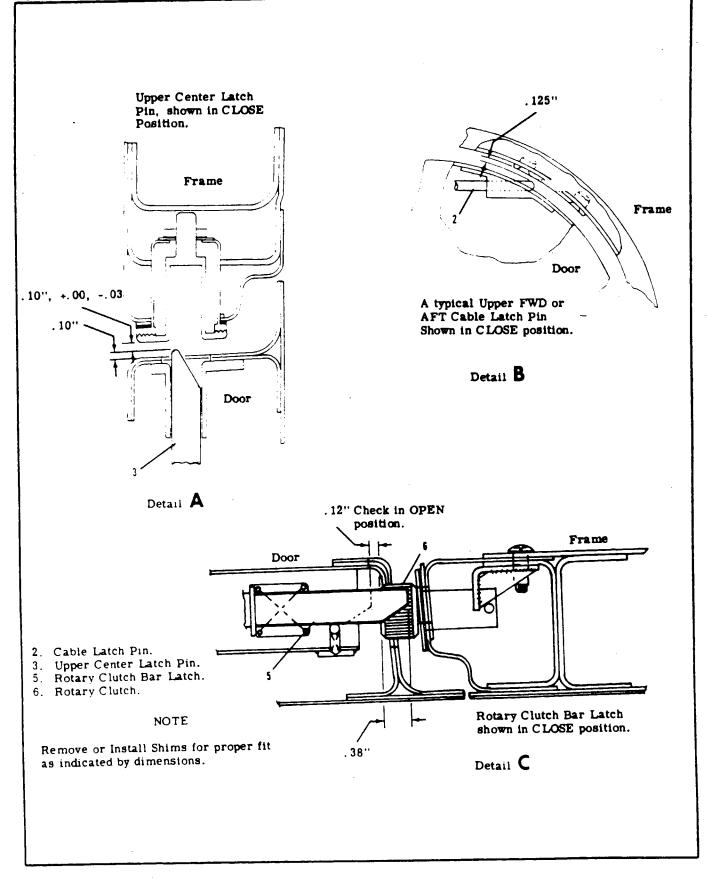
Figure 3-5. Door Latch Mechanism (Sheet 4 of 4).
