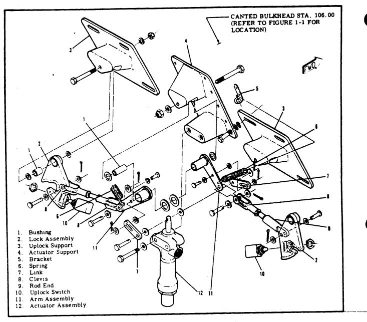
Figure 5-4. Main Landing Gear Uplock Installation
