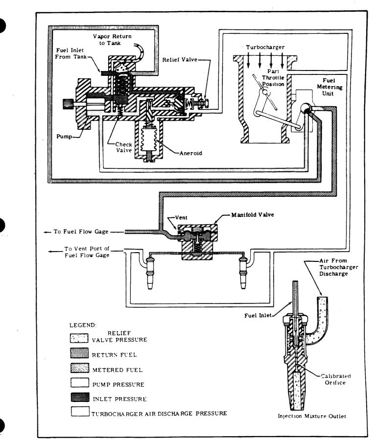
Figure 12-6. Fuel System Schematic
