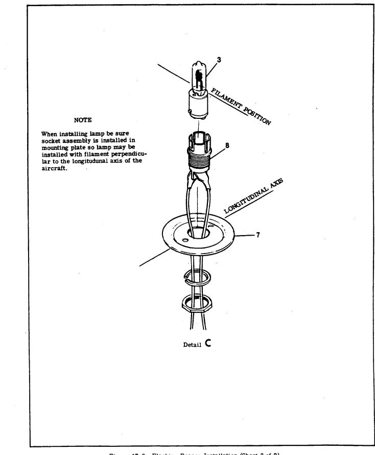
Figure 17-9. Flashing Beacon Installation (Sheet 2 of 2)
