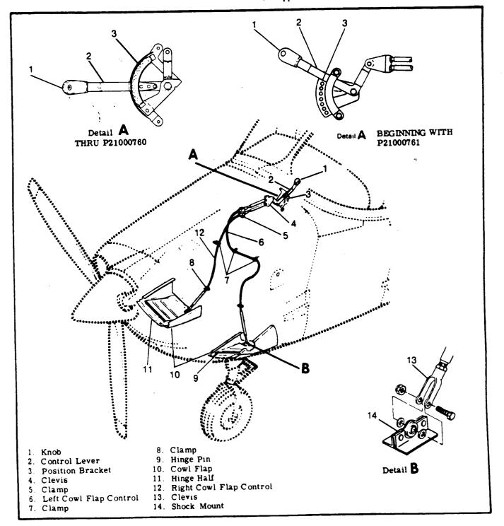
Figure 12-1. Cowl Flaps Installation
