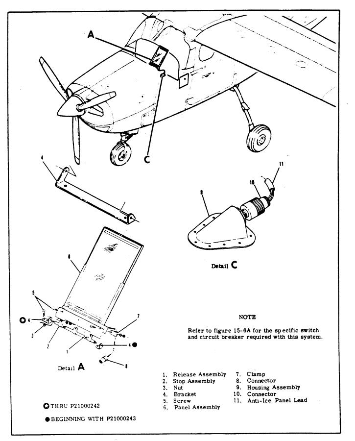
Figure 15-6B. Windshield Anti-Ice Panel Installation (Removable)
