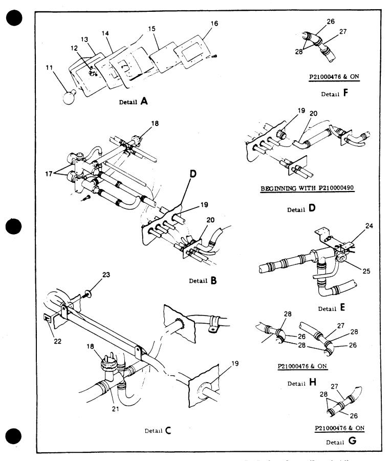
Figure 15-4A. Wing, Horizontal Stabilizer and Vertical Fin De-Icing System (Sheet 2 of 5)
