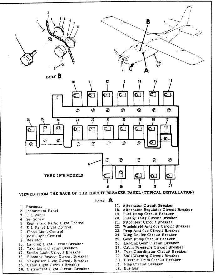
Figure 17-1. Bus Bar and Circuit Breaker Installation (Sheet 1 of 4)
