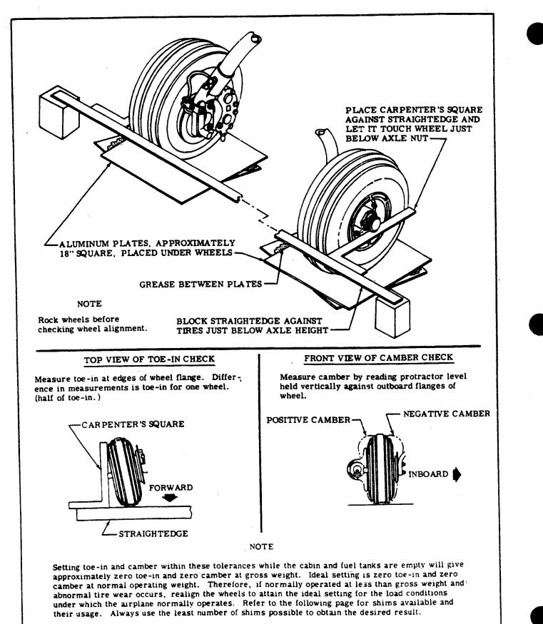
Figure 5A-11 Wheel Alignment (Sheet 1 of 2)
