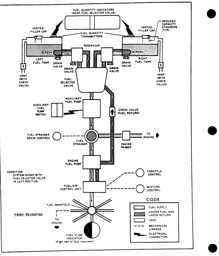
Figure 13-1. Fuel System Schematic
