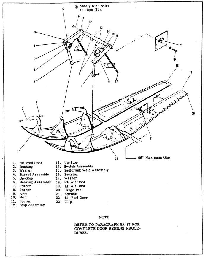
Figure 5A-13. Nose Gear Doors
