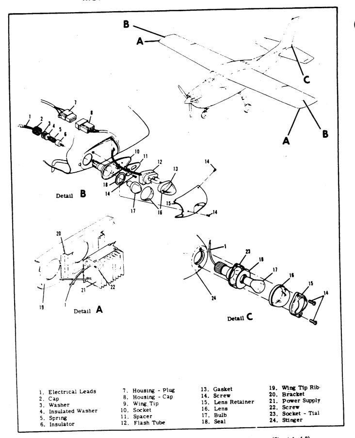
Figure 17-8. Navigation, Flood and Anti-Collision Strobe Lights Installation (Sheet 1 of 2)
