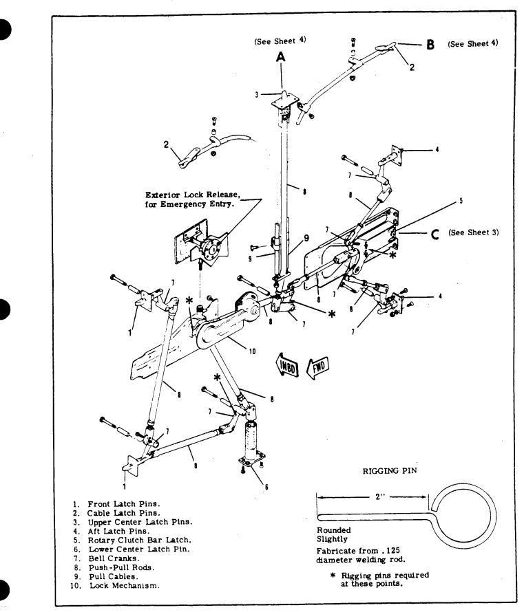
Figure 3-5. Door Latch Mechanism (Sheet 1 of 4)
