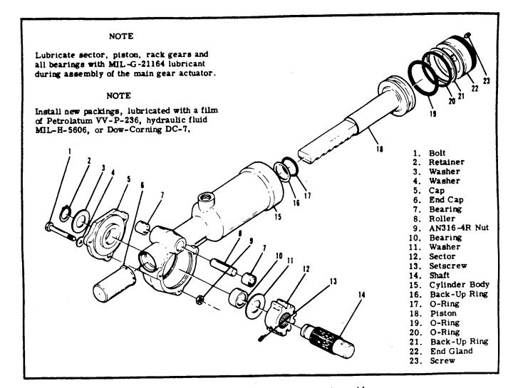
Figure 5-2. Main Landing Gear Actuator Assembly
