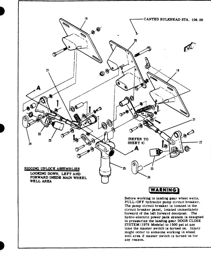
Figure 5-36. Rigging Main Landing Gear (Sheet 3 of 4)
