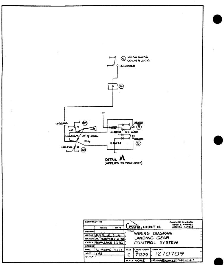
Landing Gear Control System (Sheet 2 of 2)
