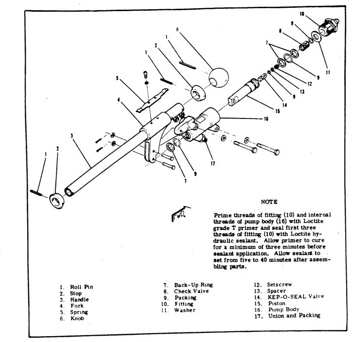
Figure 5A-6. Emergency Hand Pump Disassembly
