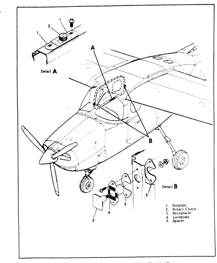
Figure 3-6. Emergency Exit Door Installation (Sheet 1 of 2).
