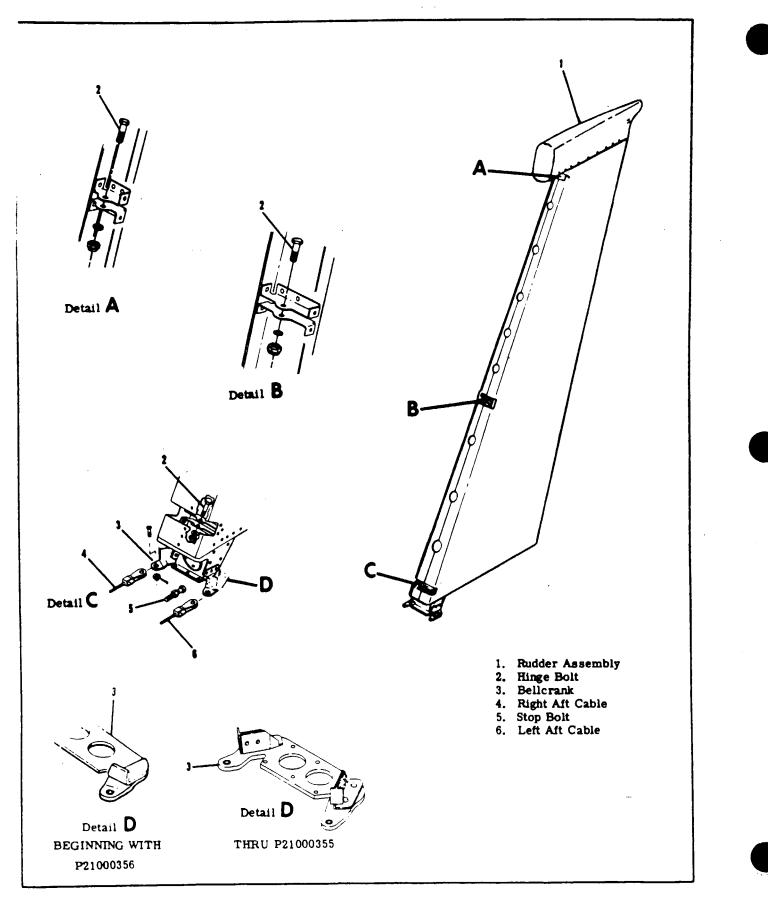
Figure 10-4. Rudder Installation
