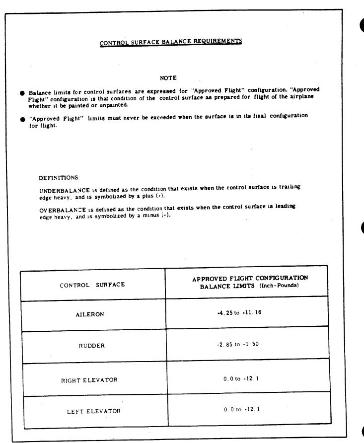
Figure 18-2. Control Surface Balancing (Sheet 4 of 4).
