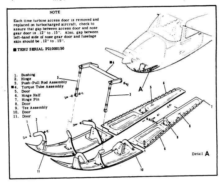
Figure 5-22. Nose Gear Door System
