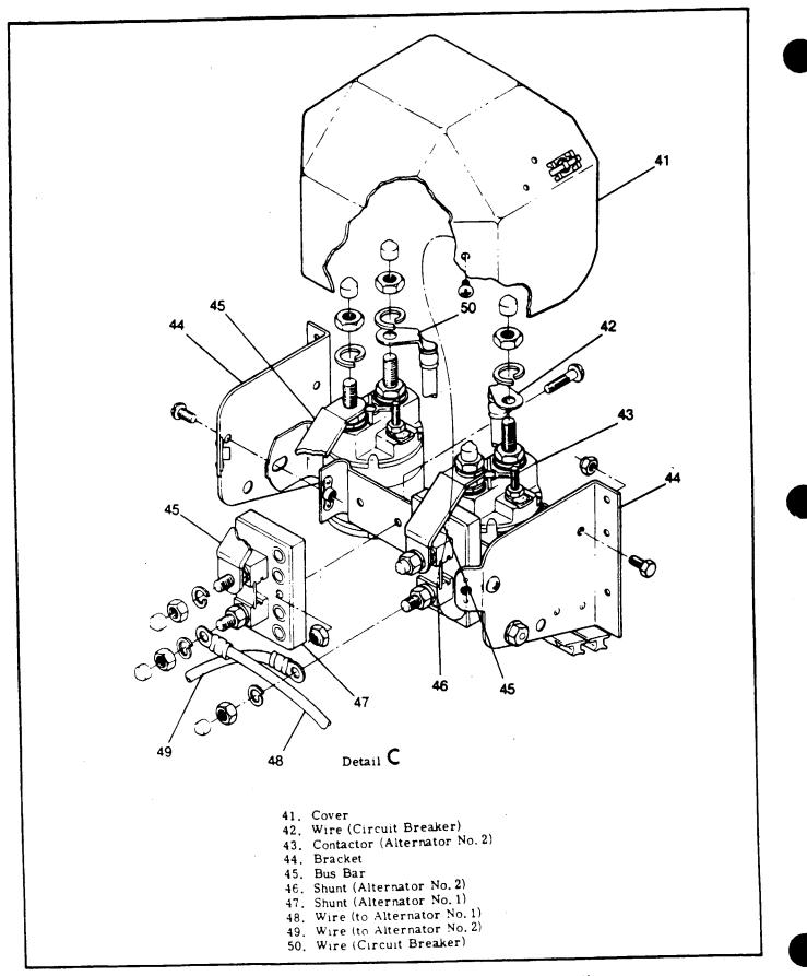
Figure 17-6B. Dual Alternator System Installation (Sheet 5 of 8)
