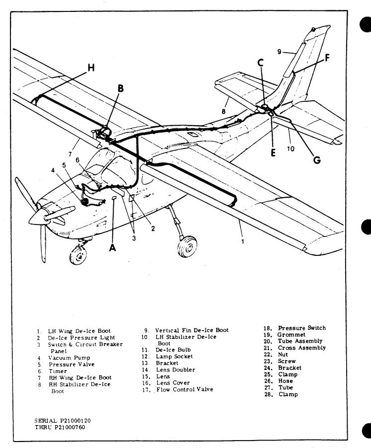
Figure 15-4A. Wing, Horizontal Stabilizer and Vertical Fin De-Icing System (Sheet 1 of 5)
