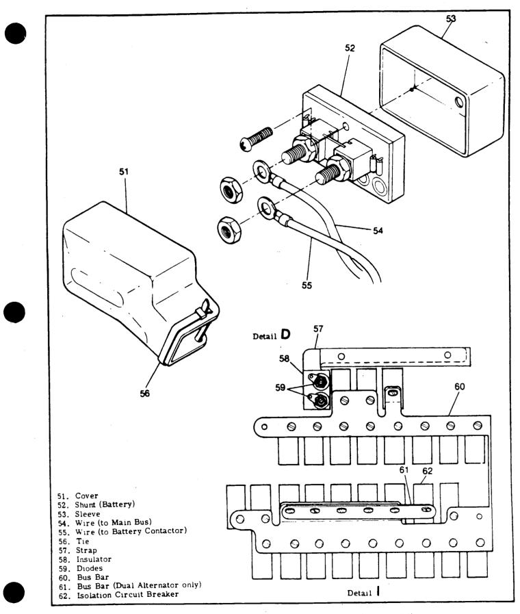
Figure 17-6B. Dual Alternator System Installation (Sheet 6 of 8)
