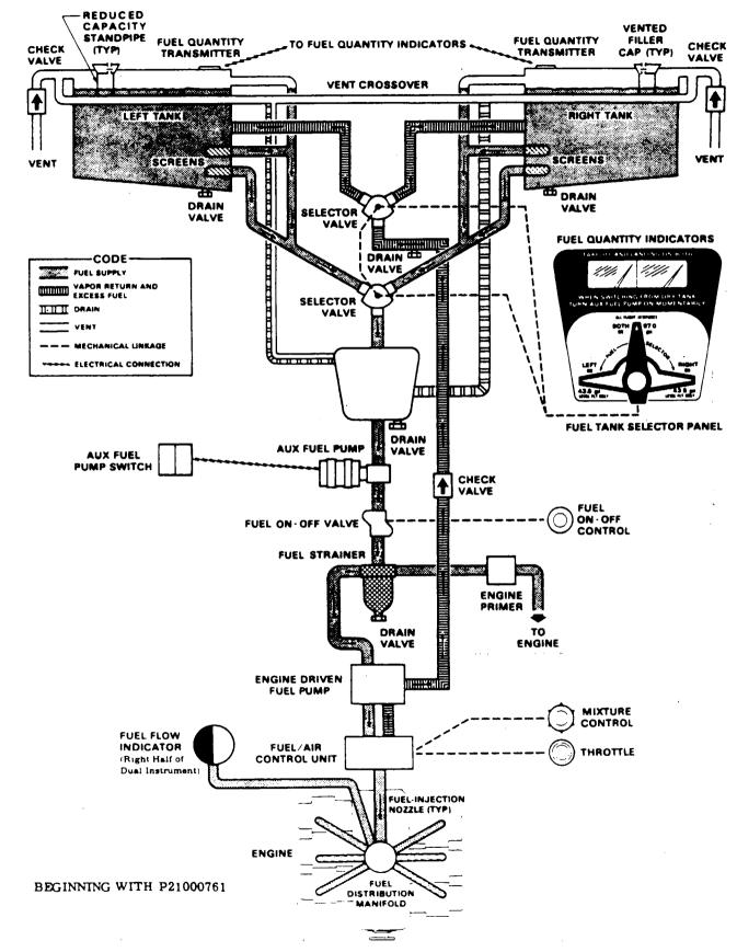
Figure 13-10. Fuel System Schematic
