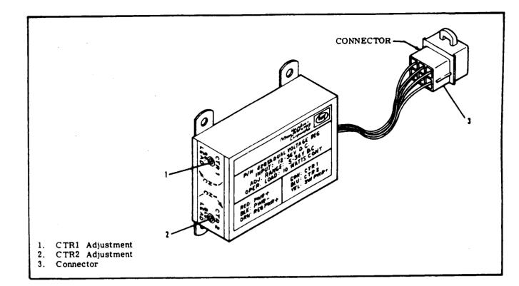
Figure 9-7. Dual Voltage Regulator
