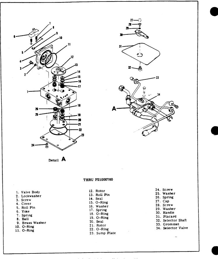
Figure 13-6. Fuel Selector Valve Assembly
