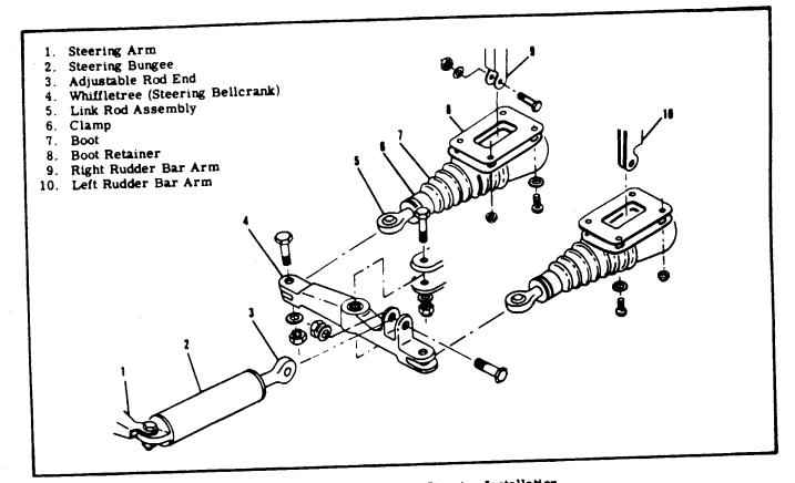
Figure 10-3. Nose Gear Steering Installation
