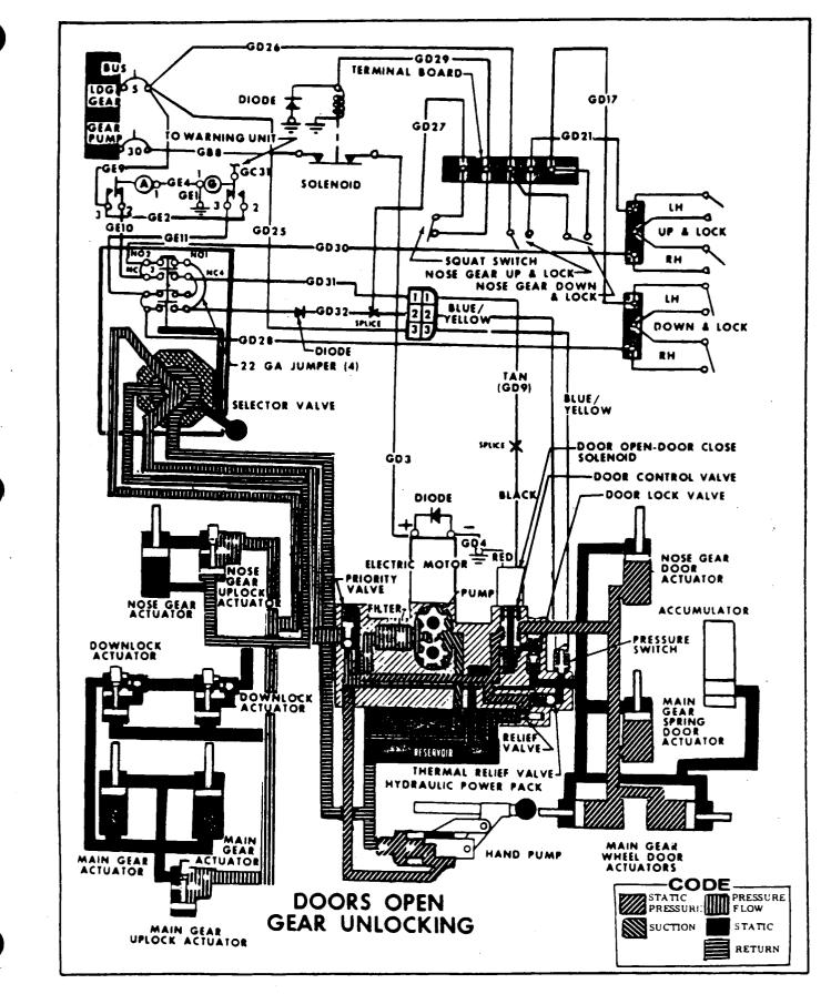
Figure 5-38. Hydraulic and Electrical System Schematic (Sheet 3 of 7)
