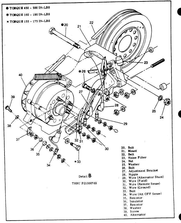
Figure 17-6B. Dual Alternator System Installation (Sheet 3 of 8)
