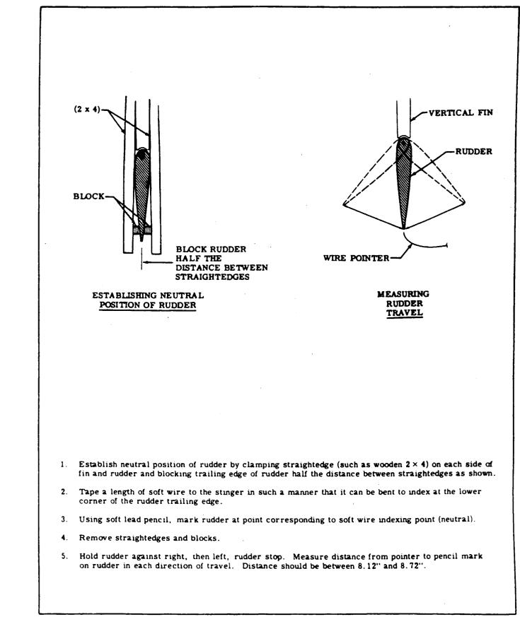
Figure 10-5. Checking Rudder Travel
