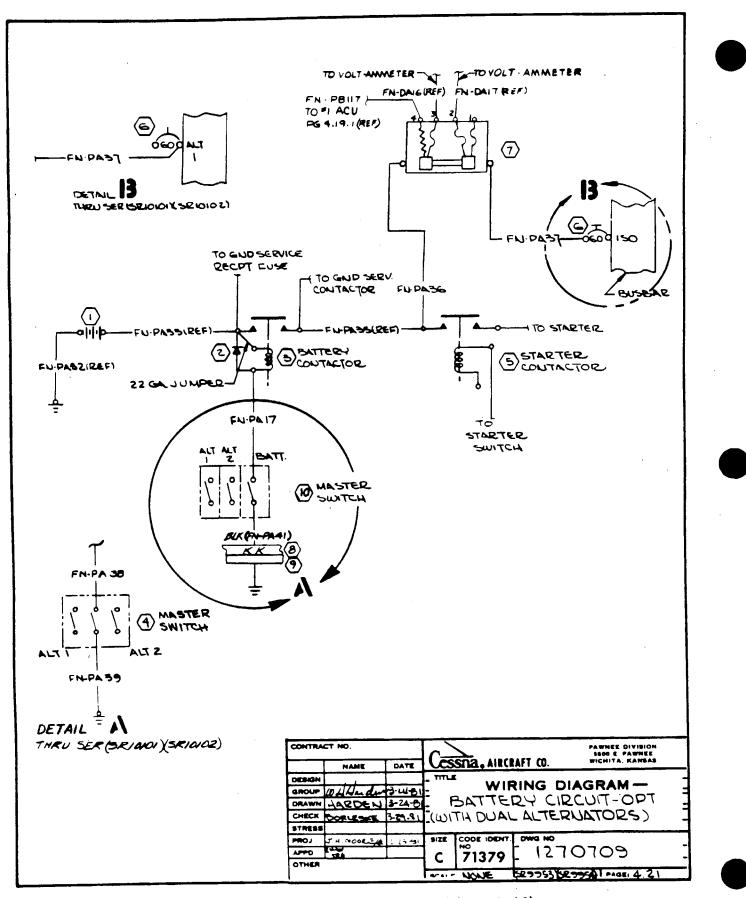
Battery Circuit-OPT (With Dual Alternators) (Sheet 2 of 2)
