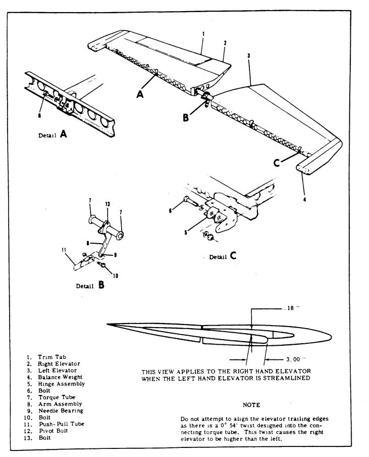
Figure 8-2. Elevator Installation
