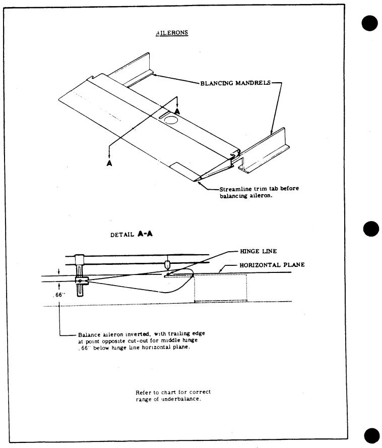
Figure 18-2. Control Surface Balancing (Sheet 2 of 4).
