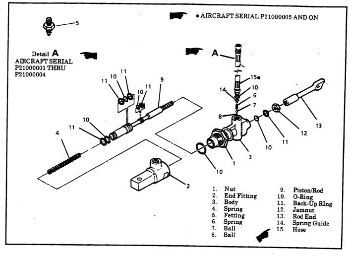
Figure 5-6A. Main Landing Gear Downlock Actuator.
