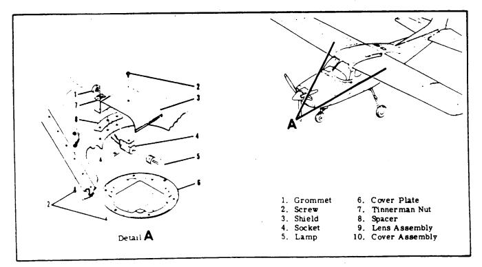
Figure 17-13. Courtesy Light Installation
