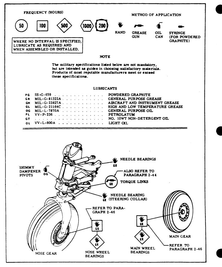
Figure 2-5. Lubrication (Sheet 1 of 4)
