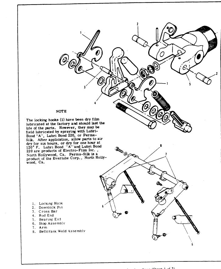
Figure 5A-14. Rigging Nose Landing Gear (Sheet 1 of 2)
