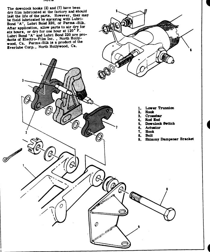
Figure 5-20. Nose Gear Downlock Mechanism
