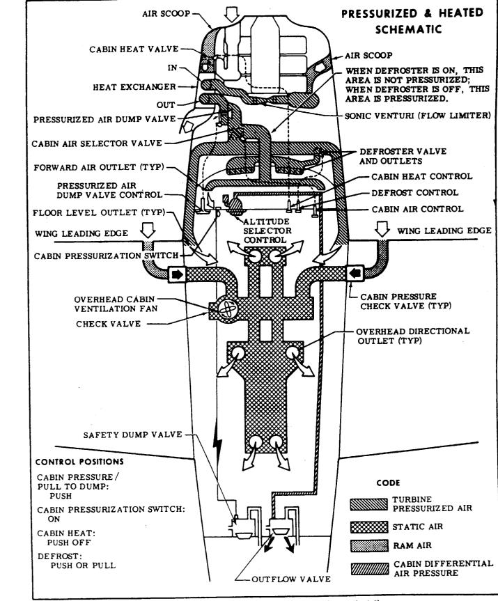
Figure 15-2. Cabin Air Flow Schematic (Sheet 6 of 6)
