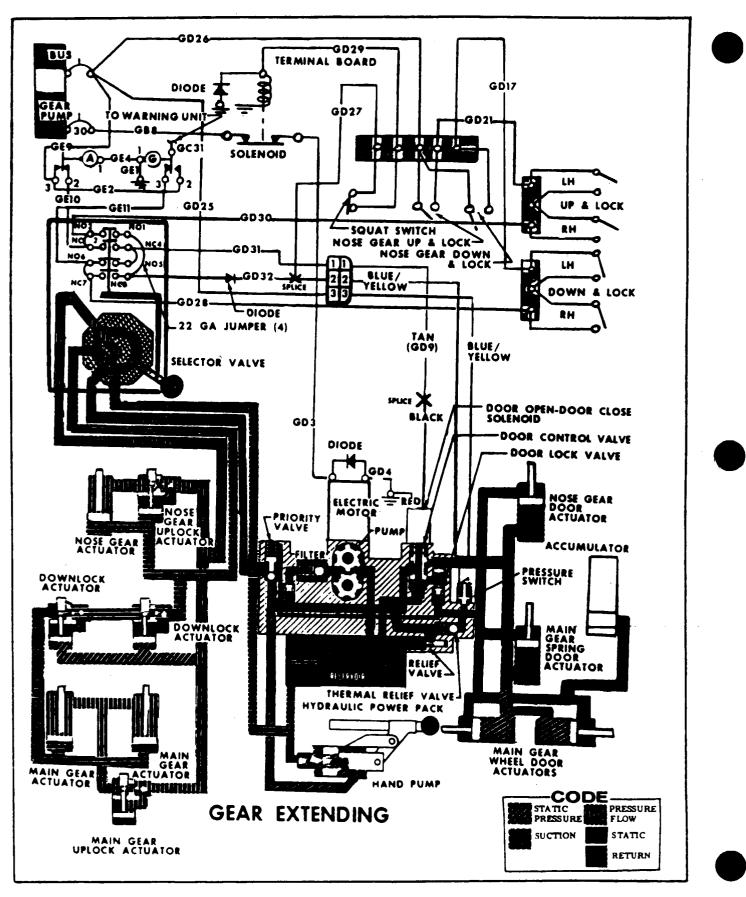
Figure 5-38. Hydraulic and Electrical System Schematic (Sheet 4 of 7)
