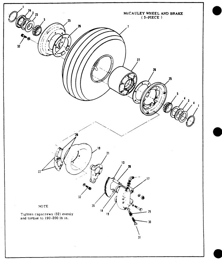
Figure 5-10 Main Landing Gear Wheel, Tire and Brake Assembly (Sheet 3 of 3)
