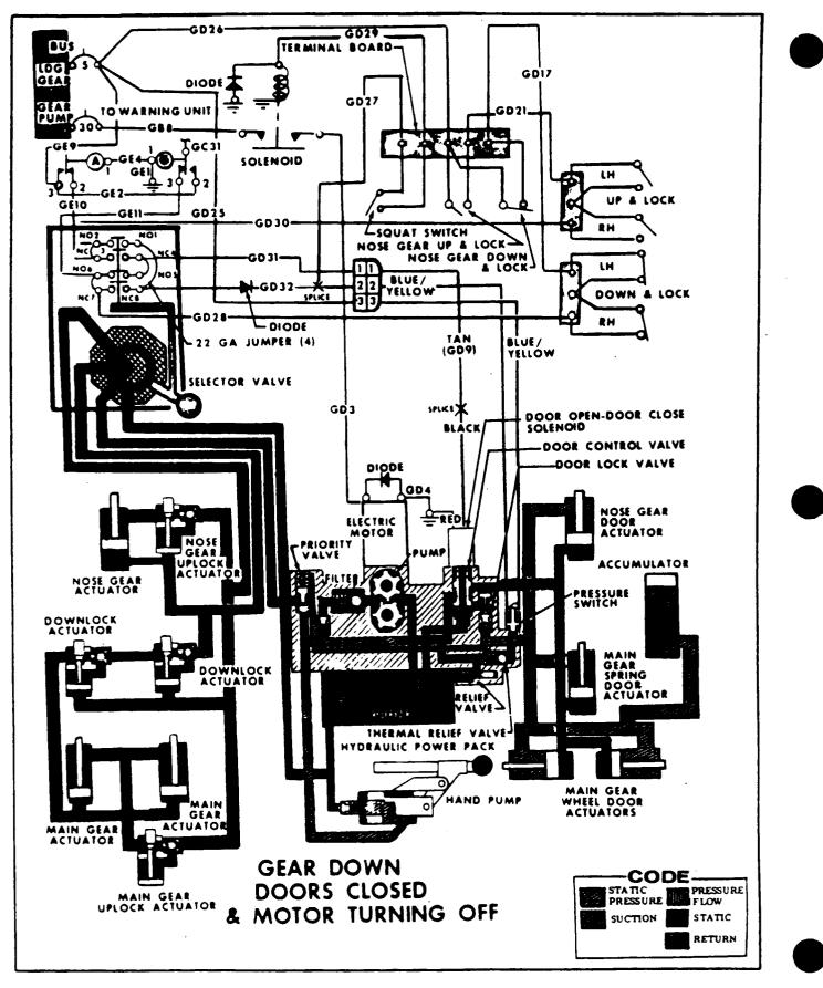
Figure 5-38: Hydraulic and Electrical System Schematic (Sheet 6 of 7)
