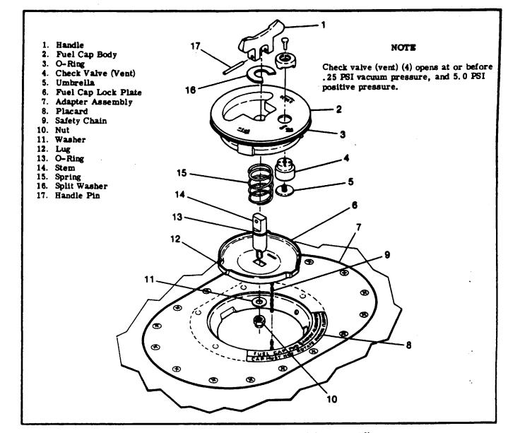
Figure 13-16. Fuel Filler Cap (Metal) (Sheet 1 of 2).
