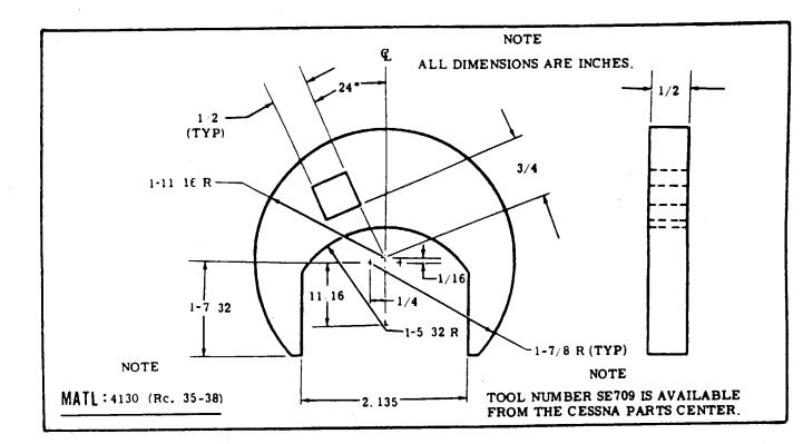
Figure 12-5. Oil Filter Adapter Wrench Fabrication
