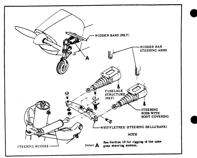
Figure 5-23. Nose Wheel Steering System
