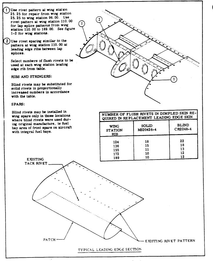
Figure 18-18. Bonded Leading Edge Repair
