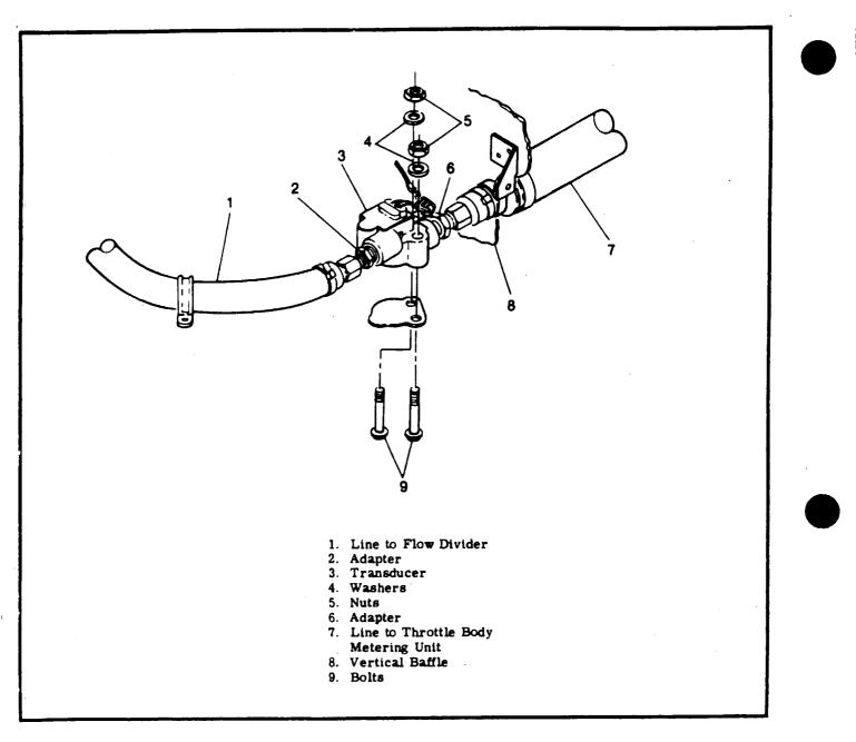
Figure 16-10. Fuel Computer Transducer.
