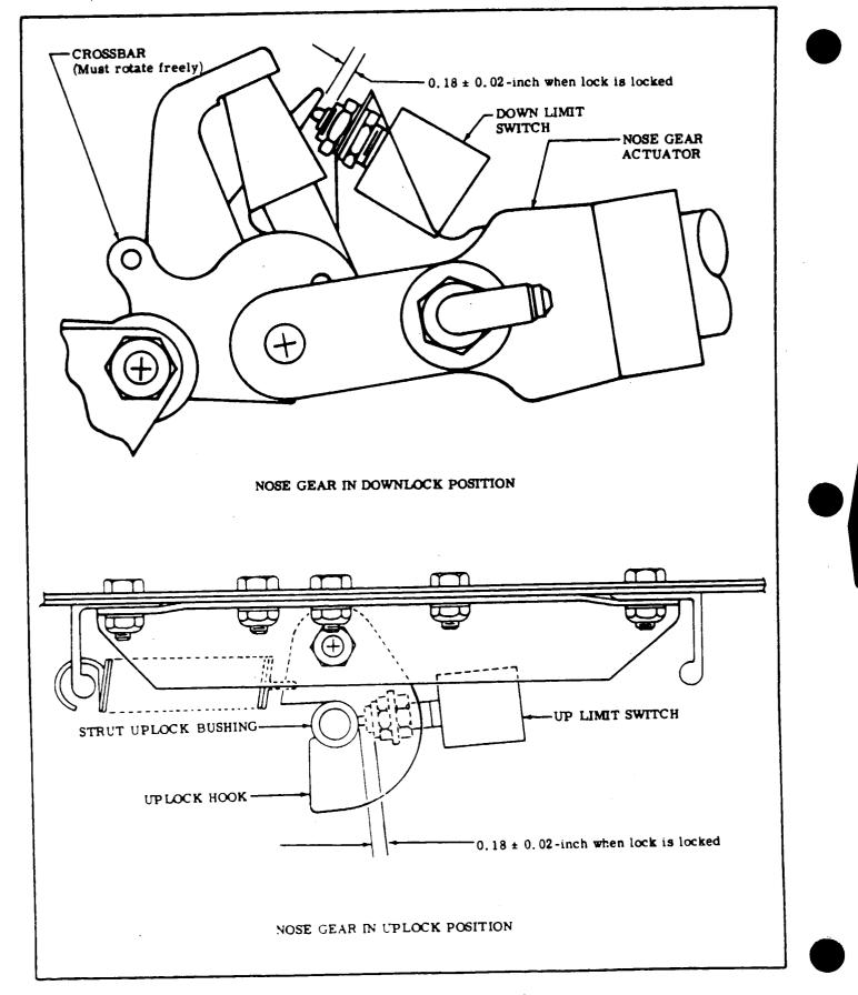
Figure 5-37. Rigging Nose Landing Gear
