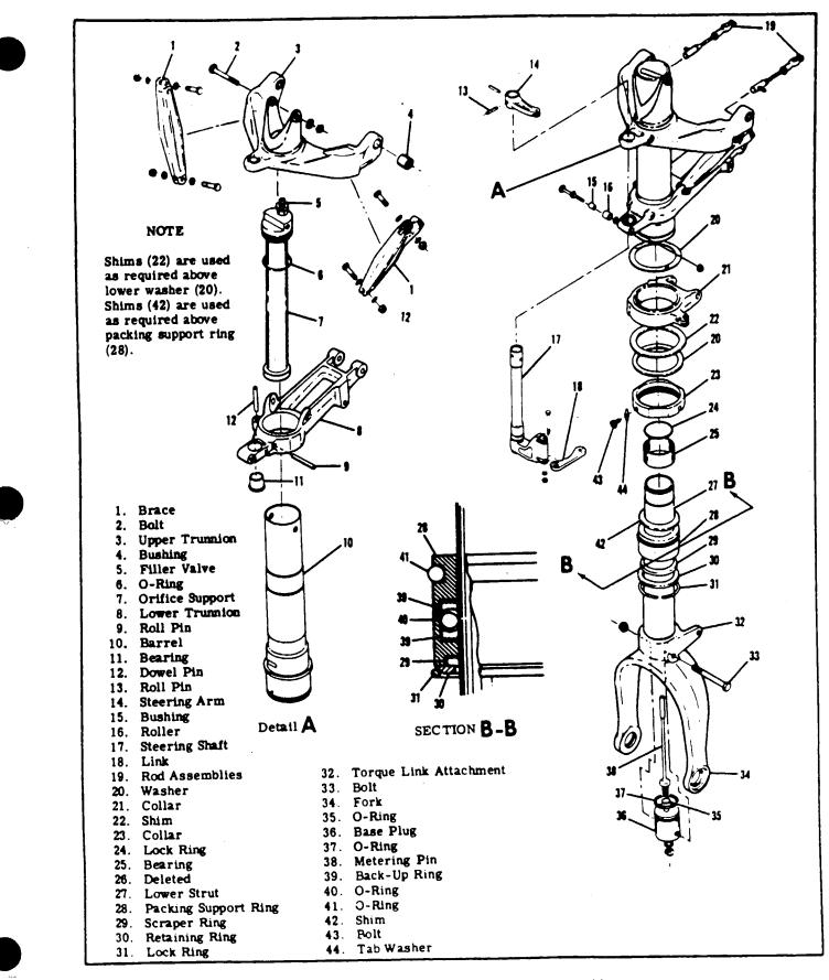
Figure 5-16. Nose Gear Shock Strut Assembly
