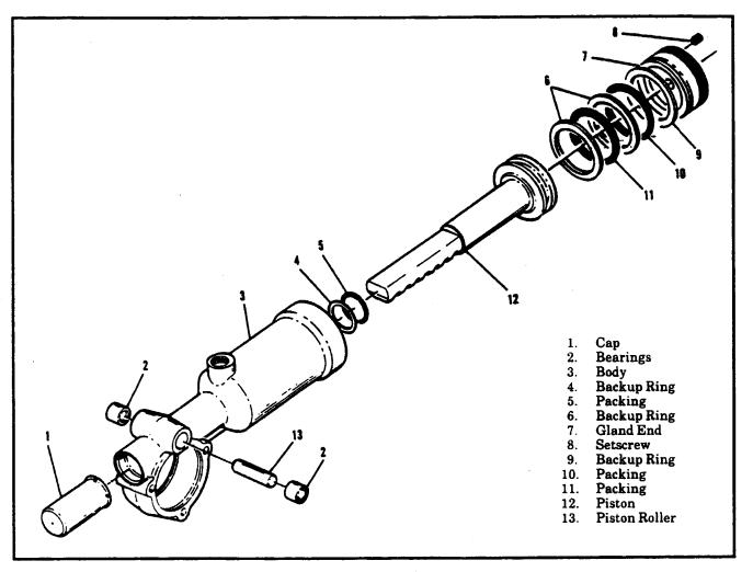
Figure 5A-12 Main Landing Gear Actuator
