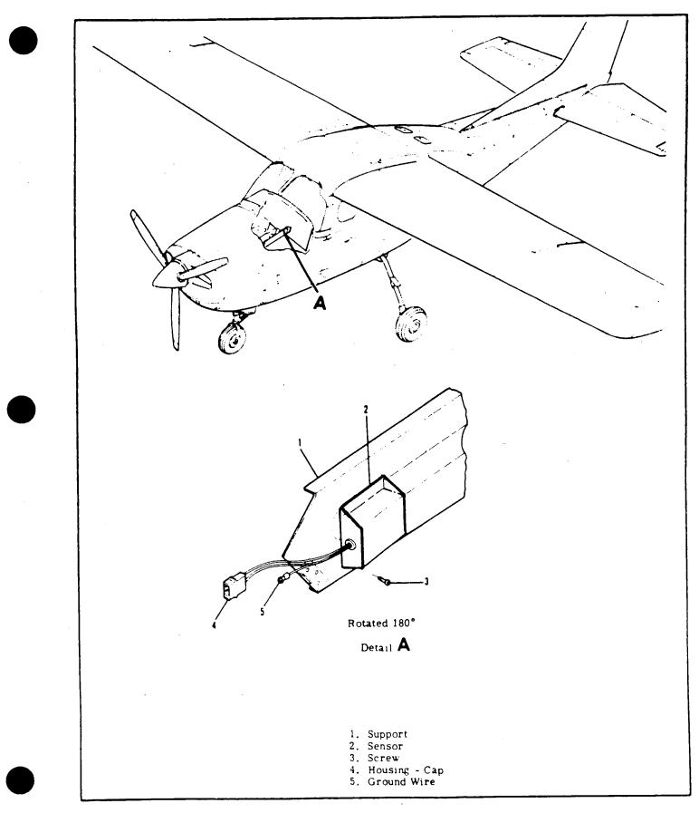
Figure 17-6. Over-Voltage Sensor Installation
