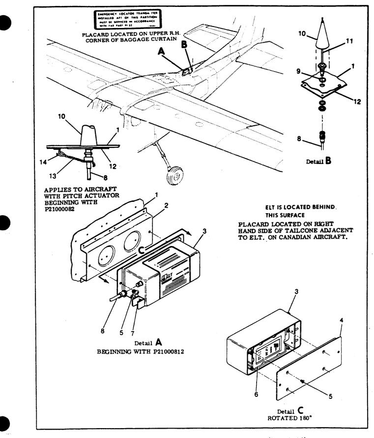
Figure 17-22. Emergency Locator Transmitter Installation (Sheet 3 of 3)
