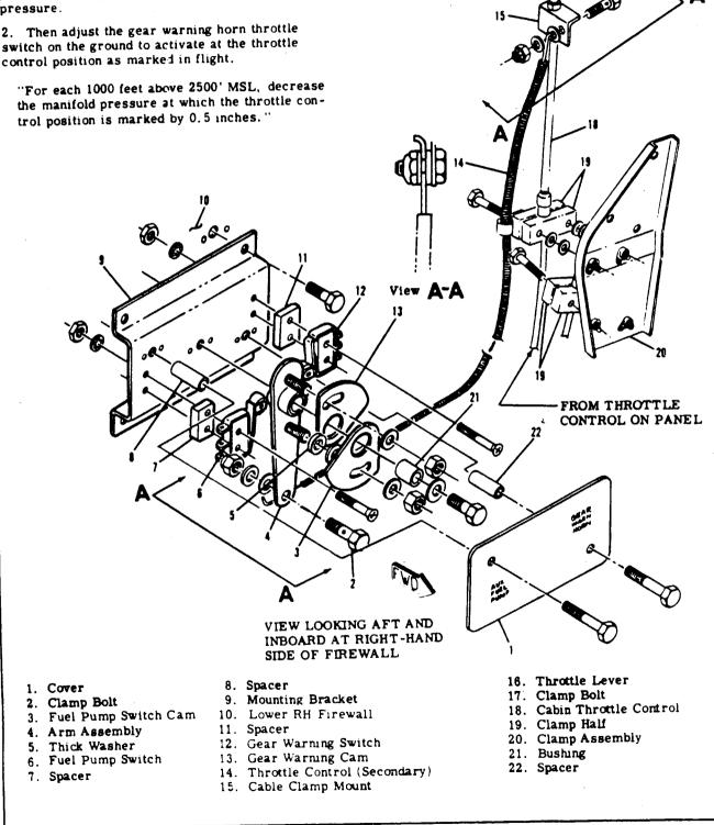
Figure 5A-8. Rigging Throttle-Operated Gear Warning Horn Switch
