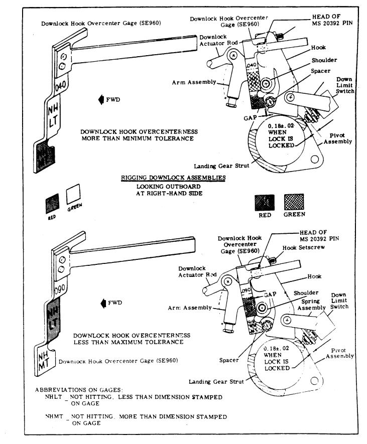
Figure 5A-10. Rigging Miin Landing Gear (Sheet 2 of 3)
