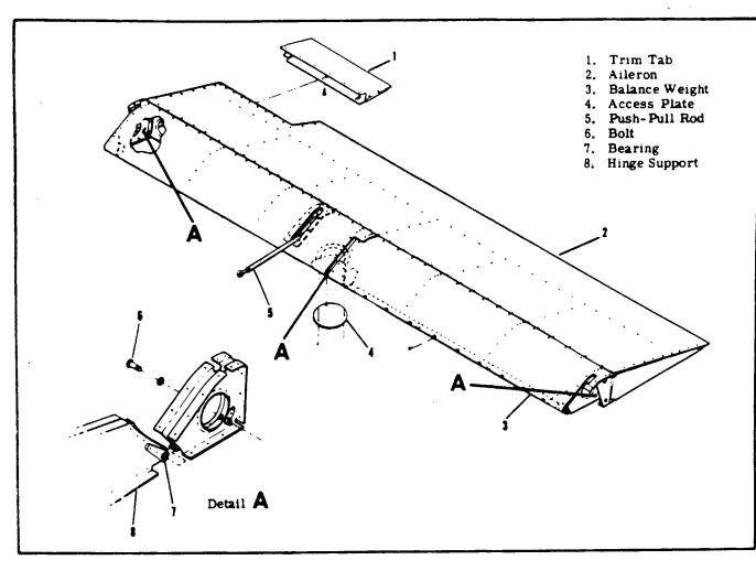
Figure 6-3. Aileron Installation
