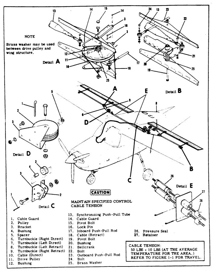
Figure 7-1. Wing Flap Control System (Sheet 1 of 3)
