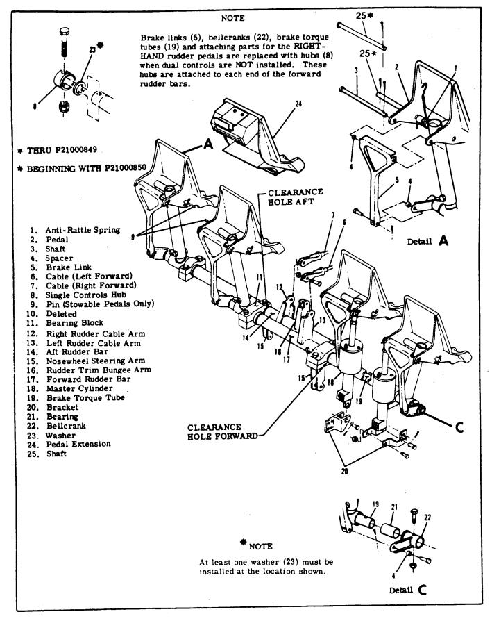
Figure 10-2. Rudder Pedal Installation
