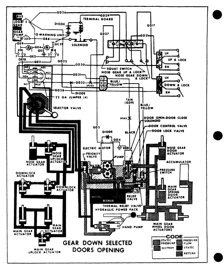
Figure 5-38. Hydraulic and Electrical System Schematic (Sheet 2 of 7)
