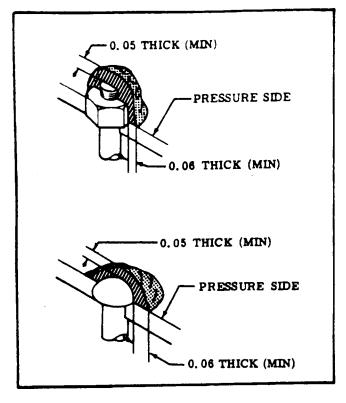
Figure 18-8. Fastener Sealing
