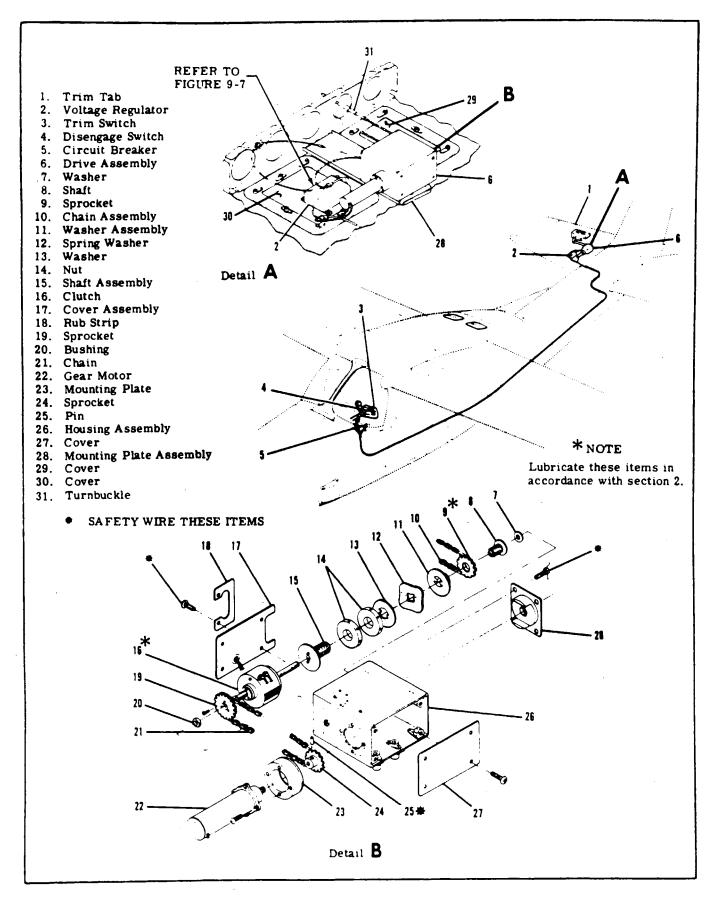
Figure 9-6 Electric Elevator Trim Assist Installation
