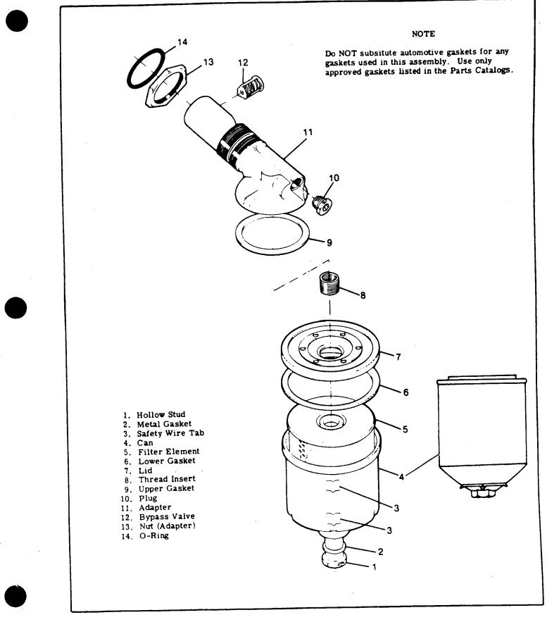
Figure 12-4. Full-Flow Oil Filter
