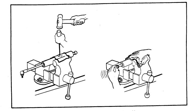
Figure 3-6A. Disposal of Gas Spring Assembly
