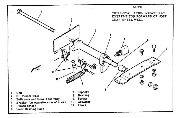
Figure 5-19. Nose Gear Uplock Mechanism
