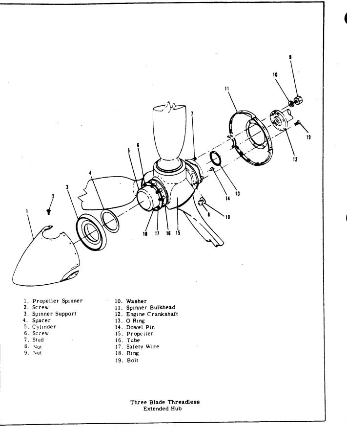
Figure 14-1. Propeller Installation
