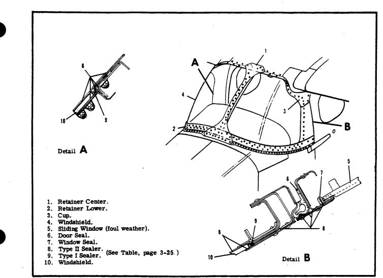
Figure 3-2. Windshield Installation.
