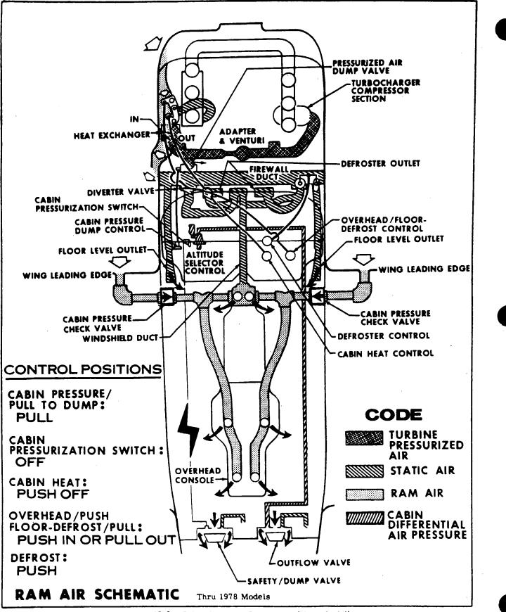
Figure 15-2. Cabin Air Flow Schematic (Sheet 1 of 6)
