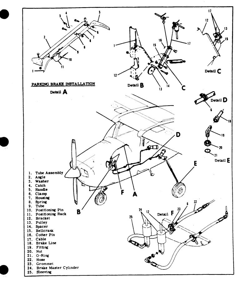
Figure 5-14. Parking Brake System
