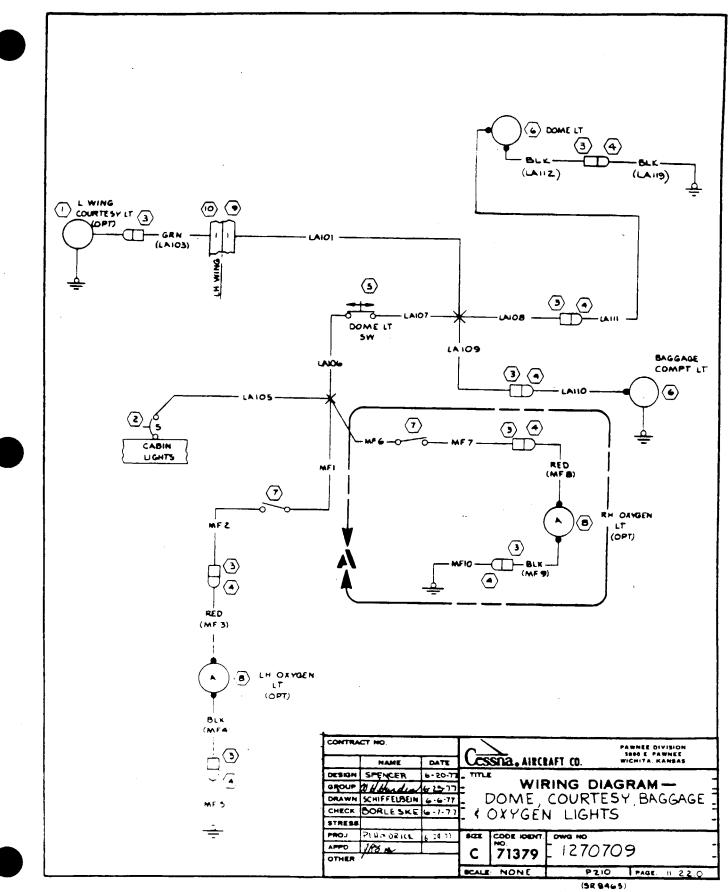
Dome, Courtesy, Baggage & Oxygen Lights (Sheet 2 of 2)
