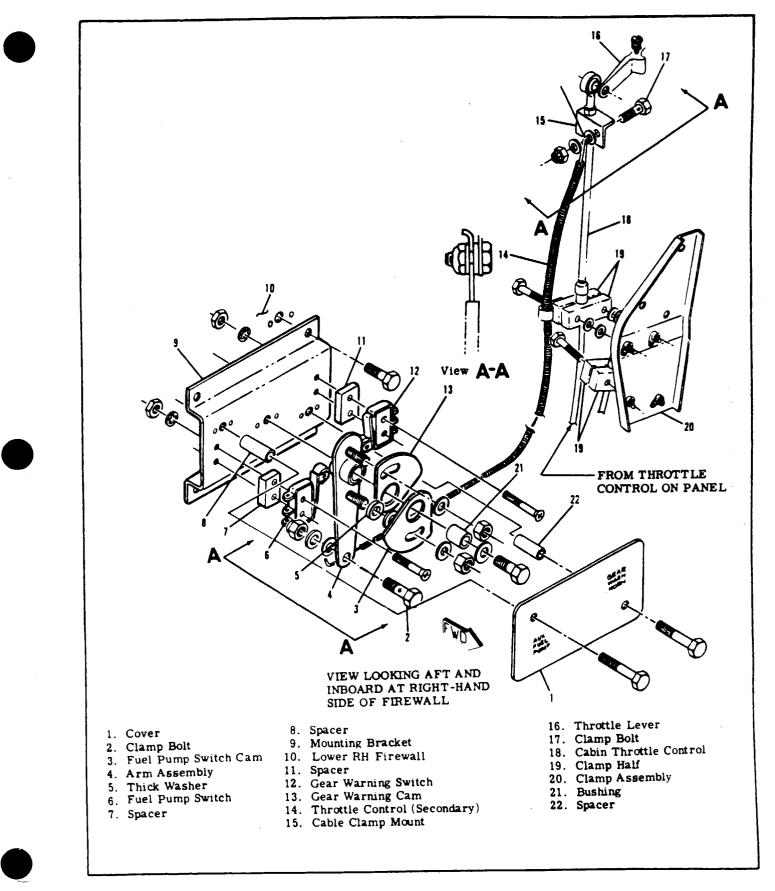
Figure 13-7. Throttle-Operated Microswitches
