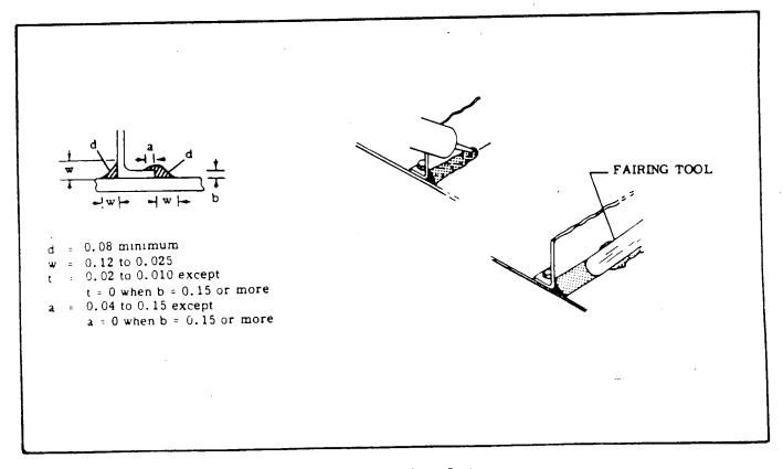
Figure 18-7 Fillet Sealing
