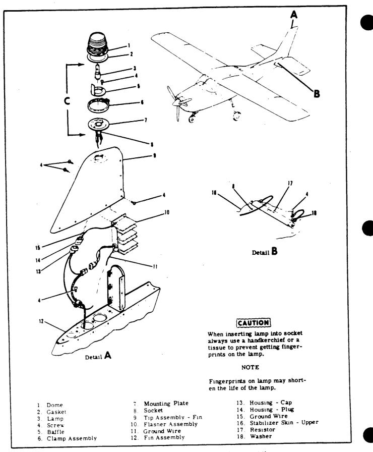
Figure 17-9. Flashing Beacon Installation (Sheet 1 of 2)
