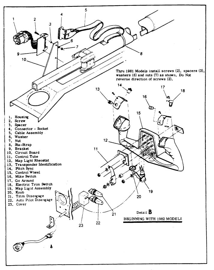
Figure 6-2. Control Column Installation (Sheet 4 of 5)
