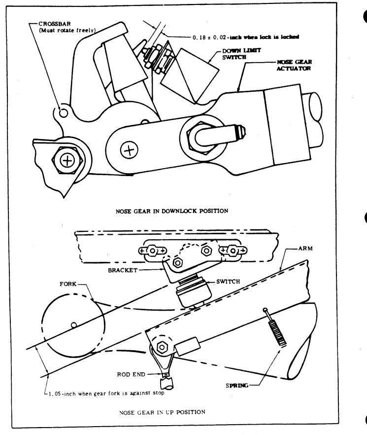
Figure 5A-14. Rigging Nose Landing Gear (Sheet 2 of 2)
