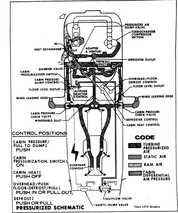
Figure 15-2. Cabin Air Flow Schematic (Sheet 2 of 6)
