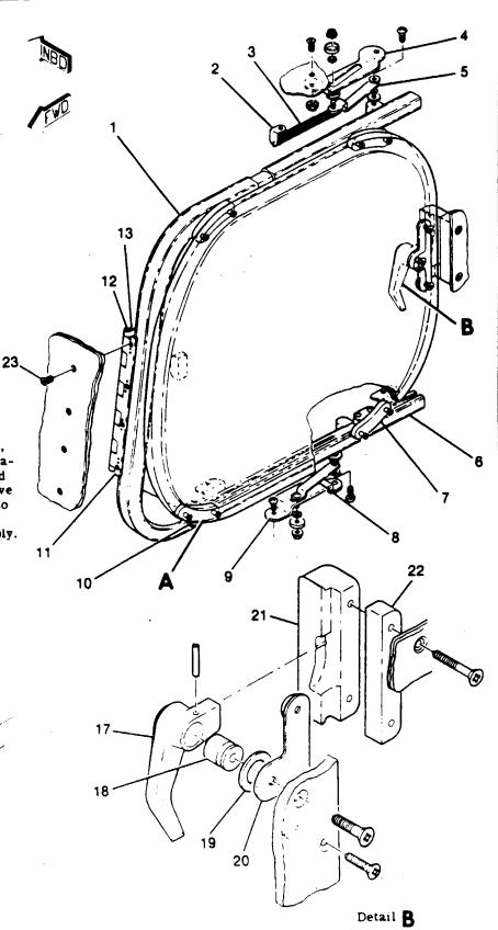
Figure 3-4. Cabin Door Sliding Window Installation
