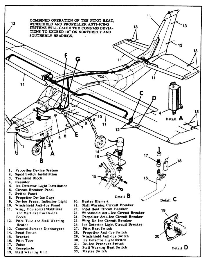
Figure 15-6A. Known Icing Equipment (Sheet 1 of 4)
