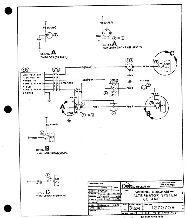
Alternator System, 60 Amp (Sheet 2 of 2)
