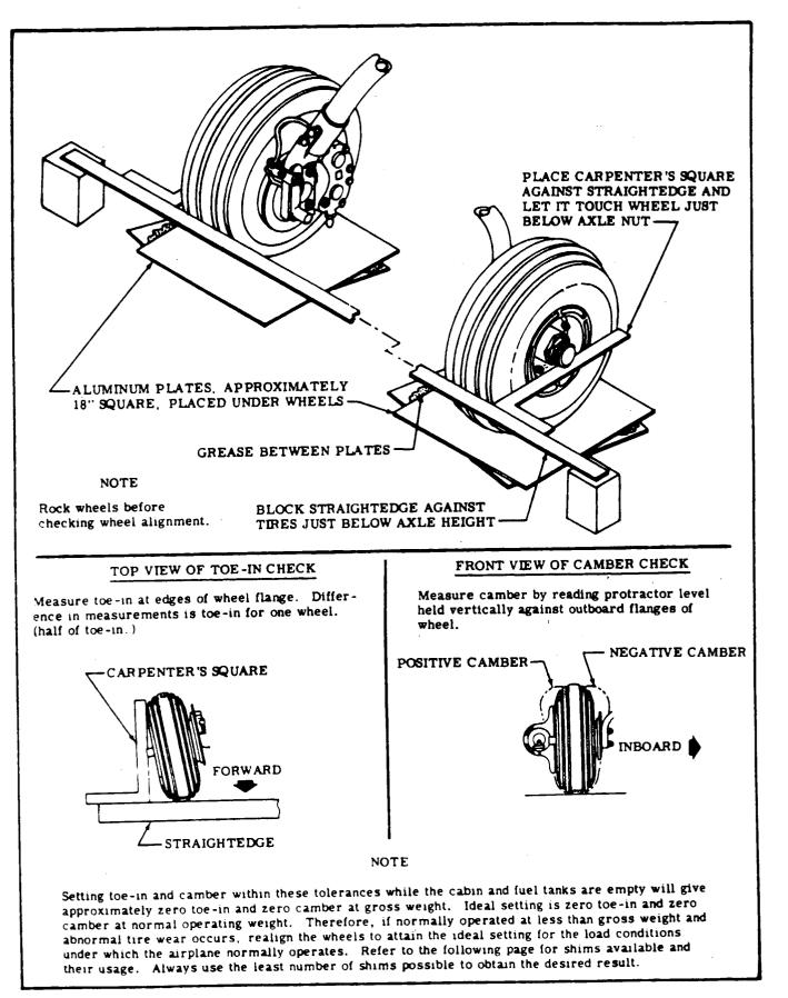
Figure 5-12. Wheel Alignment (Sheet 1 of 2)
