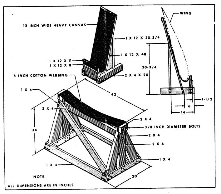
Figure 18-1. Wing and Fuselage Support Stands
