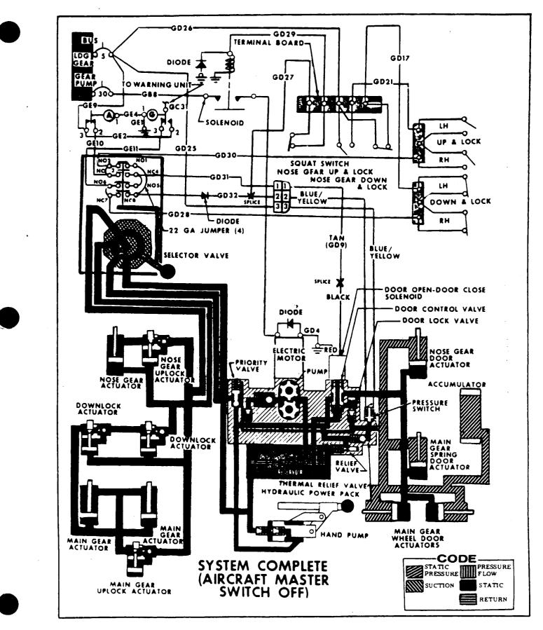
Figure 5-38. Hydraulic and Electrical System Schematic (Sheet 7 of 7)
