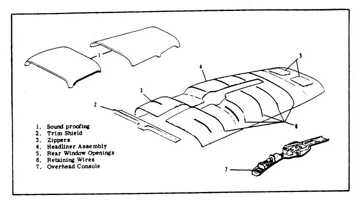
Figure 3-9. Cabin Headliner Installation
