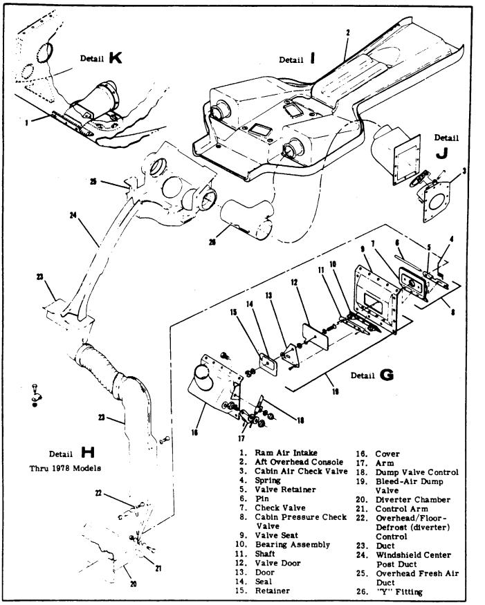
Figure 15-1. Heating, Ventilating and Pressurization System (Sheet 4 of 5)
