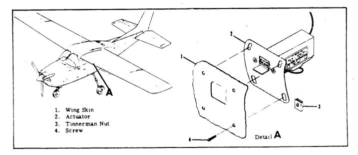
Figure 17-18. Stall Warning Switch.
