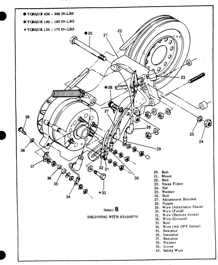
Figure 17-6B. Dual Alternator System Installation (Sheet 4 of 8)
