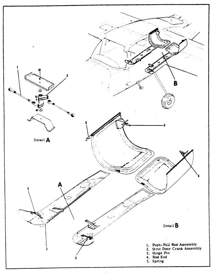
Figure 5-7. Main Landing Gear Doors Installation
