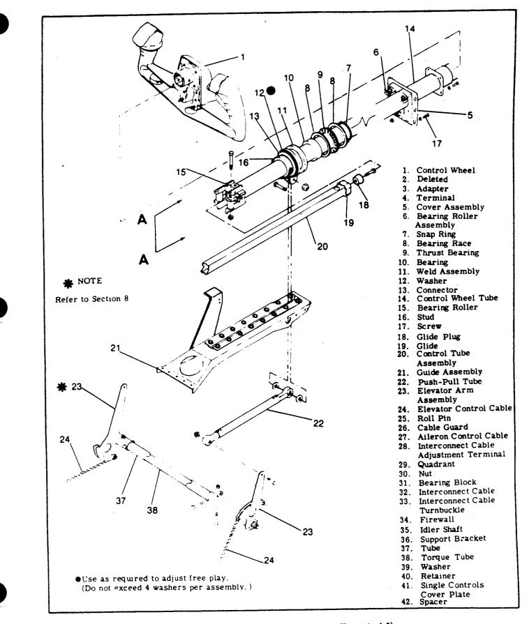
Figure 6-2. Control Column Installation (Sheet 1 of 5)
