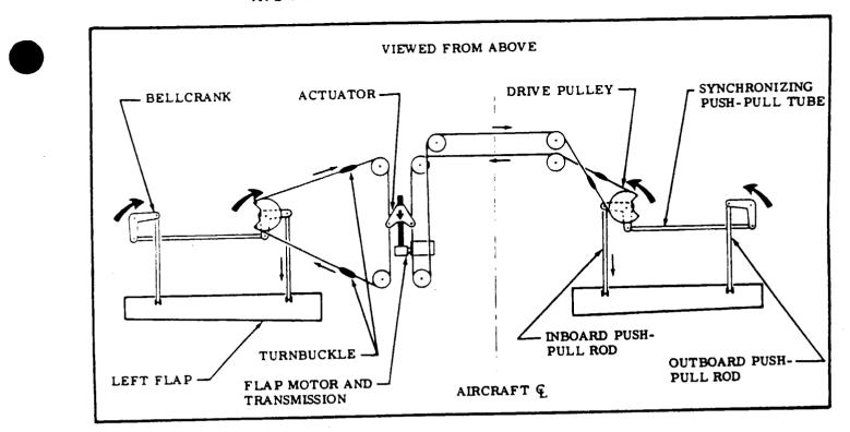
Figure 7-3. Flap System Schematic
