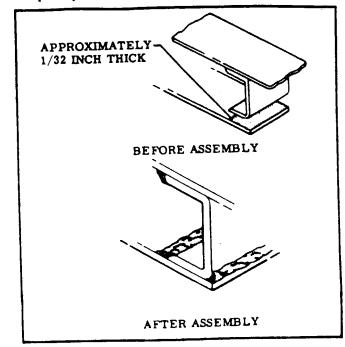
Figure 18-4 Fay Surface Sealing
