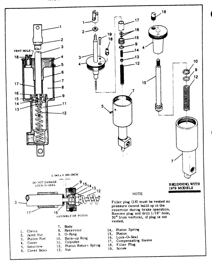
Figure 5-13. Brake Master Cylinder
