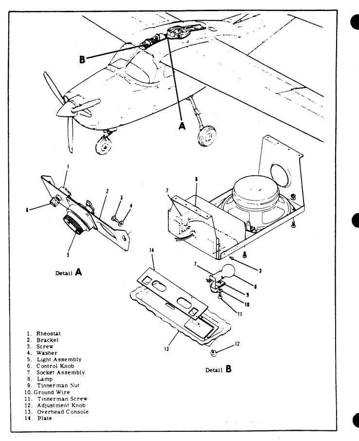
Figure 17-11. Lighting - Overhead Console
