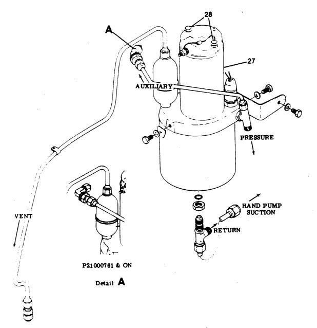
Figure 5A-3. Hydraulic Power Pack Assembly (Sheet 2 of 2)
