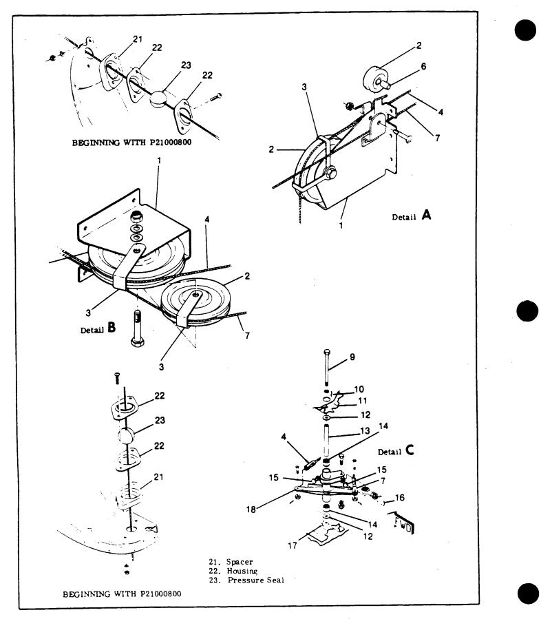
Figure 6-1. Aileron Control System (Sheet 2 of 2)
