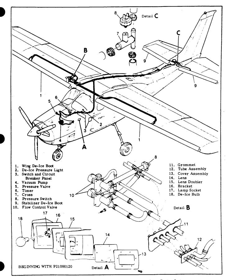
Figure 15-4. Wing and Horizontal Stabilizer Three-Cycle De-ice System
