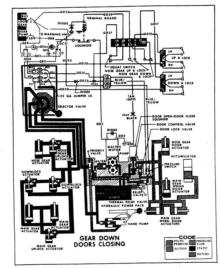
Figure 5-38. Hydraulic and Electrical System Schematic (Sheet 5 of 7)
