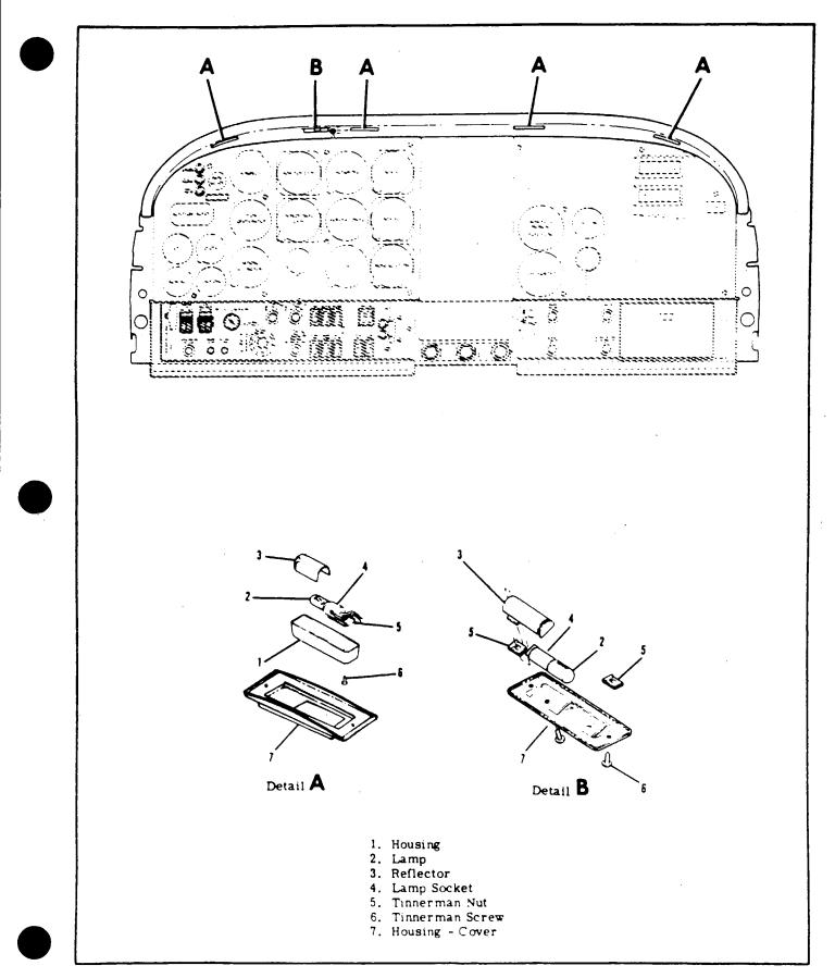
Figure 17-10. Instrument Panel Glare Shield Light Installation
