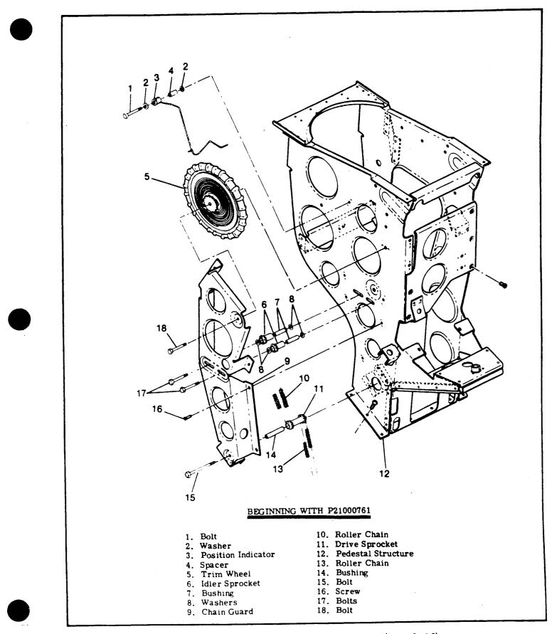
Figure 9-4. Elevator Trim Wheel Installation (Sheet 2 of 2)
