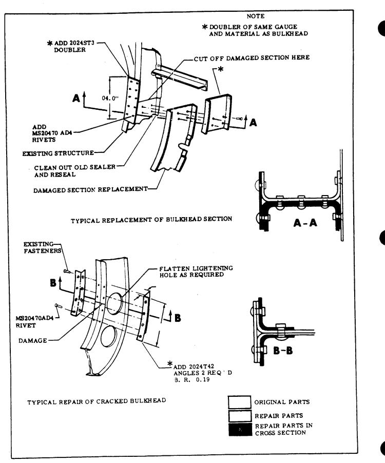
Figure 18-15. Typical Cabin Bulkhead Repair (Sheet 1 of 2)
