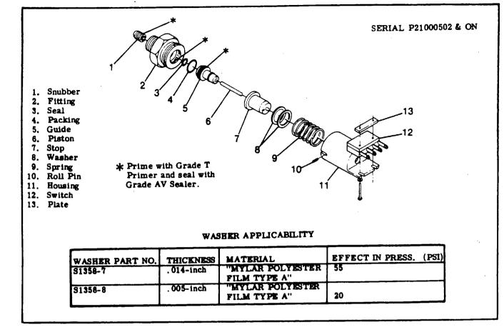
Figure 5A-5A. Pressure Switch
