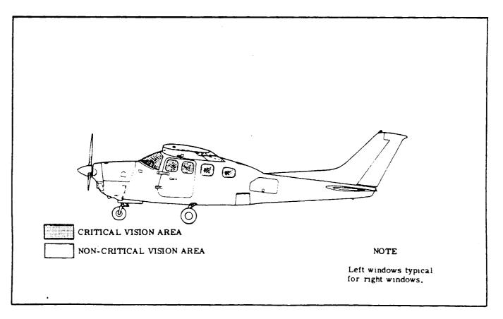
Figure 3-1. Critical Vision Diagram
