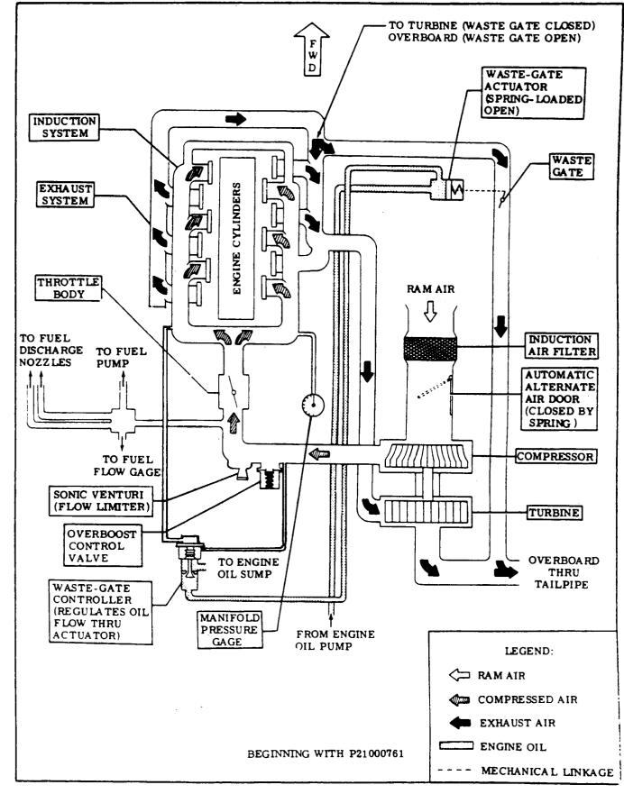
Figure 12-14. Turbocharger System Schematic (Sheet 2 of 2)
