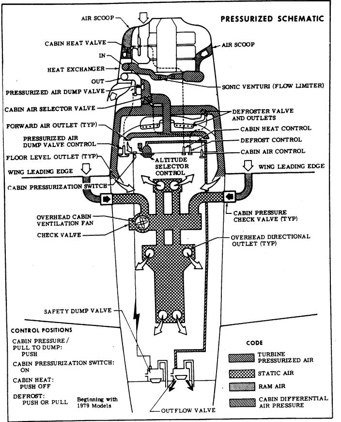
Figure 15-2. Cabin Air Flow Schematic (Sheet 5 of 6)
