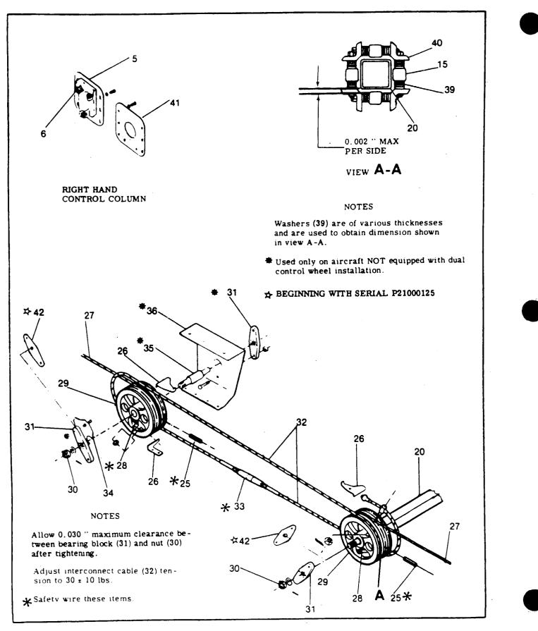
Figure 6-2. Control Column Installation (Sheet 2 of 5)
