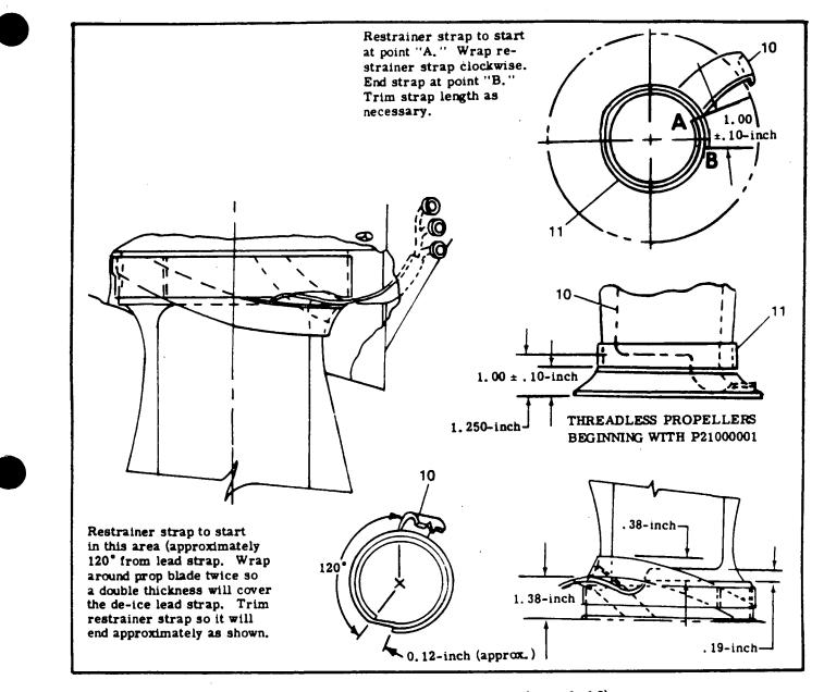
Figure 15-5. Propeller De-Ice System (Sheet 2 of 2)
