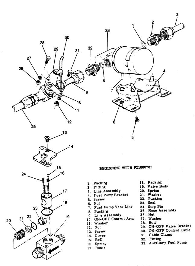
Figure 13-14. Auxiliary Fuel Pump and ON-OFF Valve.
