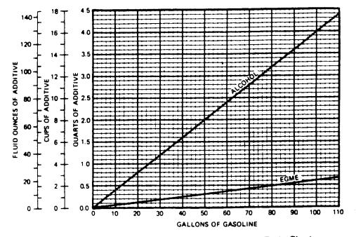
Figure 2-3. Fuel Additive Mixing Ratio Chart
