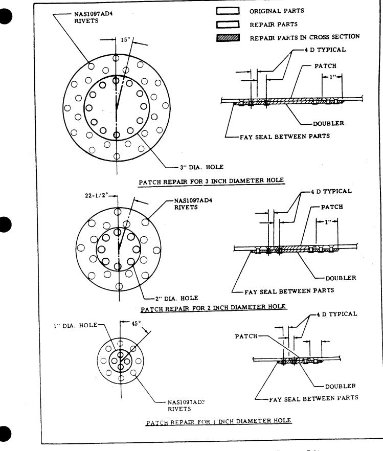
Figure 18-17. Typical Circular Hole Skin Repair in Pressure Cabin
