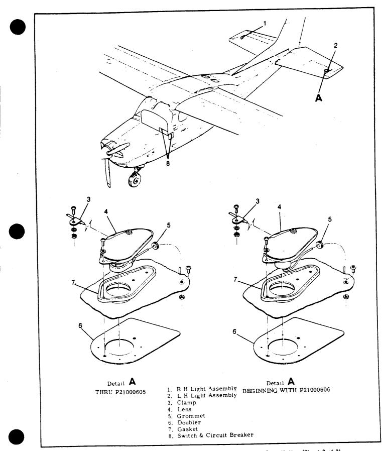
Figure 17-8. Navigation, Flood and Anti-Collision Strobe Lights Installation (Sheet 2 of 2)
