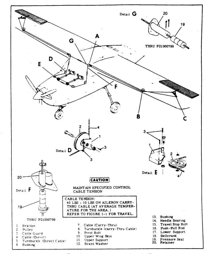
Figure 6-1. Aileron Control System (Sheet 1 of 2)
