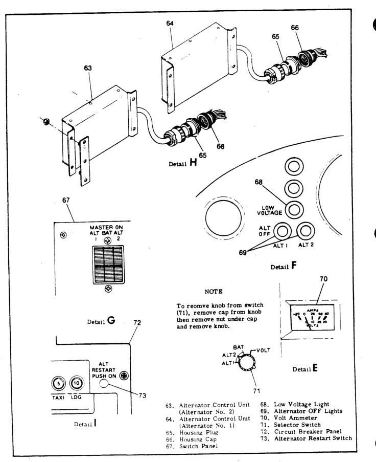
Figure 17-6B. Dual Alternator System Installation (Sheet 7 of 8)
