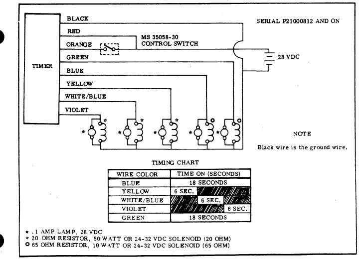
Figure 15-4E. Wing, Horizontal Stabilizer and Vertical Fin De-Ice System Timer.
