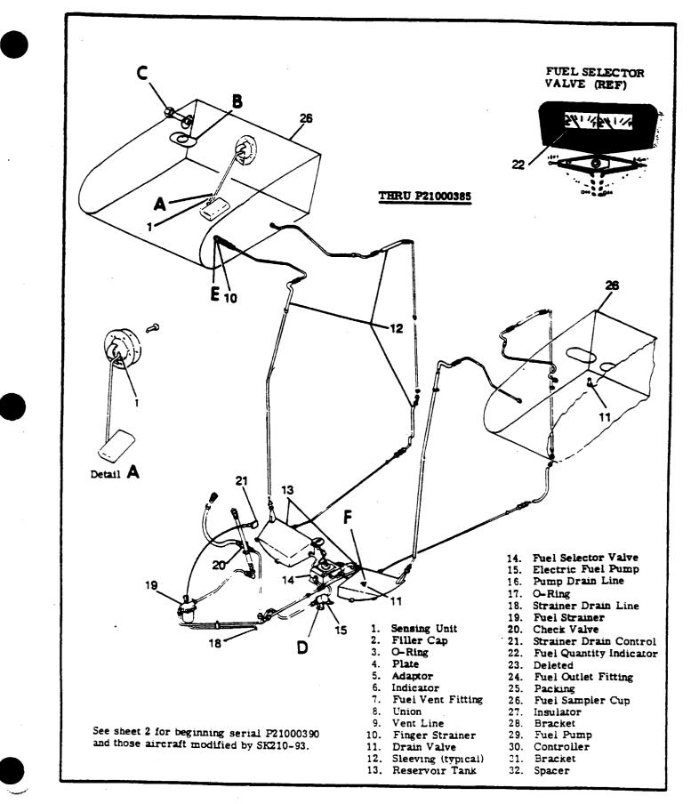
Figure 13-2. Fuel System (Sheet 1 of 4)
