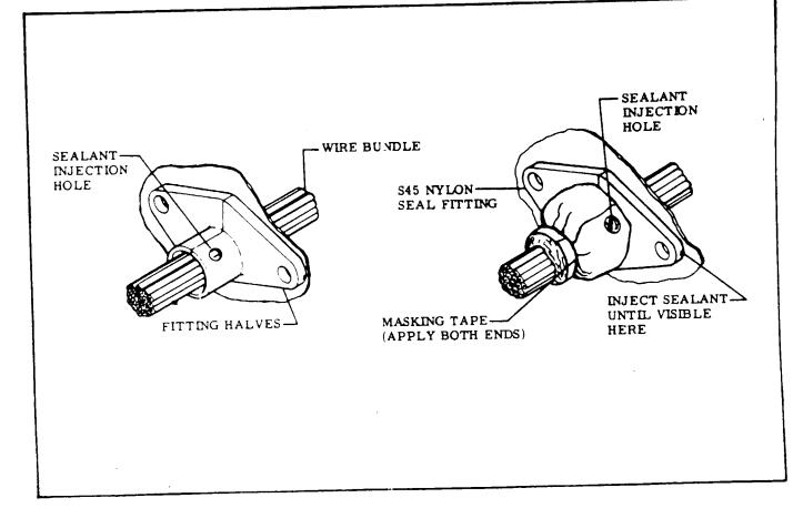
Figure 18-10. Electrical Sealing
