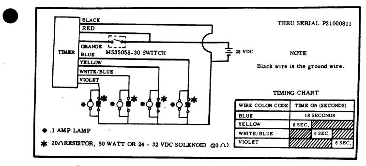
Figure 15-4D. Wing, Horizontal Stabilizer and Vertical Fin De-Ice System Timer.
