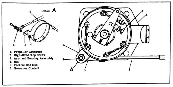
Figure 14-3. Governor and Control Adjustments
