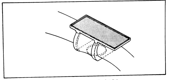
Figure 5-33. Landing Gear Strut Step Installation
