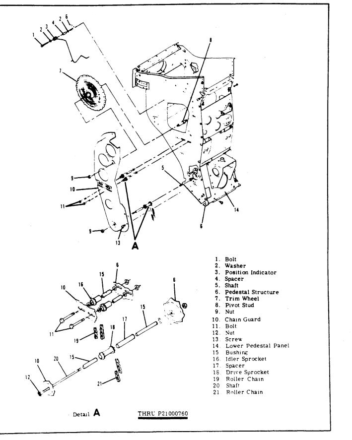
Figure 9-4. Elevator Trim Wheel Installation (Sheet 1 of 2)
