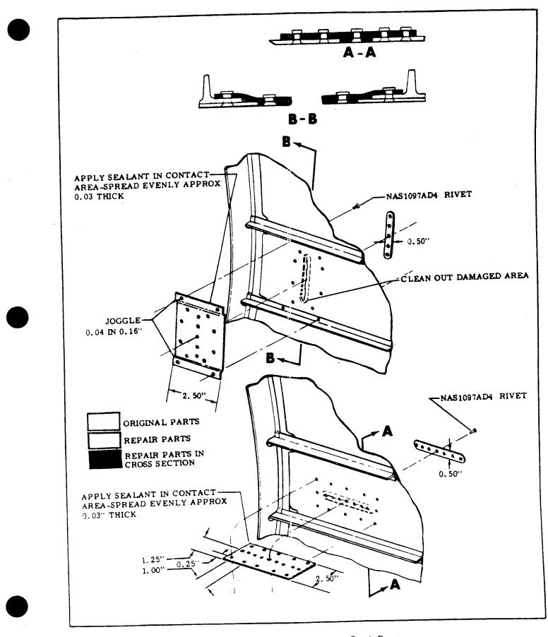
Figure 18-14. Typical Cabin Skin Crack Repair
