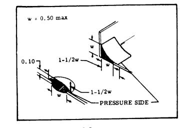
Figure 18-5. Hole Filling
