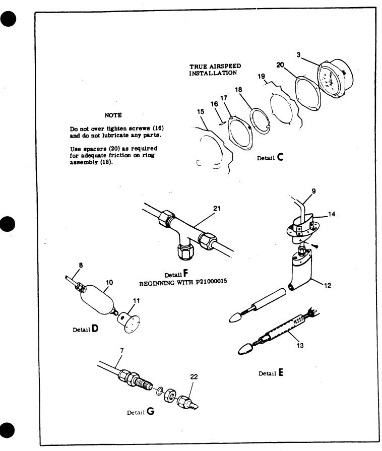
Figure 16-2. Pitot Static System (Sheet 2 of 2)
