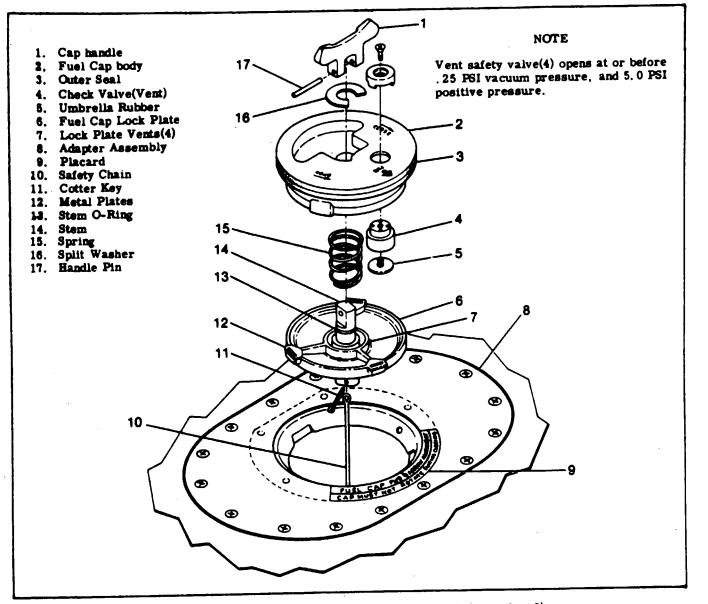
Figure 13-16. Fuel Filler Cap (Red Plastic) (Sheet 2 of 2)
