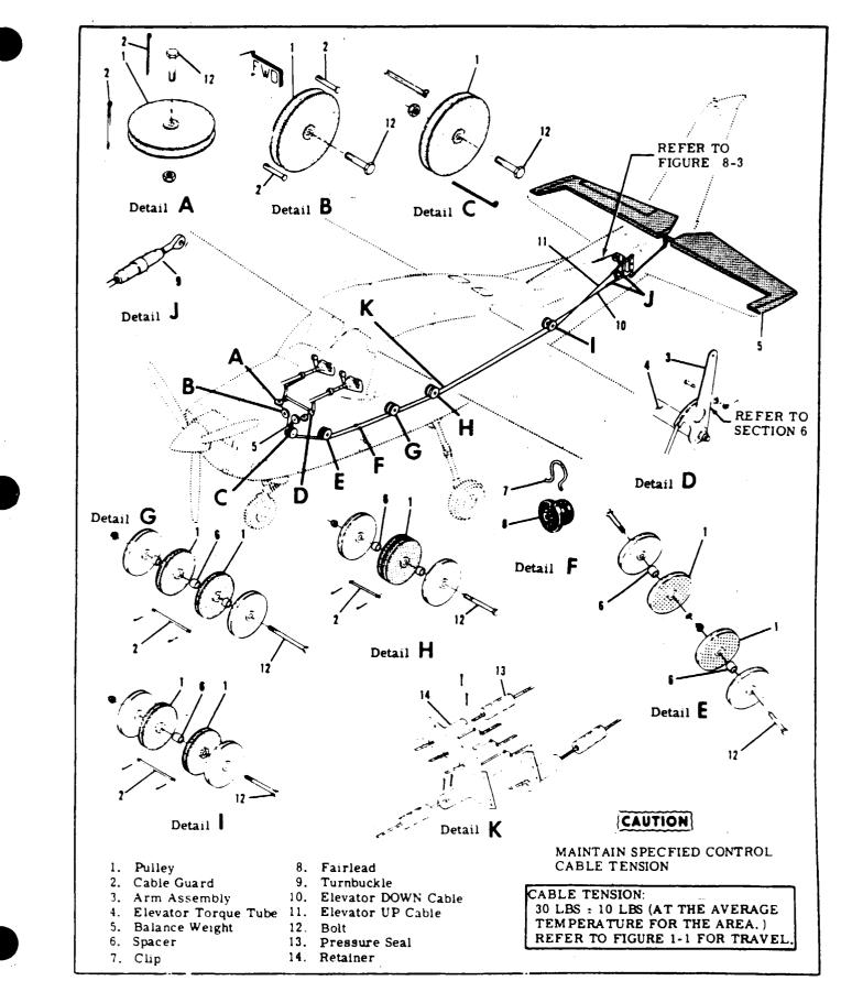
Figure 8-1. Elevator Control System
