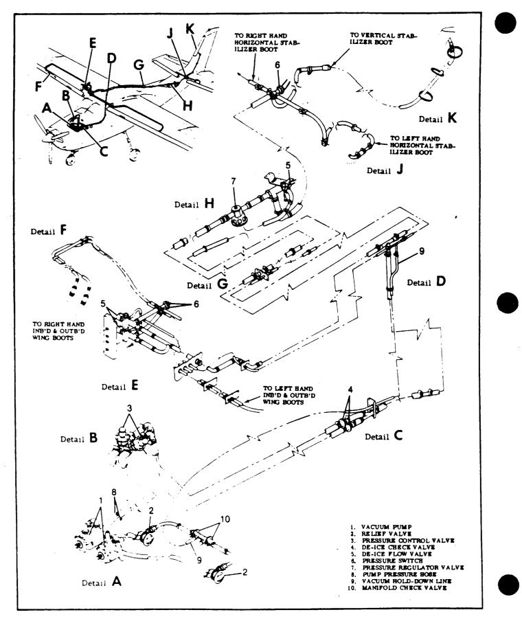
Figure 15-4C. Surface De-Ice System Components.
