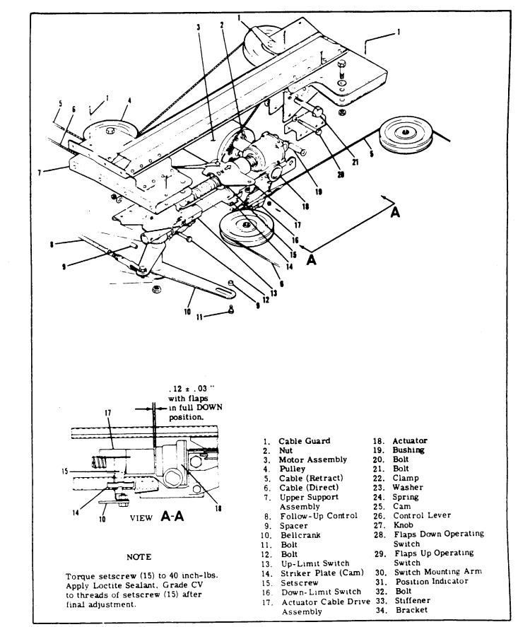
Figure 7-1. Wing Flap Control System (Sheet 2 of 3).
