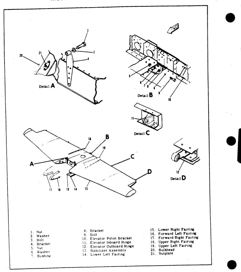
Figure 4-3. Horizontal Stabilizer Installation
