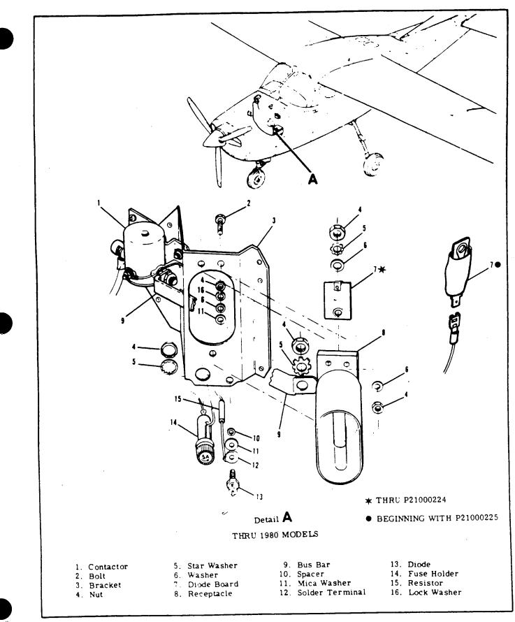
Figure 17-3. Ground Service Receptacle Installation (Sheet 1 of 2)
