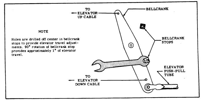
Figure 8-4. Elevator Bellcrank Travel Stop Adjustment
