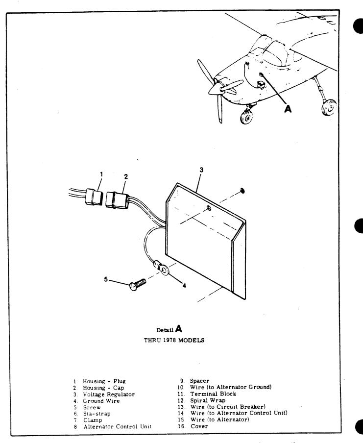
Figure 17-5. Voltage Regulator/Alternator Control Unit Installation (Sheet 1 of 3)
