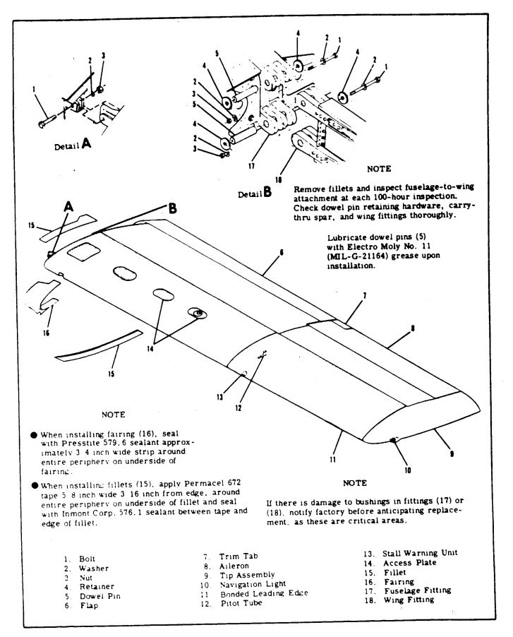
Figure 4-1. Wing Installation
