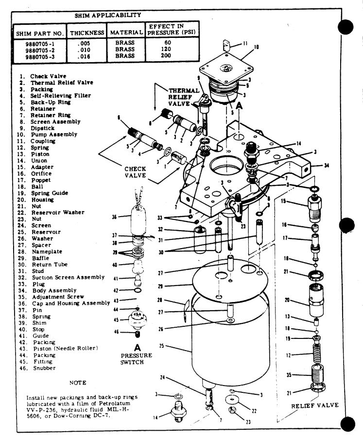
Figure 5-27. Power Pack Disassembly and Reassembly
