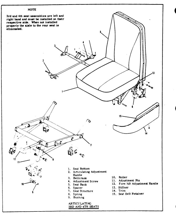
Figure 3-8. Seat Installation (Sheet 2 of 3)
