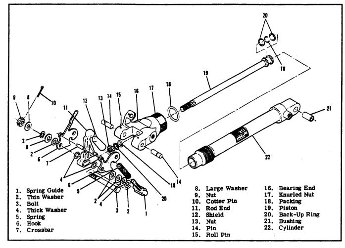
Figure 5-21. Nose Gear Actuator
