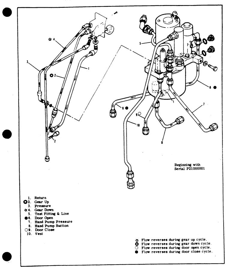
Figure 5-35. Hydraulic Power Pack Line Routing
