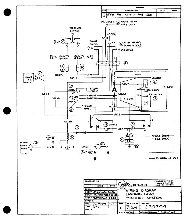
Landing Gear Control System (Sheet 1 of 2)
