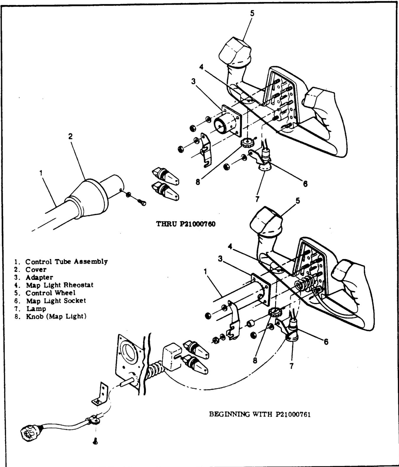
Figure 17-14. Control Wheel Map Light Installation
