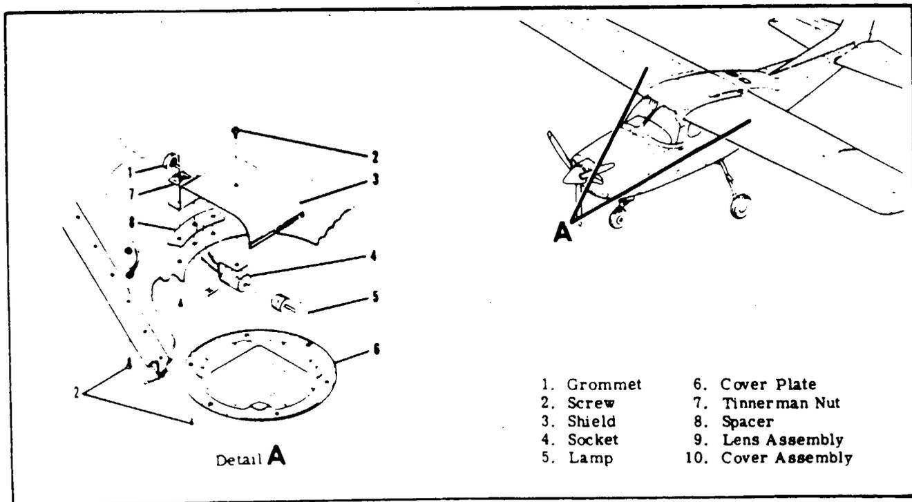
Figure 17-13. Courtesy Light Installation
