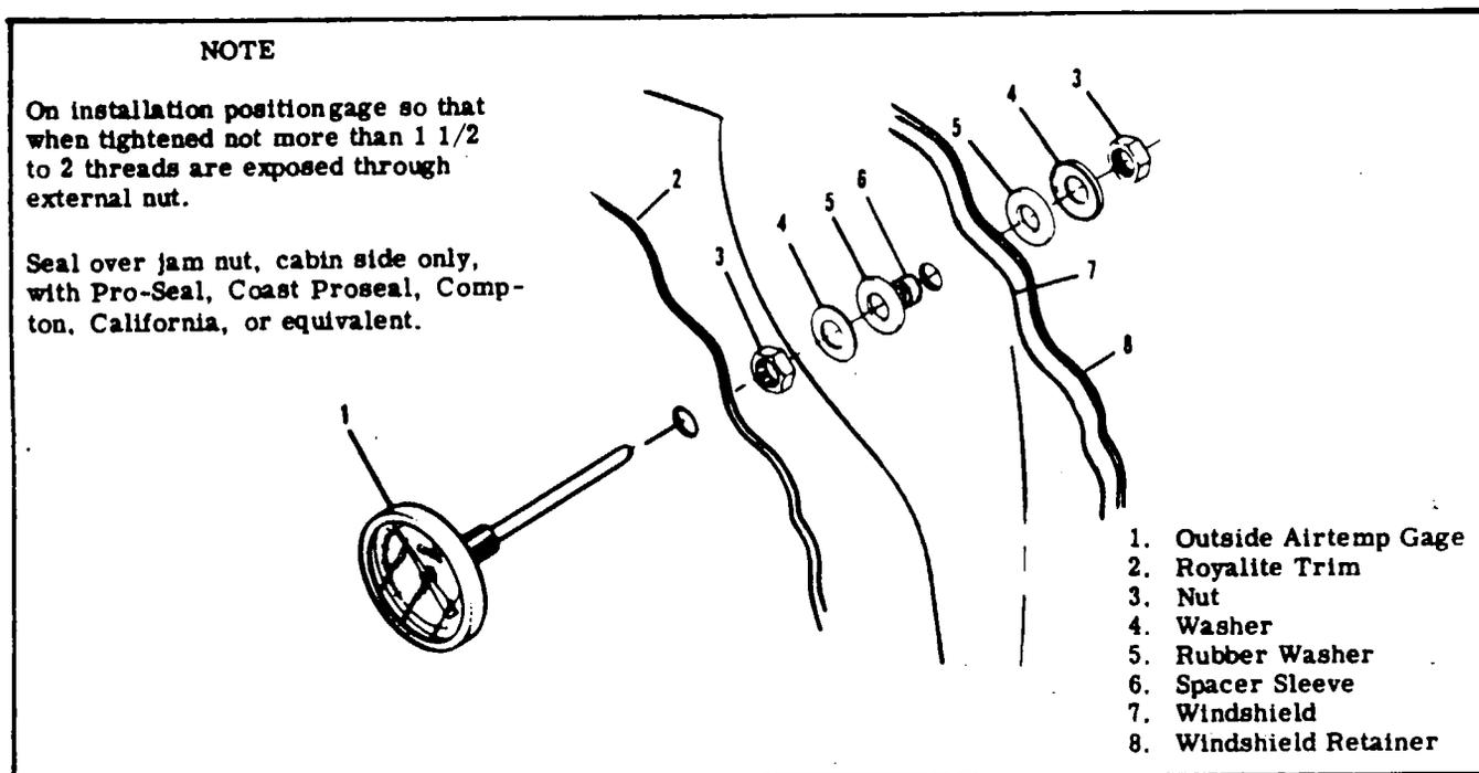
Figure 16-8. Outside Air Temperature Gage
