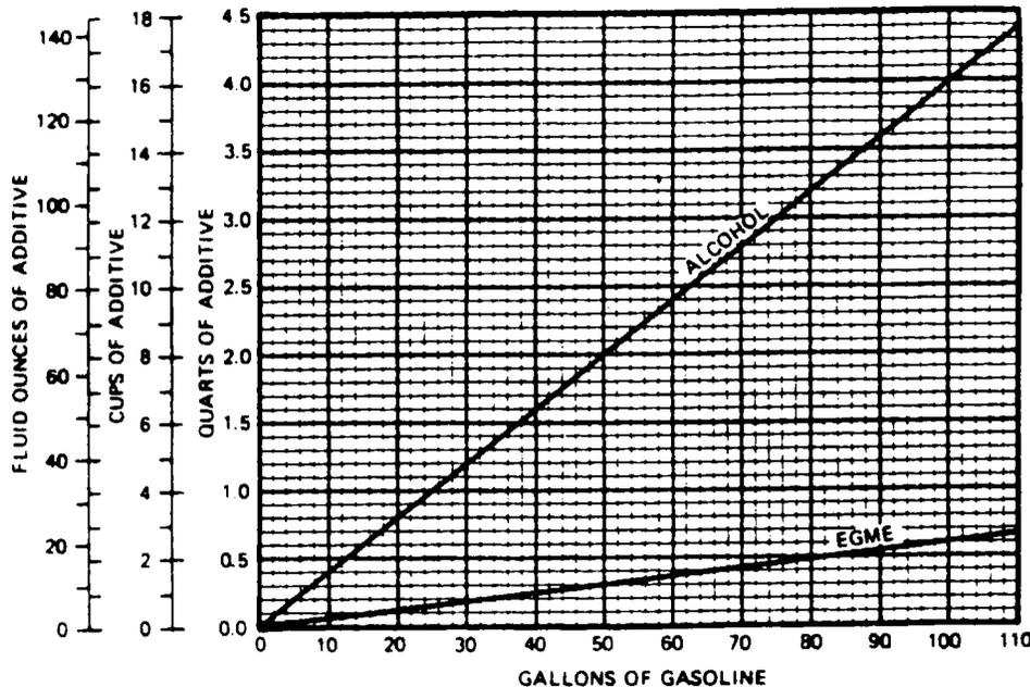
Figure 2-3. Fuel Additive Mixing Ratio Chart
