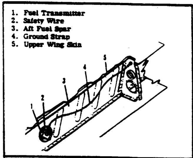
Figure 16-6. Fuel Transmitter Installation
