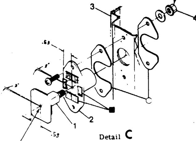
Grease cored area of receptacle before checking latch fit.
