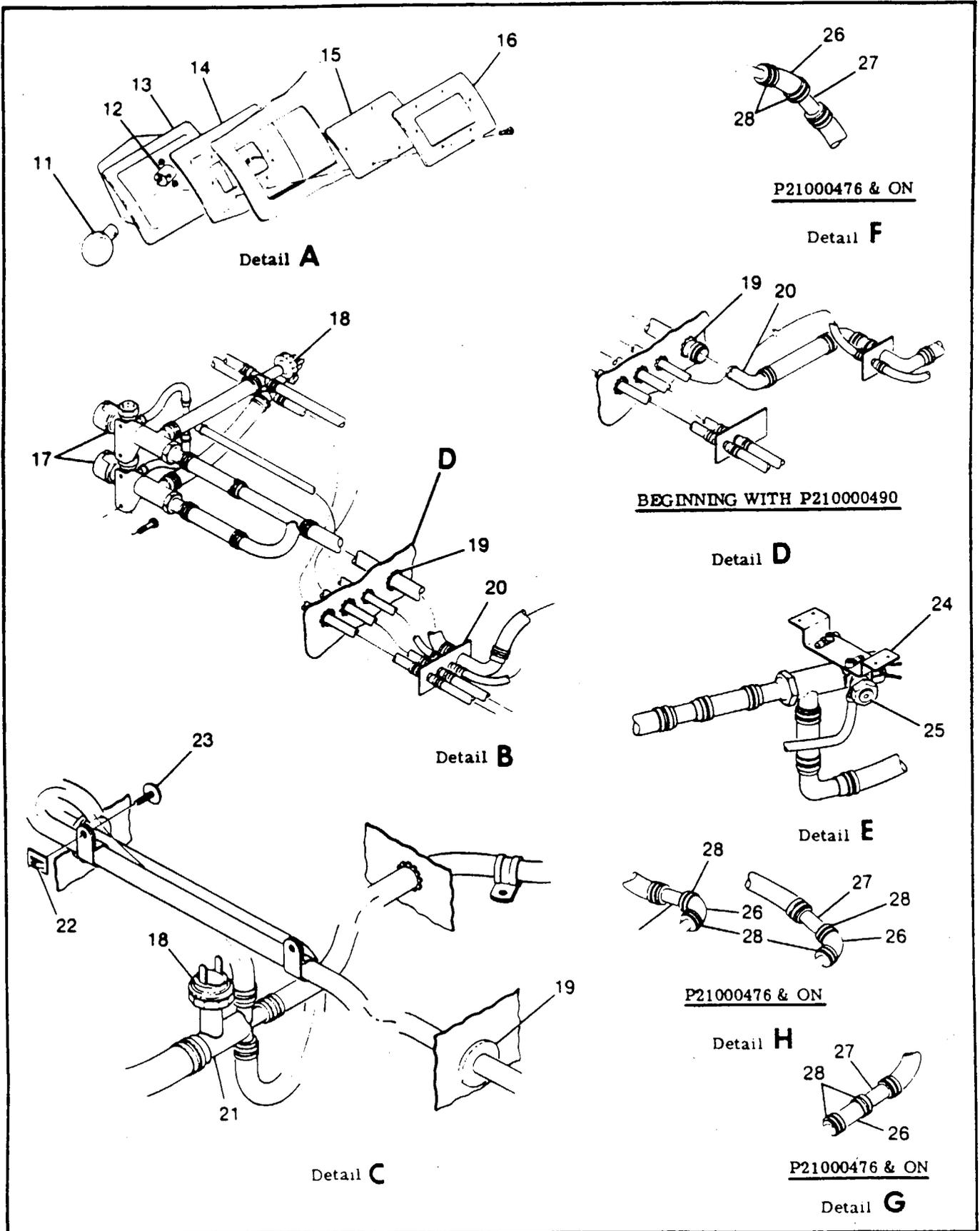
Figure 15-4A. Wing, Horizontal Stabilizer and Vertical Fin De-Icing System (Sheet 2 of 5)
