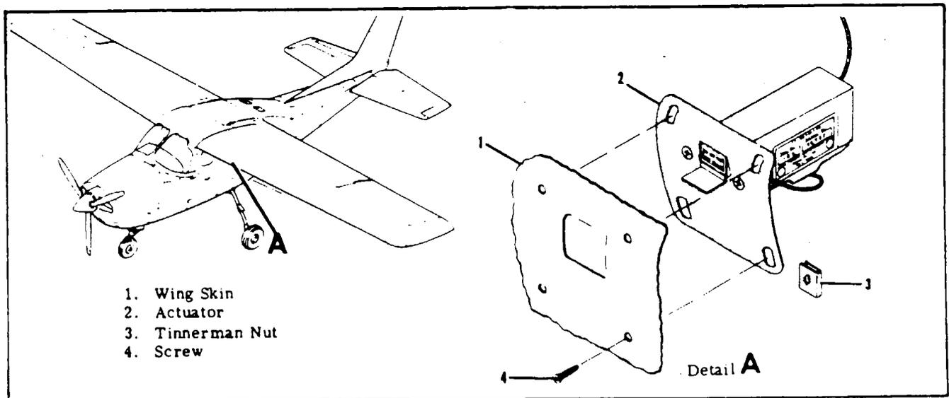
Figure 17-18. Stall Warning Switch.
