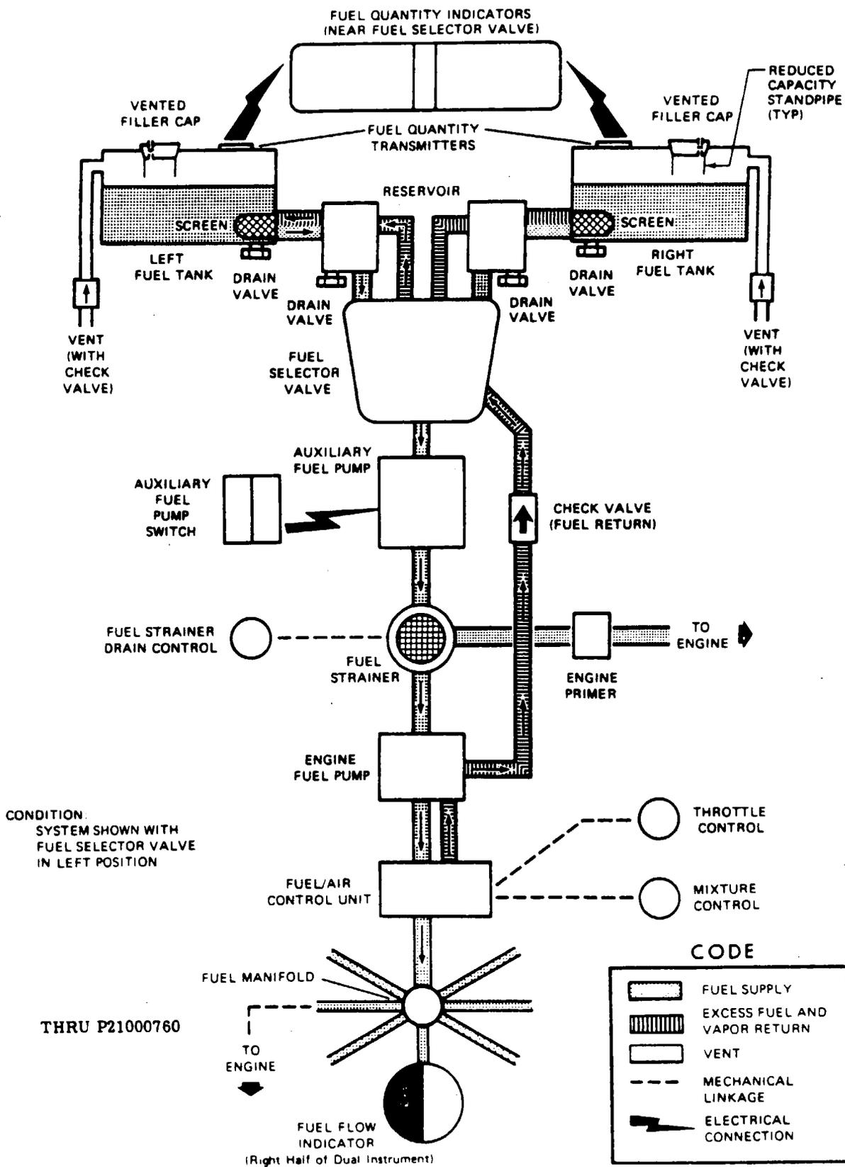
Figure 13-1. Fuel System Schematic
