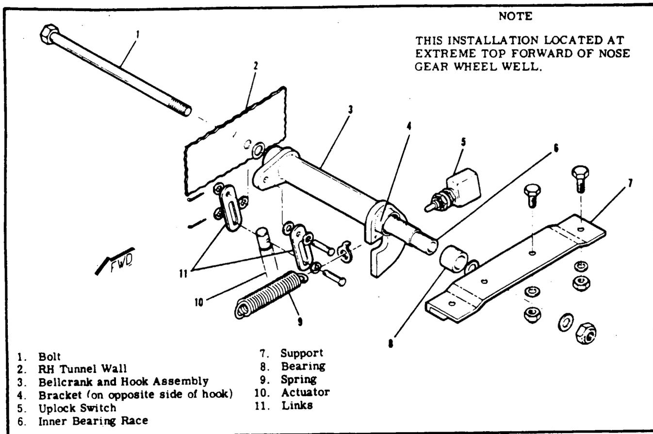
Figure 5-19. Nose Gear Uplock Mechanism
