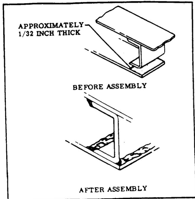
Figure 18-4 Faying Surface Sealing
