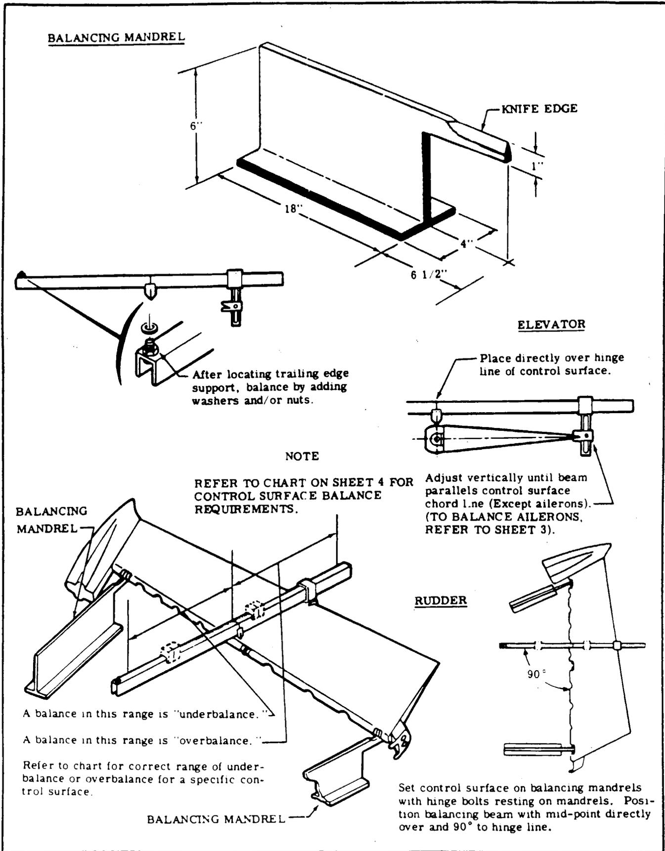
Figure 18-2. Control Surface Balancing (Sheet 1 of 4).
