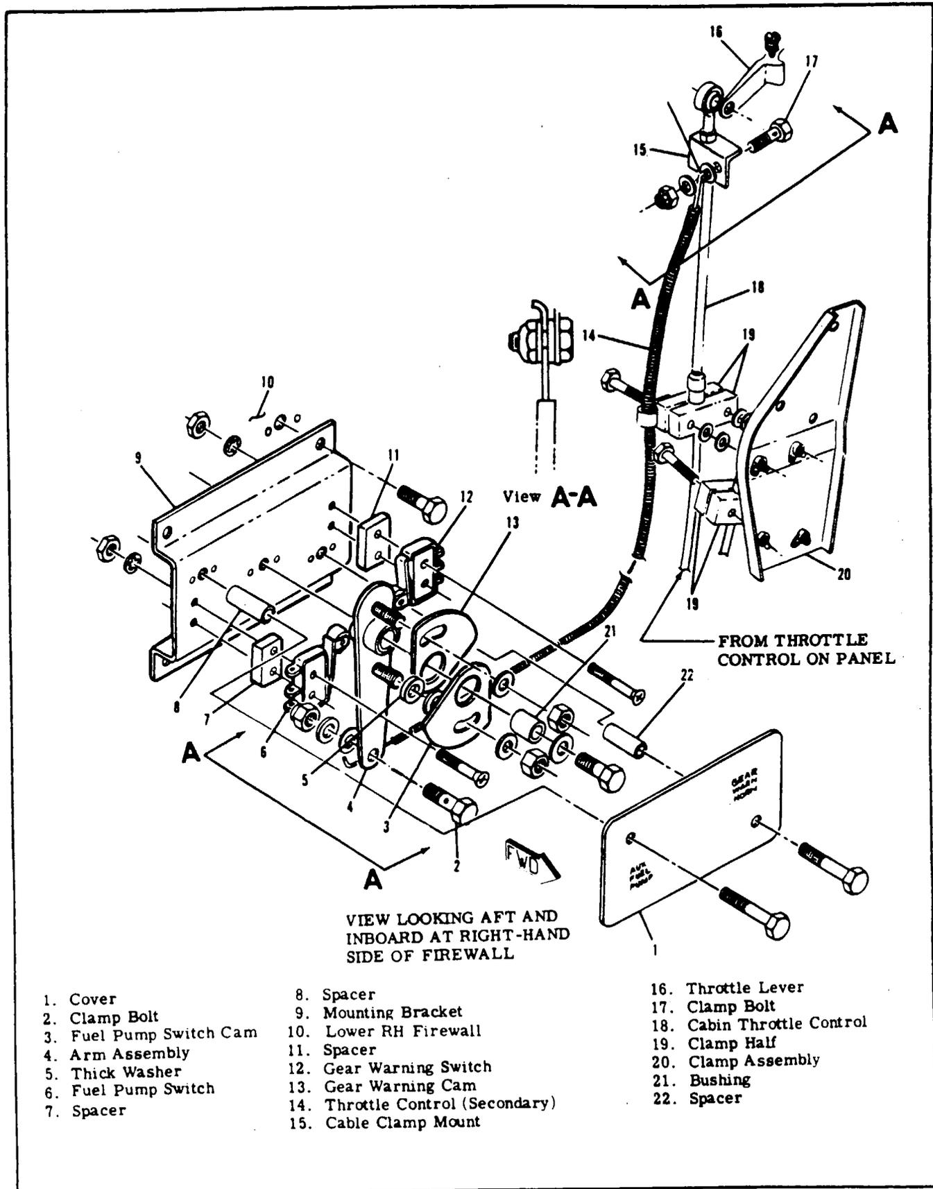
Figure 13-7. Throttle-Operated Microswitches
