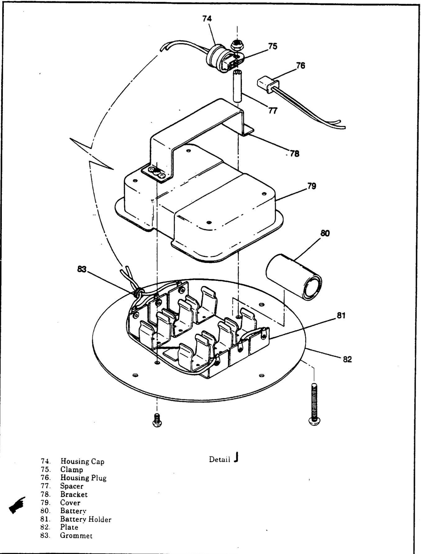
Figure 17-6B. Dual Alternator System Installation (Sheet 8 of 8)
