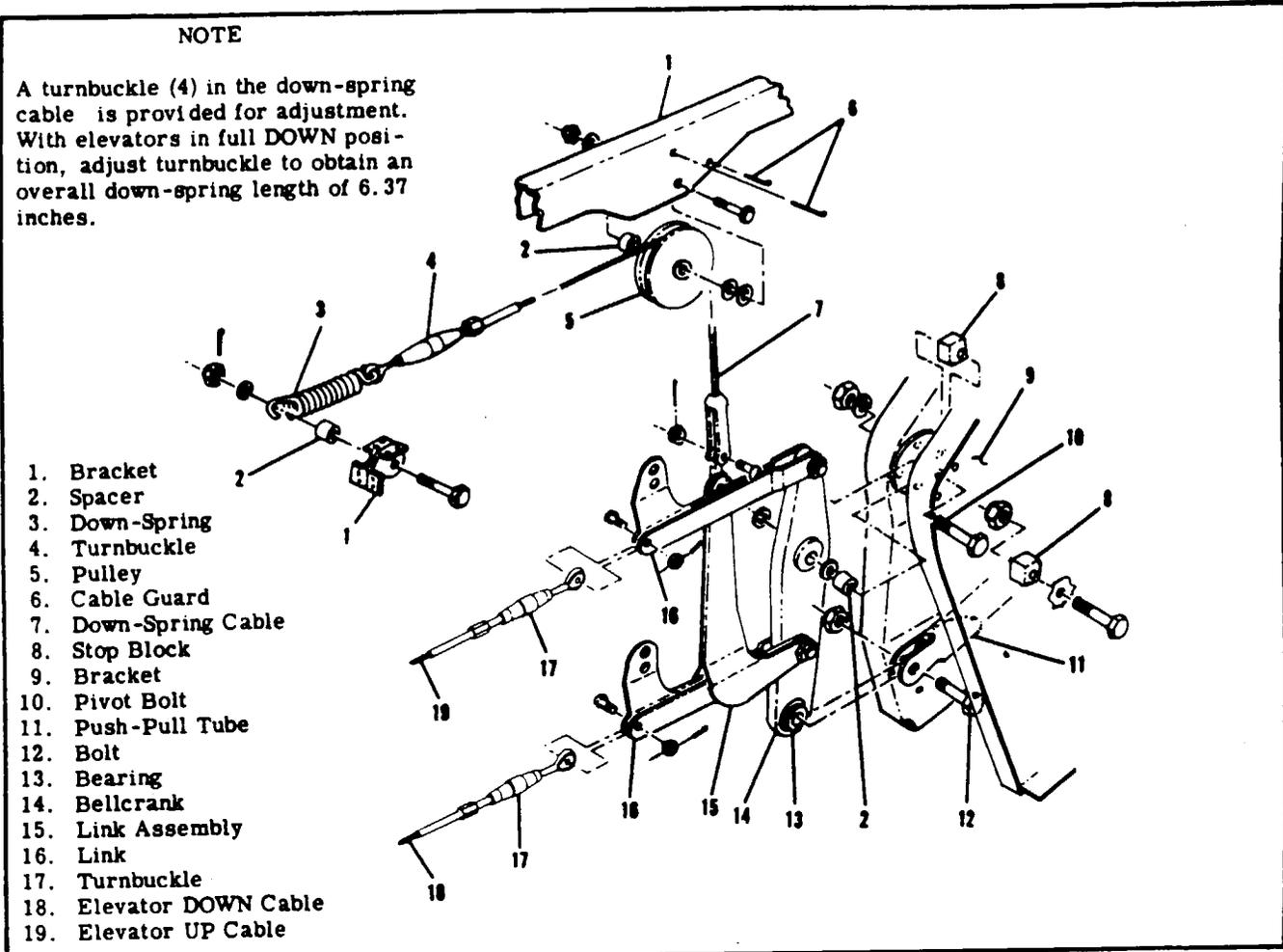
Figure 8-3. Elevator Bellcrank Installation
