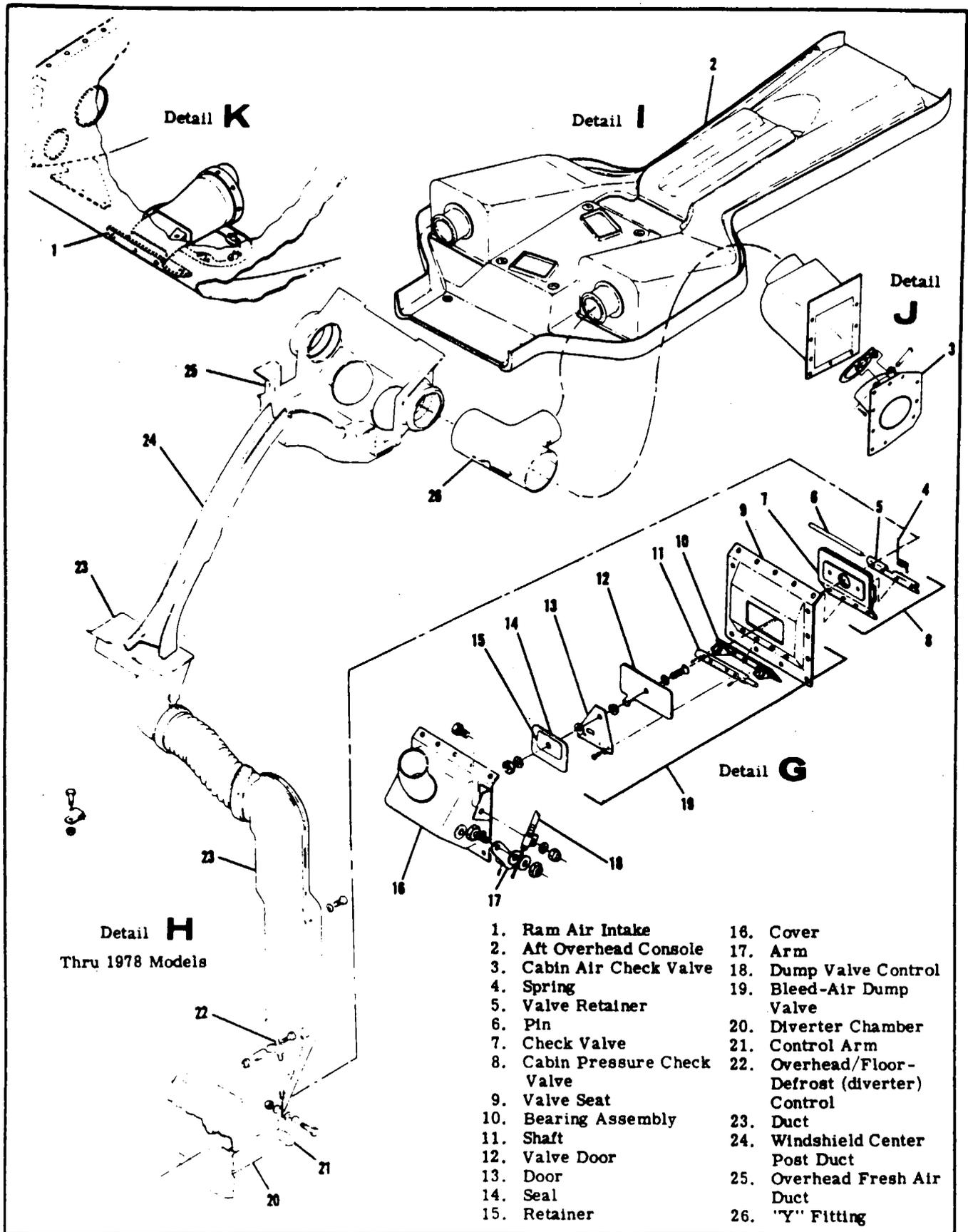
Figure 15-1. Heating, Ventilating and Pressurization System (Sheet 4 of 5)
