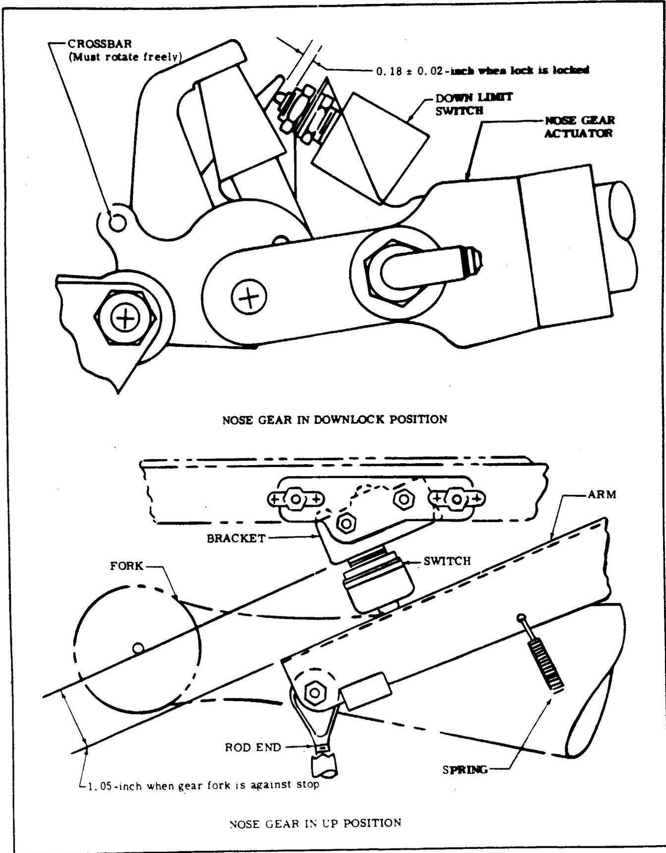
Figure 5A-14. Rigging Nose Landing Gear (Sheet 2 of 2)
