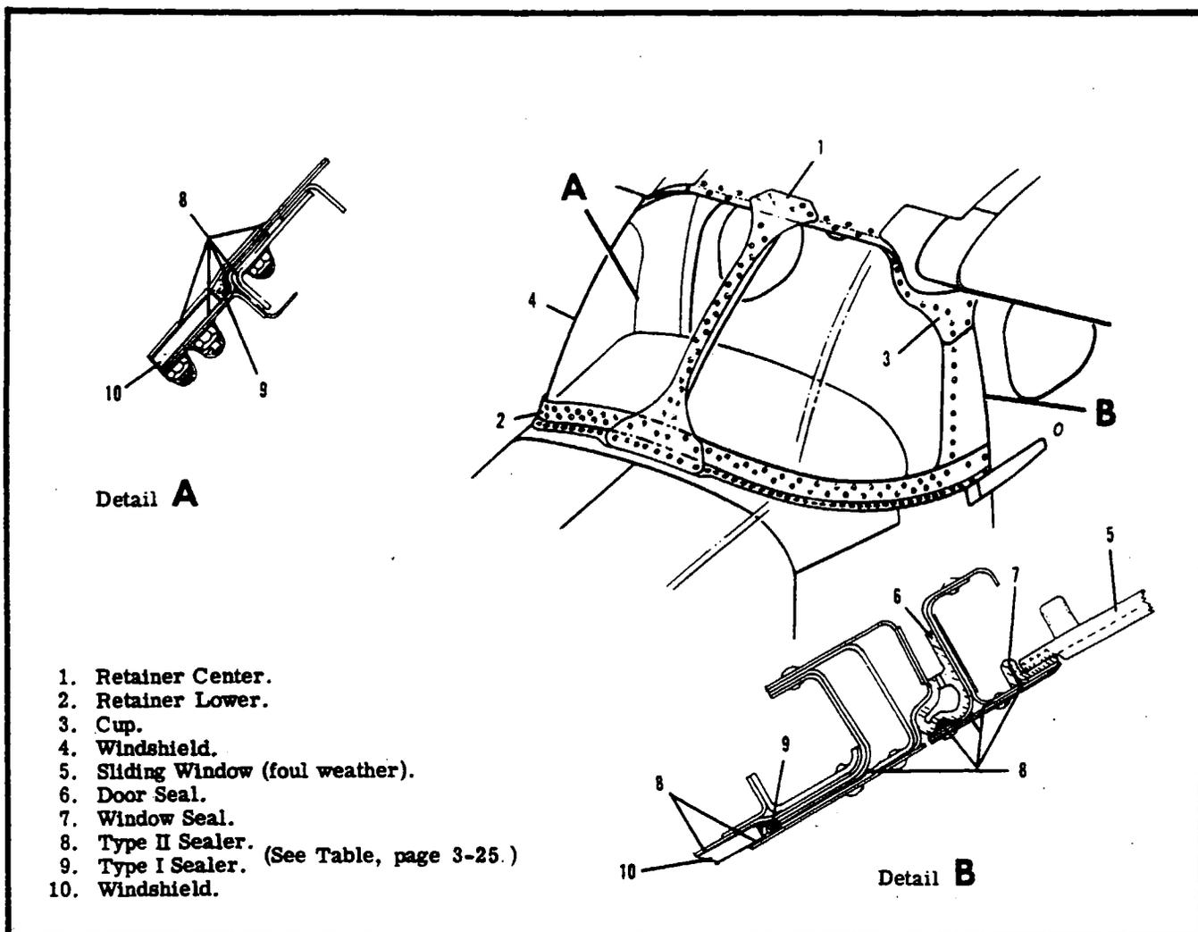
Figure 3-2. Windshield Installation.
