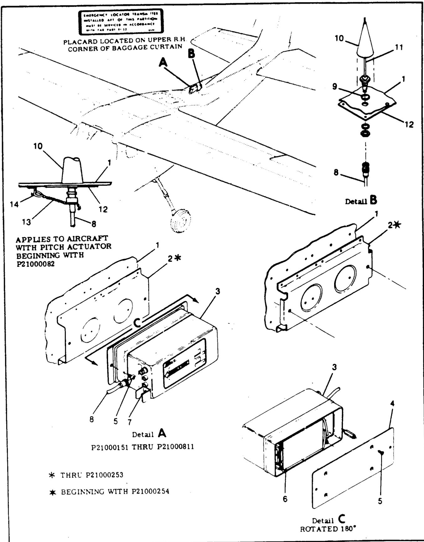
Figure 17-22. Emergency Locator Transmitter Installation (Sheet 2 of 3)
