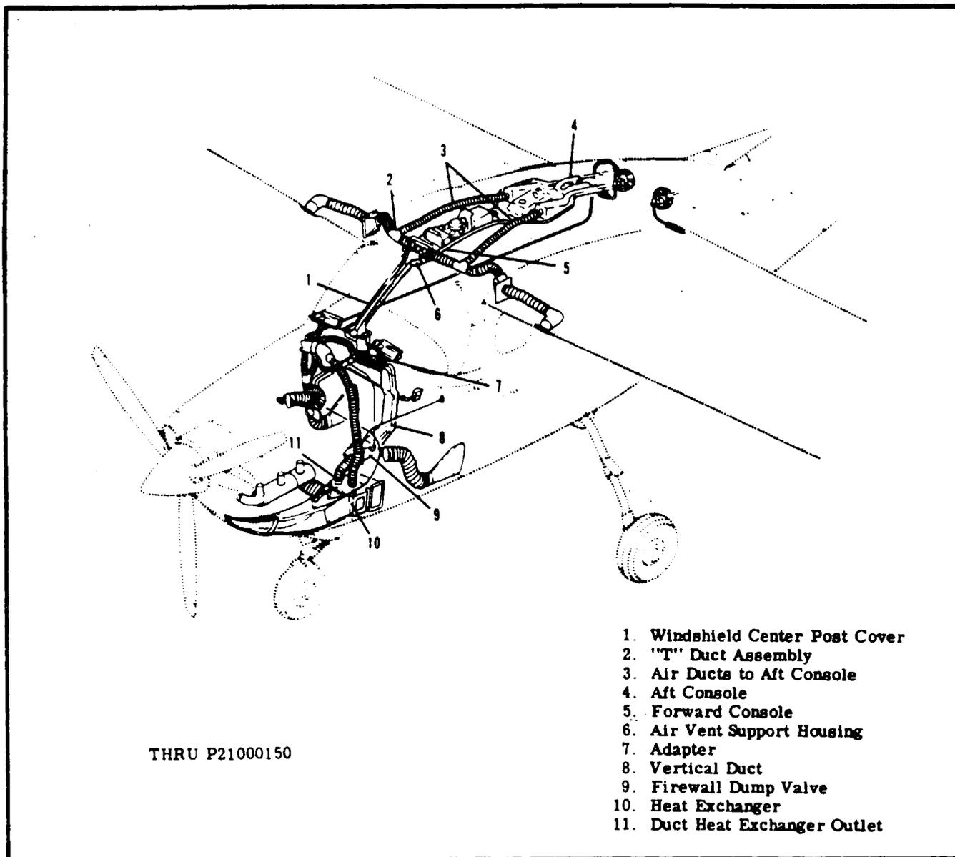
Figure 3-10. Ventilation System (Sheet 1 of 2)
