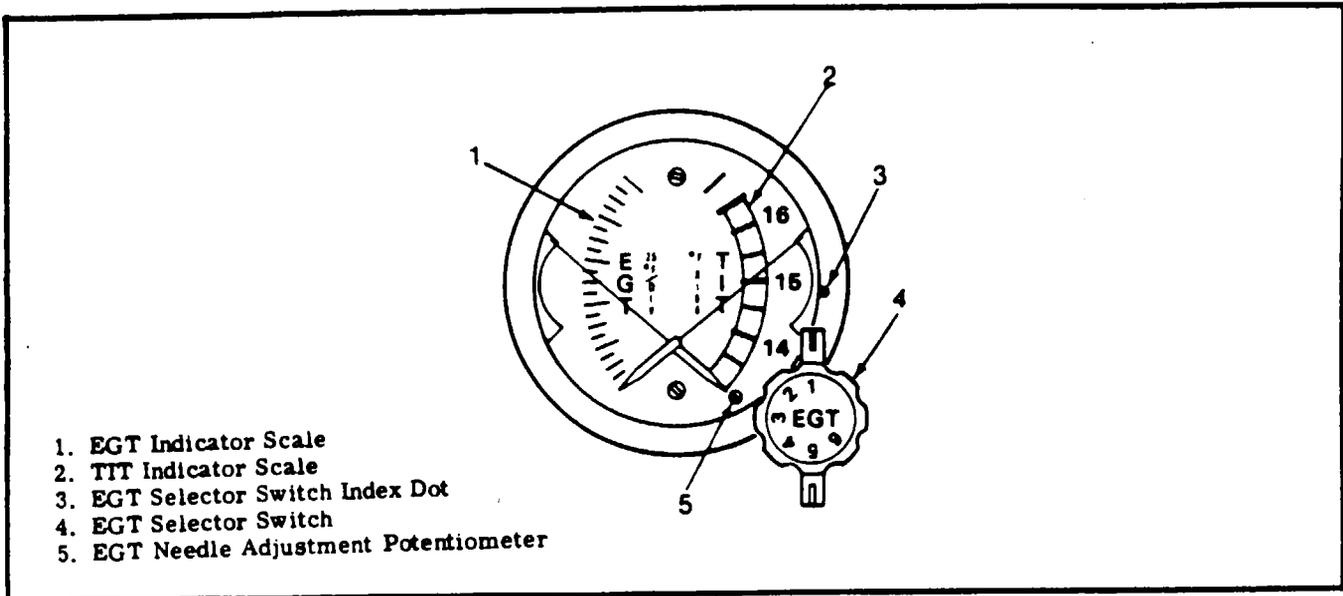
Figure 16-9. Turbine Inlet/ Six-Position Exhaust Gas Temperature Indicator
