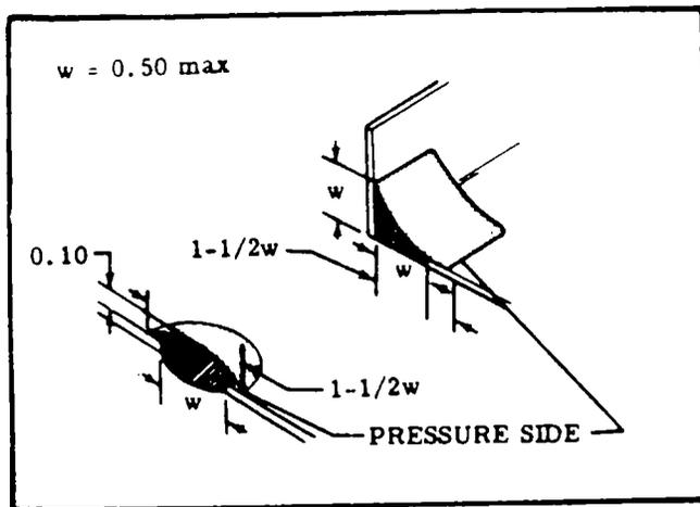
Figure 18-5. Hole Filling
