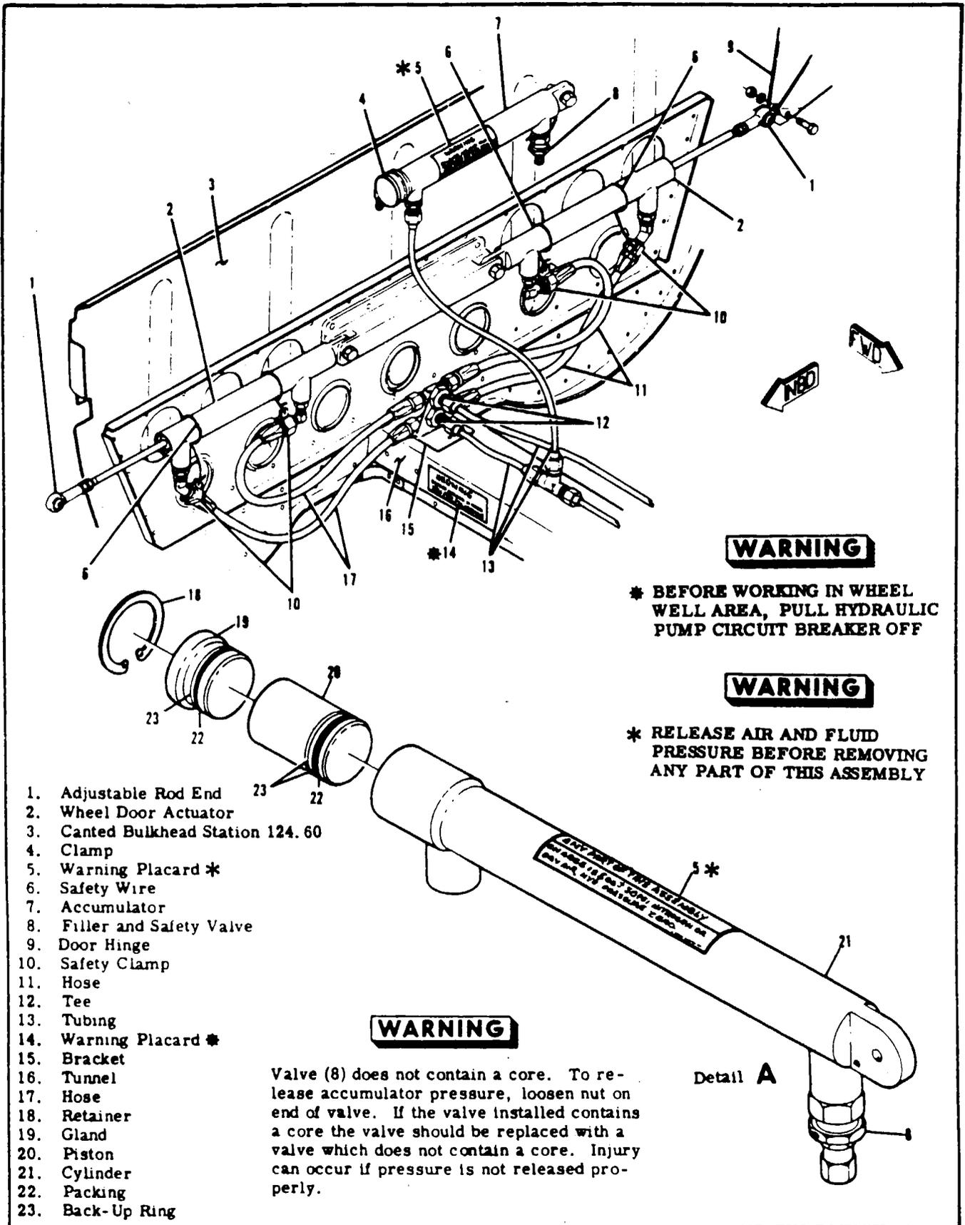
Figure 5-11. Main Landing Gear Wheel Door Close System Accumulator
