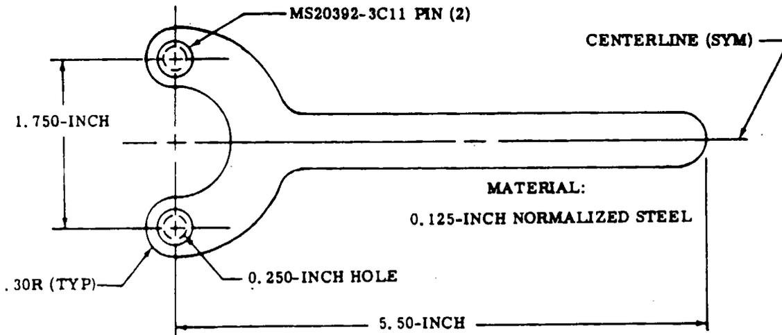
1. WRENCH USED TO INSTALL OR REMOVE END GLAND ON MAIN GEAR ACTUATOR.
