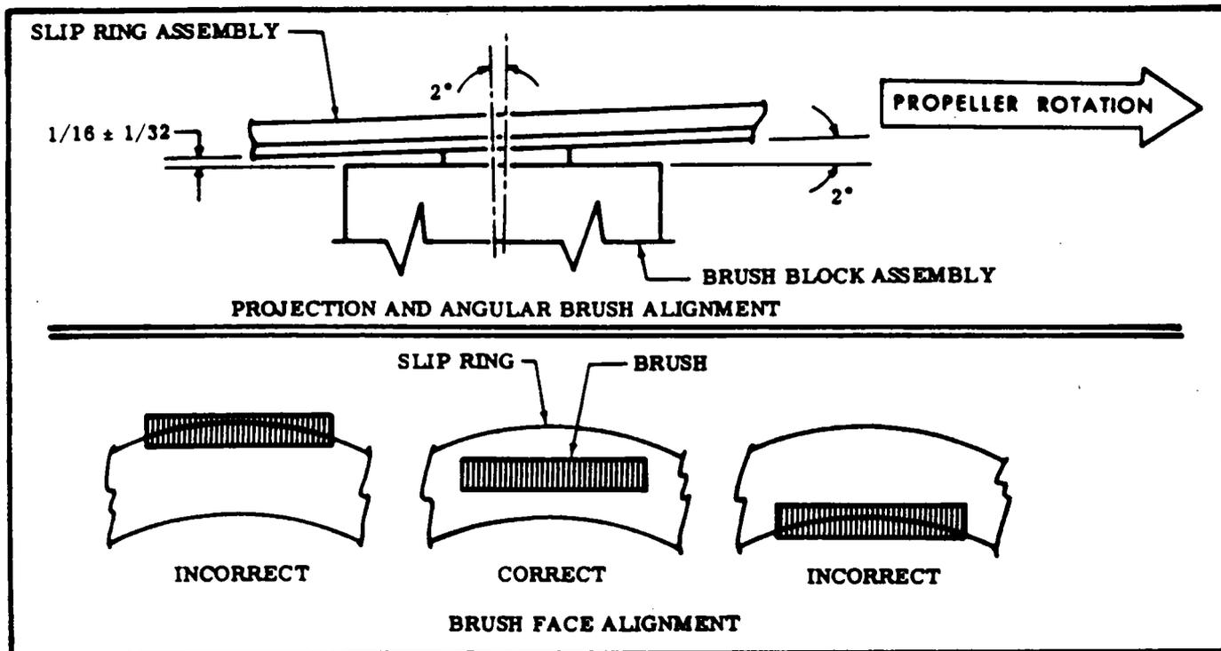
Figure 15-6. Brush Face Alignment and Projection and Angular Brush Alignment
