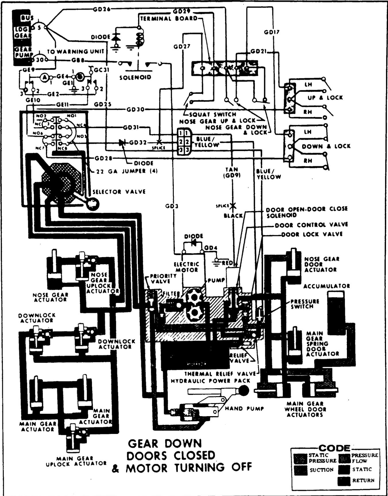
Figure 5-38: Hydraulic and Electrical System Schematic (Sheet 6 of 7)
