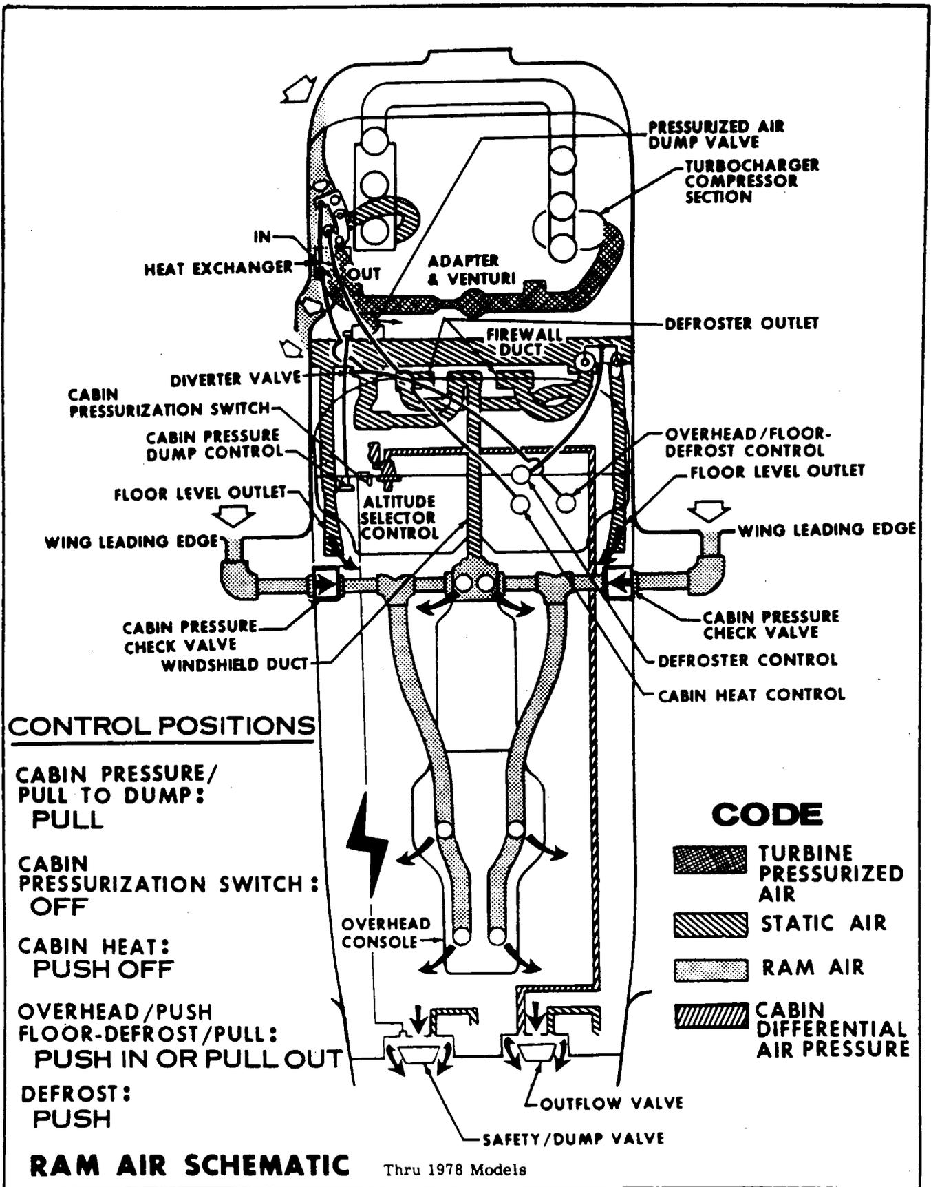
Figure 15-2. Cabin Air Flow Schematic (Sheet 1 of 6)
