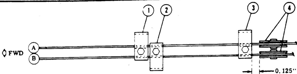
1. With elevators in neutral, set trim tab to neutral (split the non-faired difference between the inboard and outboard ends).
