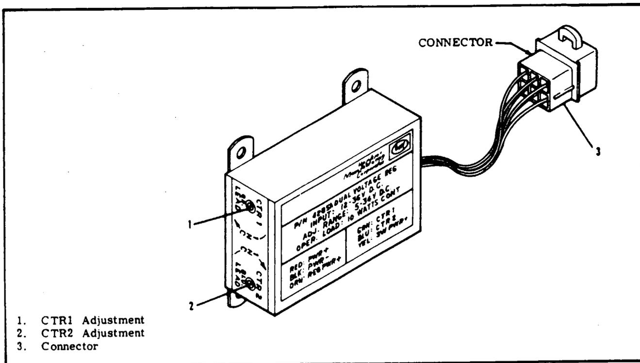
Figure 9-7. Dual Voltage Regulator
