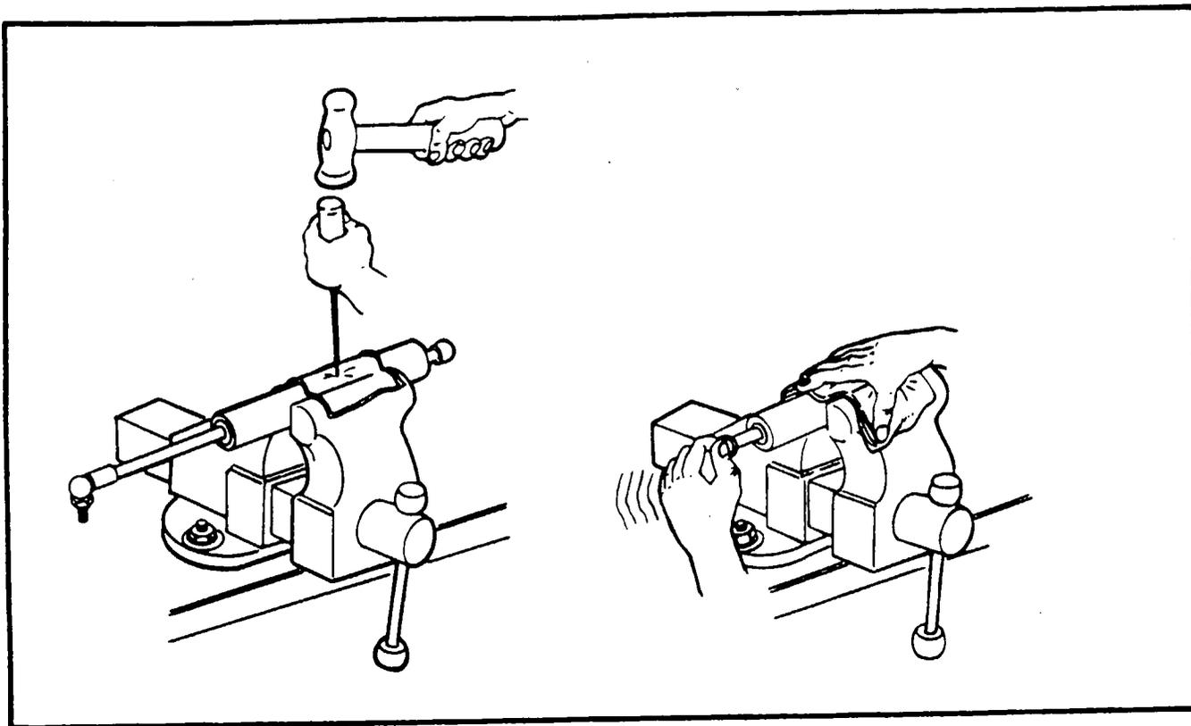
Figure 3-6A. Disposal of Gas Spring Assembly
