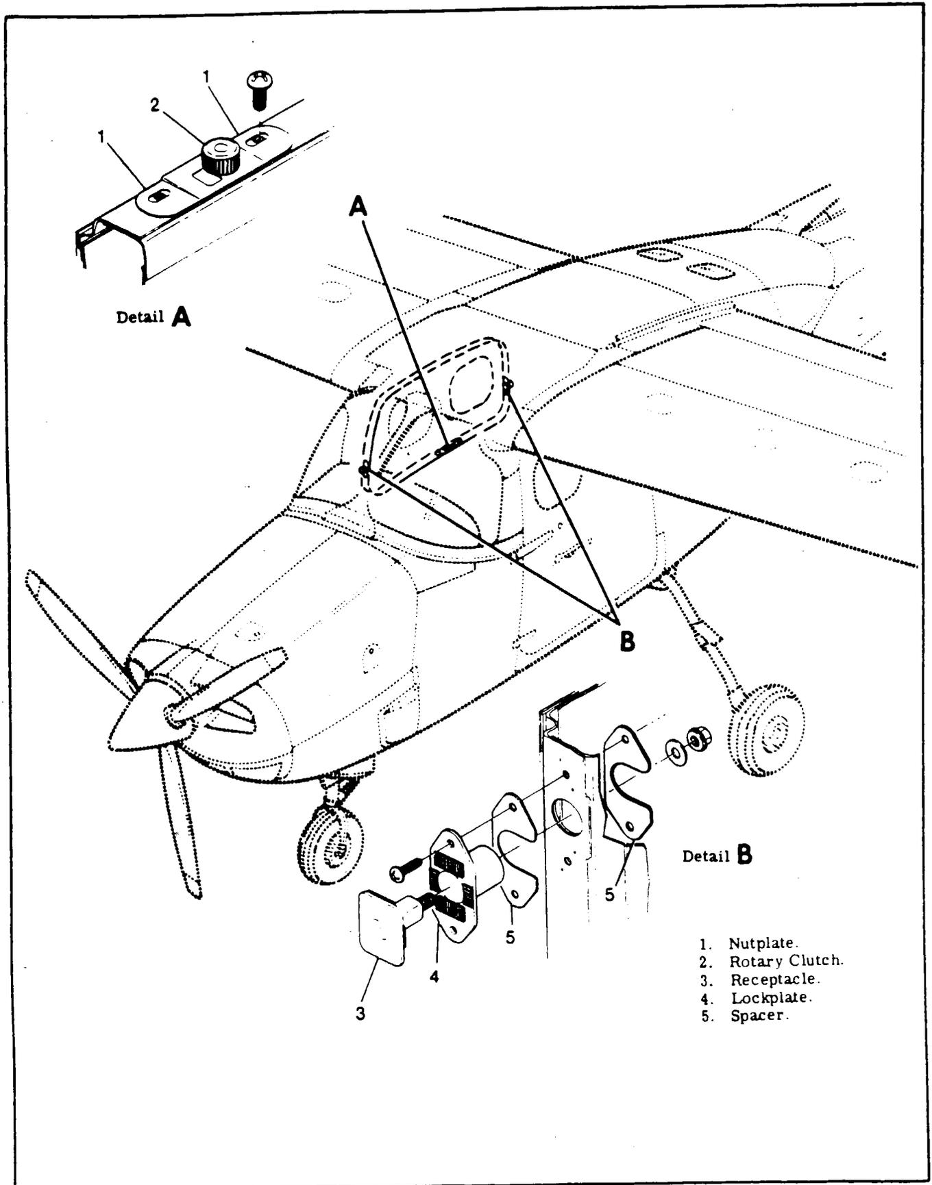
Figure 3-6. Emergency Exit Door Installation (Sheet 1 of 2).
