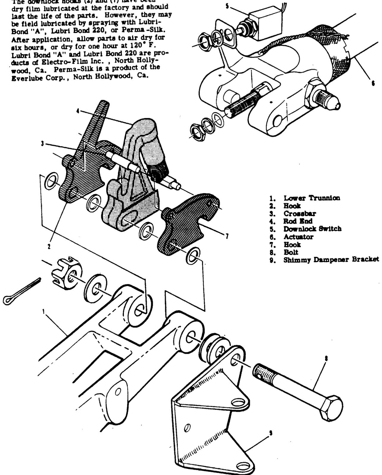
Figure 5-20. Nose Gear Downlock Mechanism
