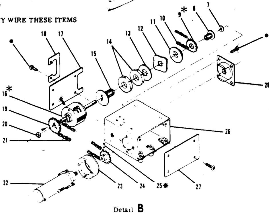
Figure 9-6 Electric Elevator Trim Assist Installation
