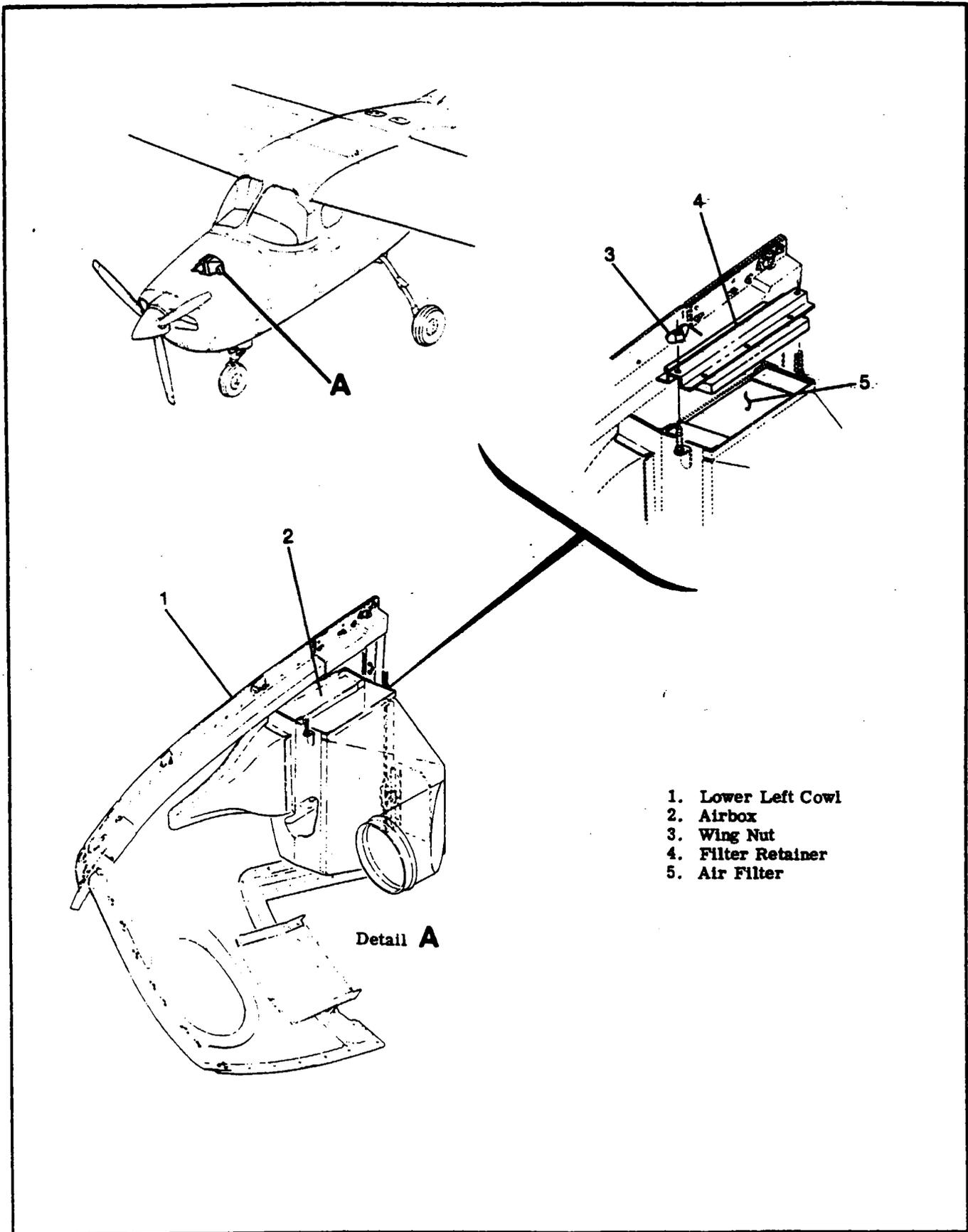
Figure 12-9. Airbox Installation
