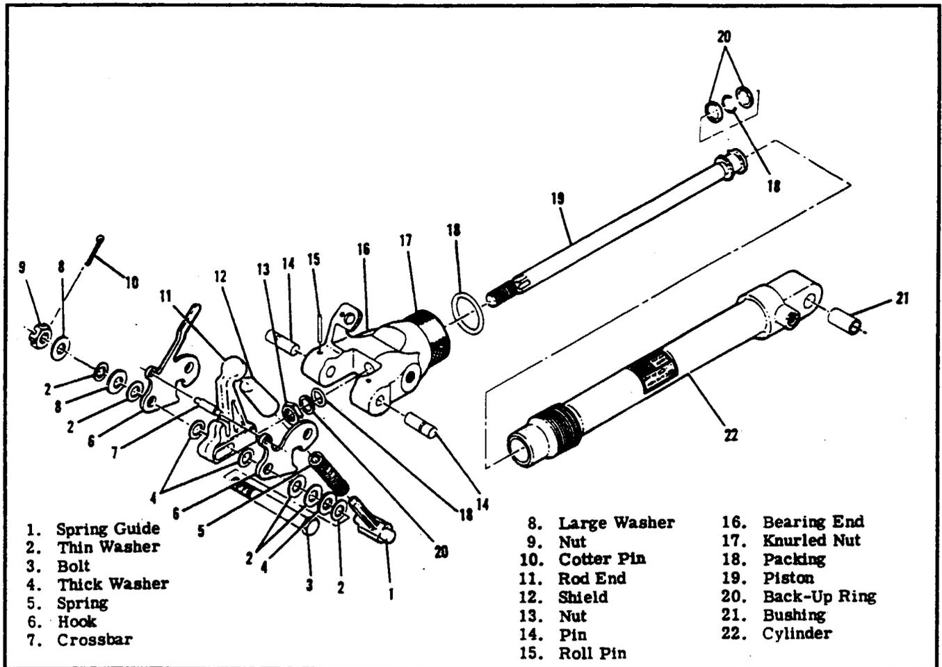
Figure 5-21. Nose Gear Actuator
