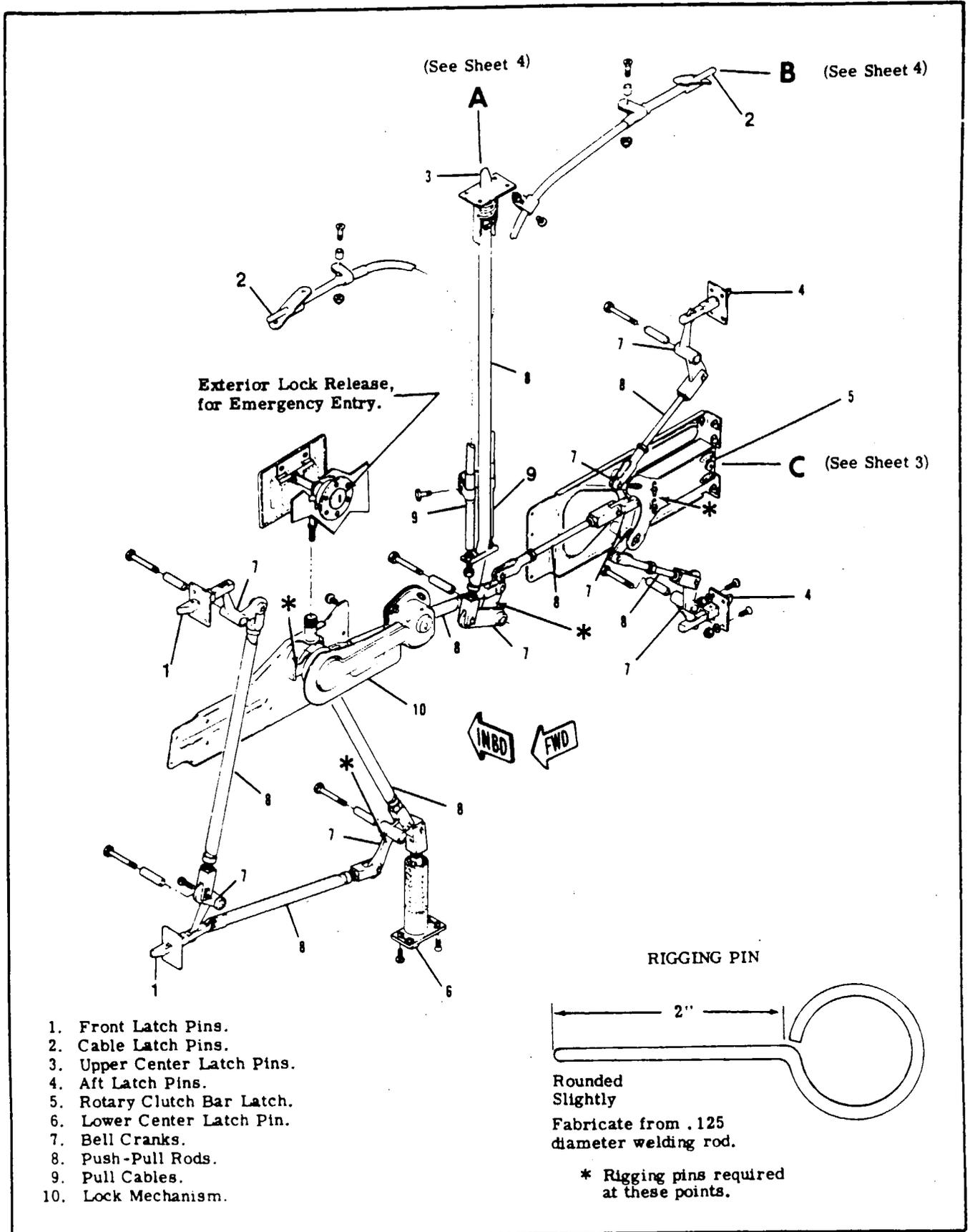
Figure 3-5. Door Latch Mechanism (Sheet 1 of 4)
