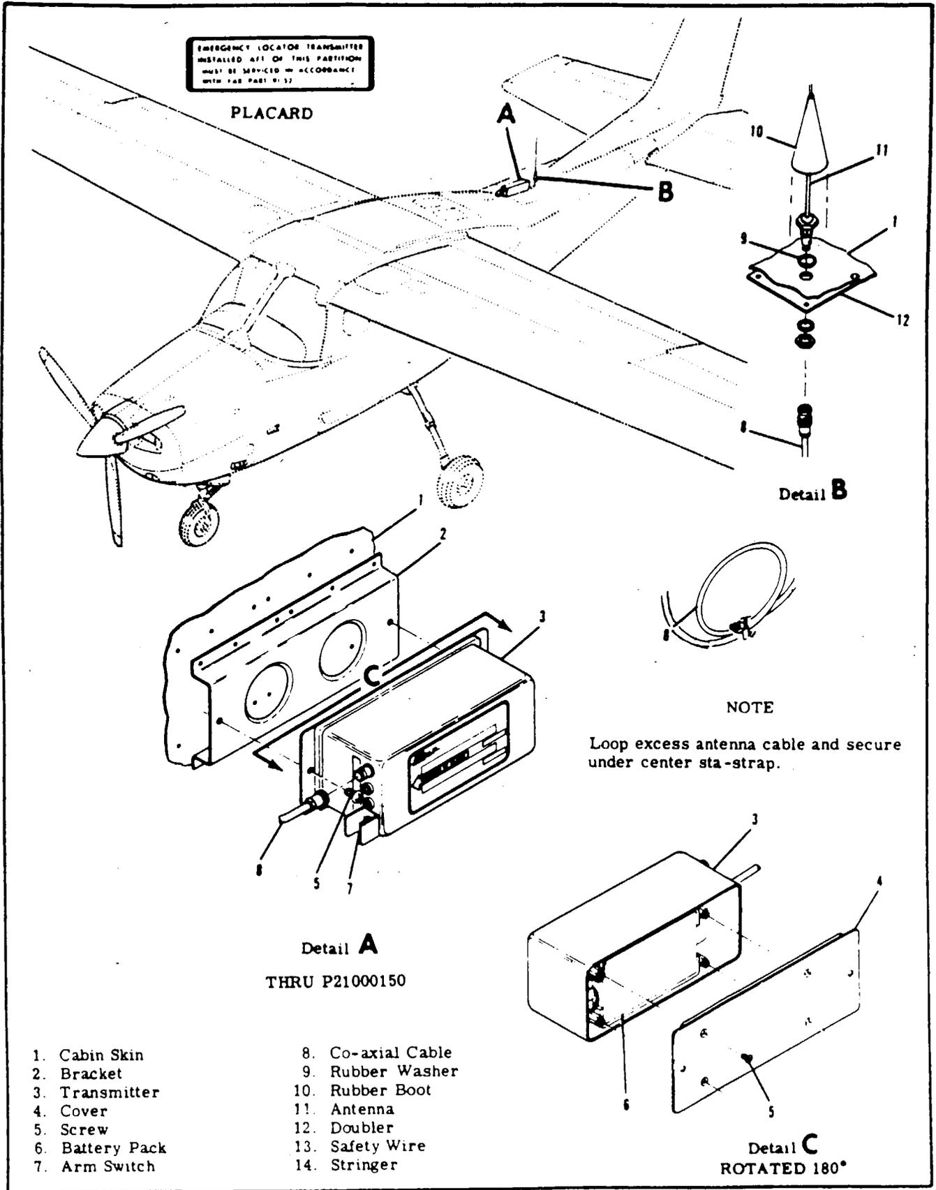
Figure 17-22. Emergency Locator Transmitter Installation (Sheet 1 of 3)
