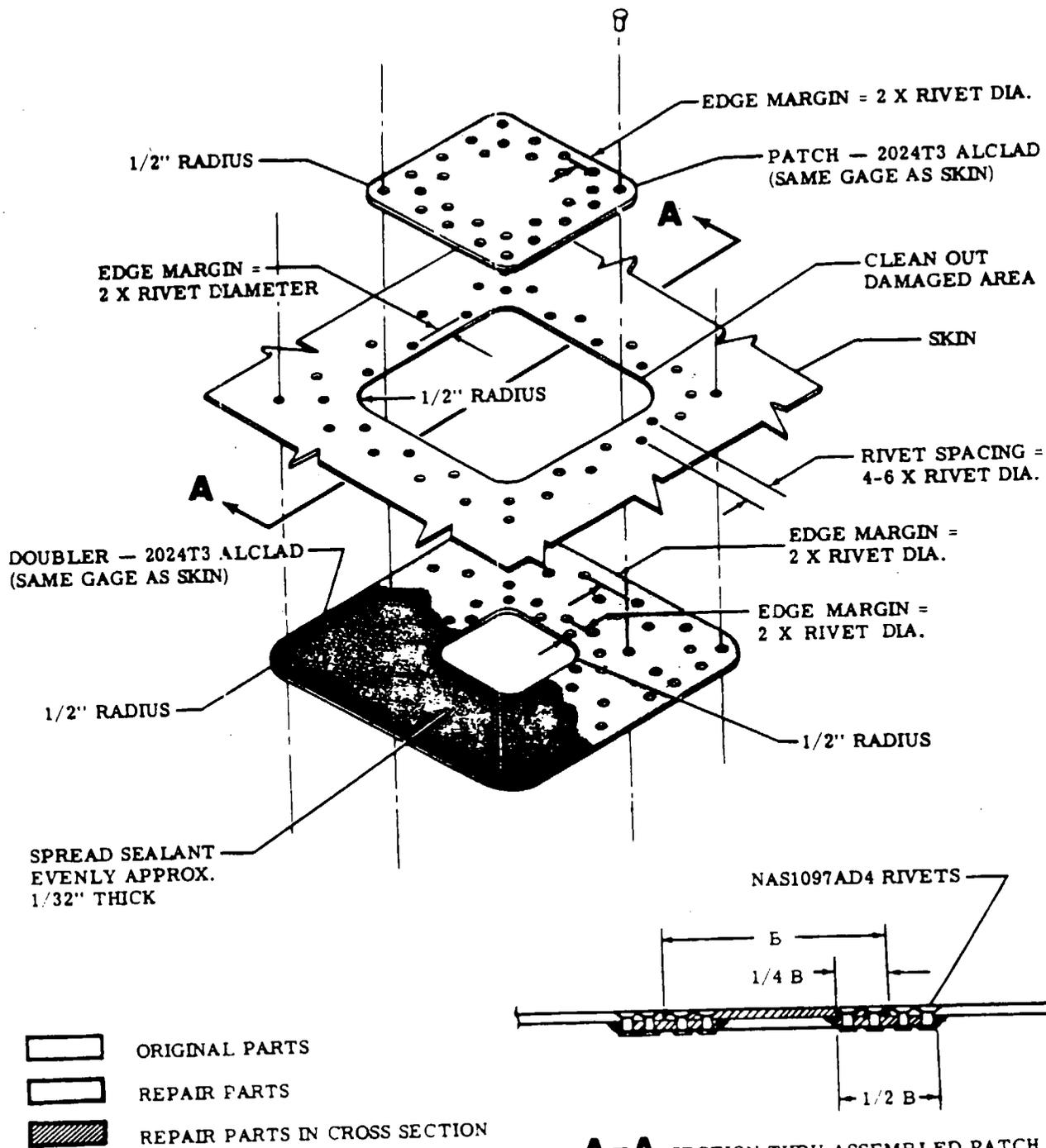
Figure 18-16. Typical Insert Patch in Pressure Cabin
