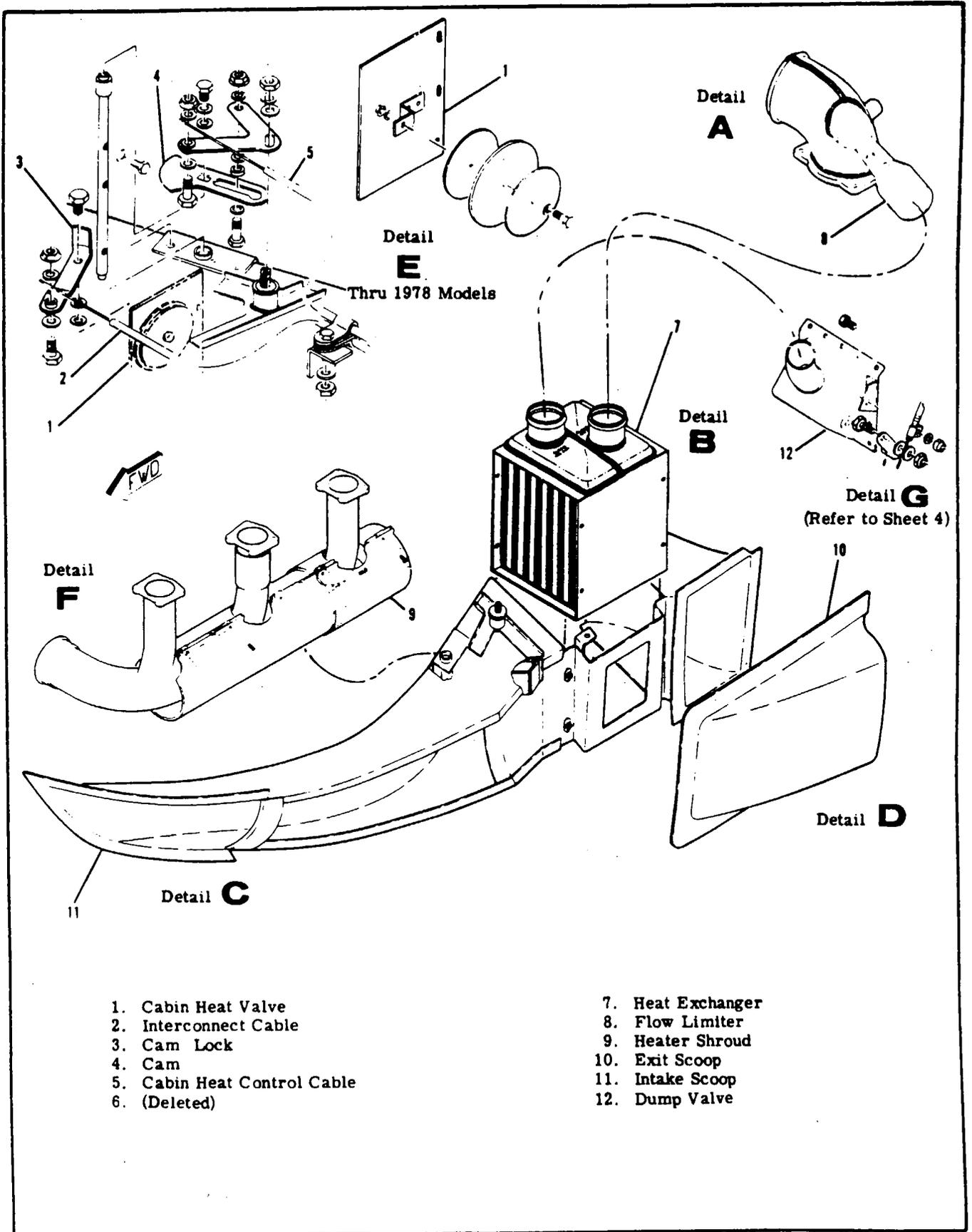
Figure 15-1. Heating, Ventilating and Pressurization System (Sheet 3 of 5)
