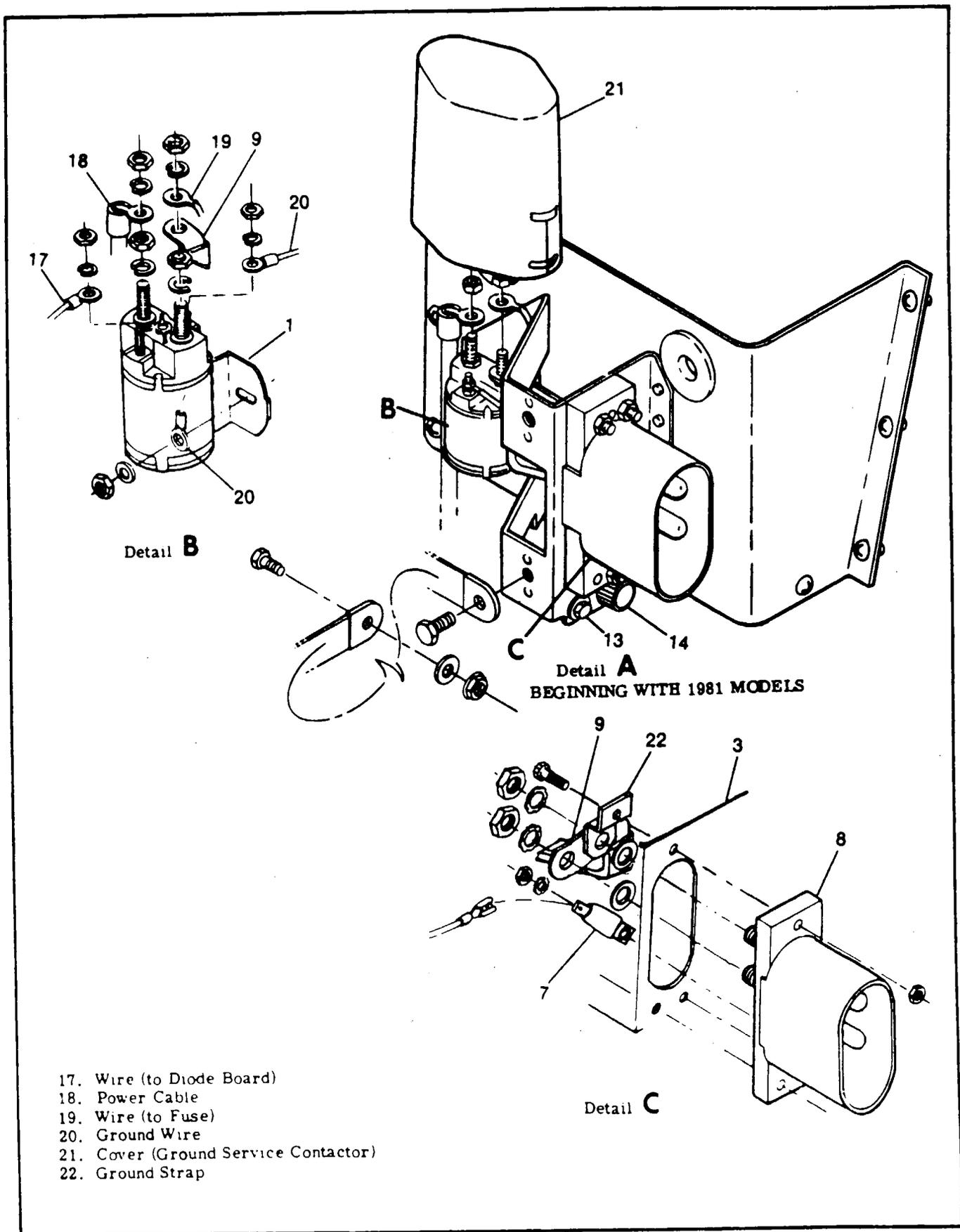
Figure 17-3. Ground Service Receptacle Installation (Sheet 2 of 2)
