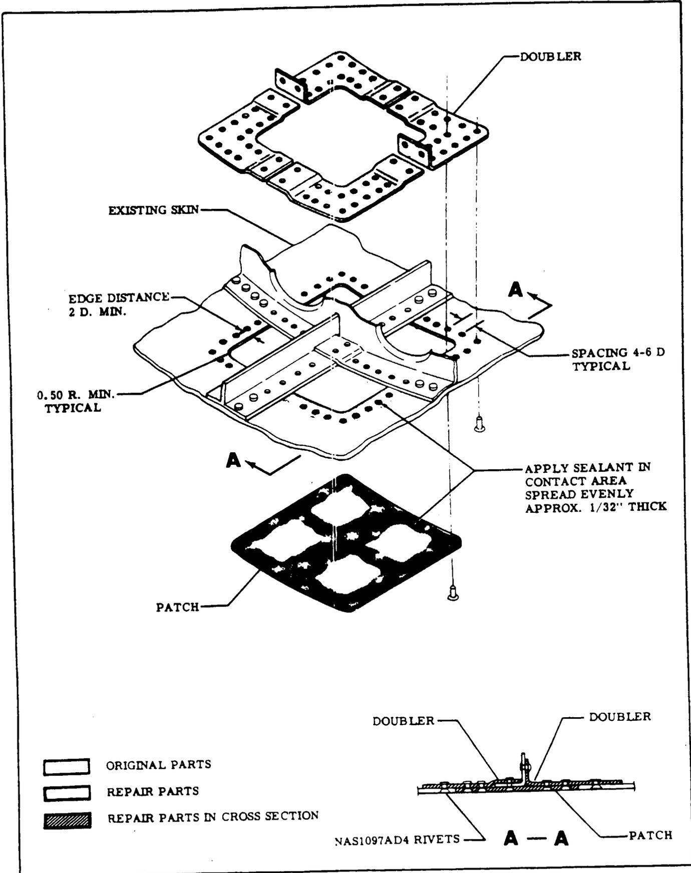
Figure 18-11. Over Structure Repair of Pressure Cabin
