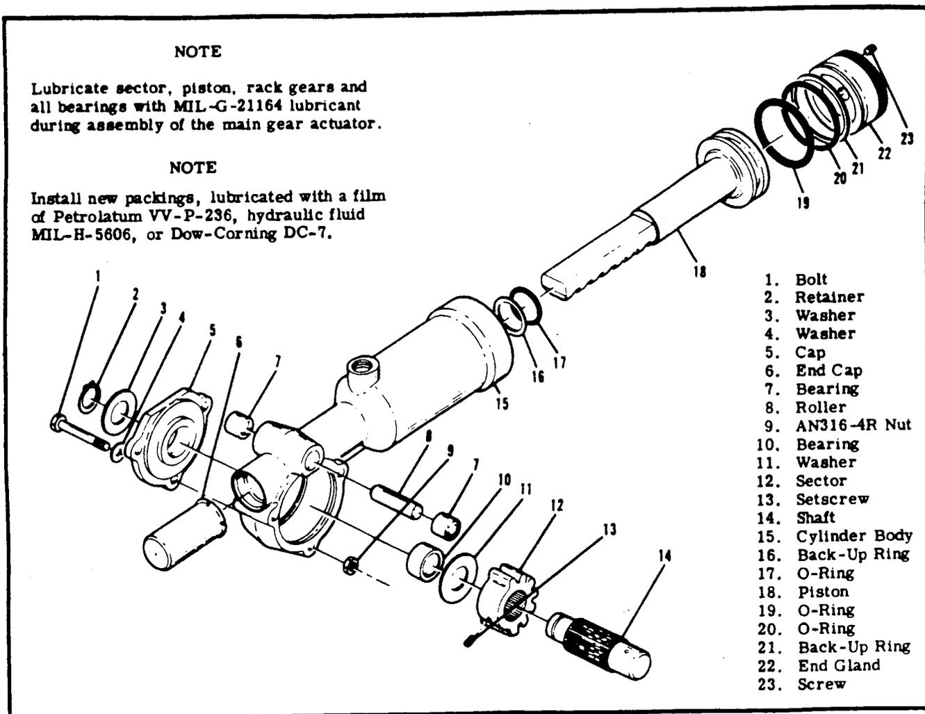
Figure 5-2. Main Landing Gear Actuator Assembly
