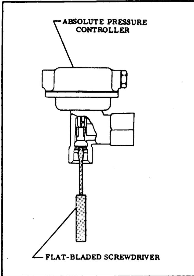
Figure 12-18. Controller Adjustment
