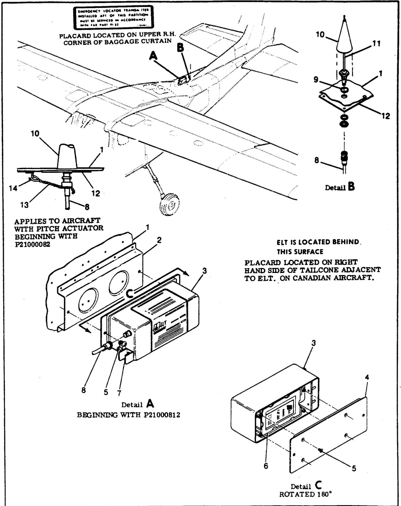
Figure 17-22. Emergency Locator Transmitter Installation (Sheet 3 of 3)
