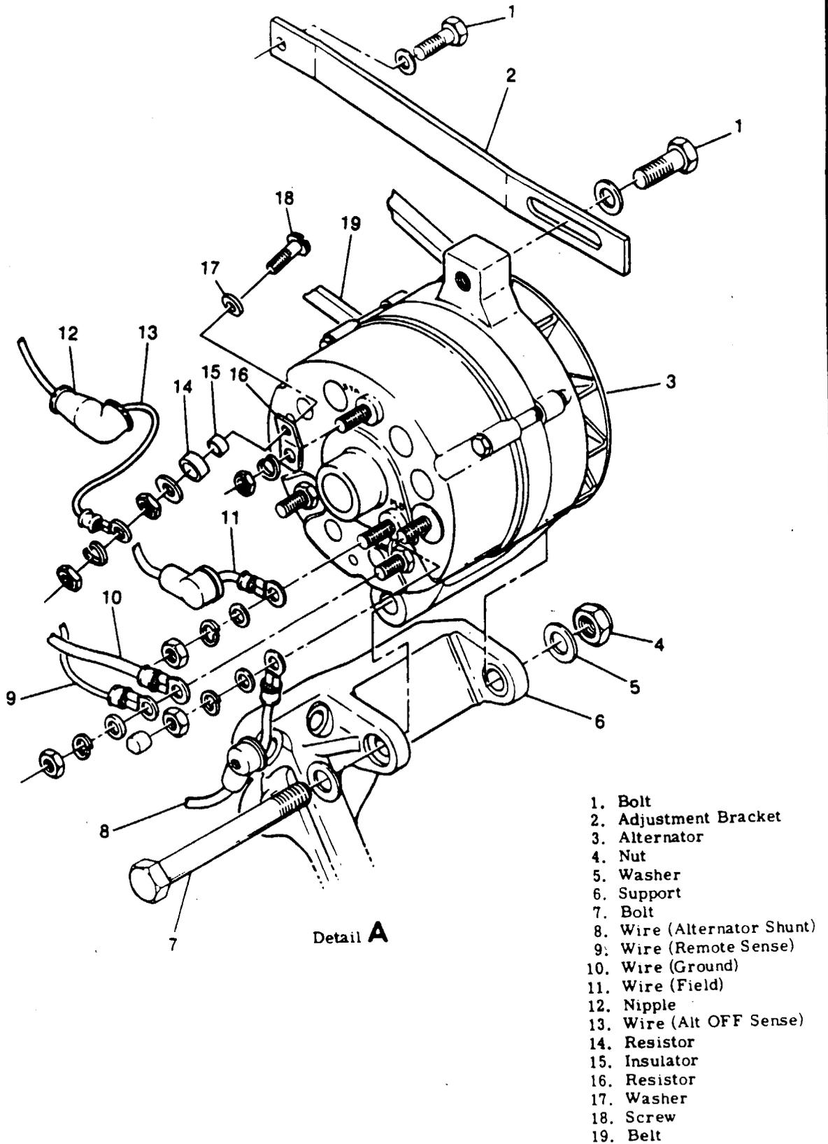
Figure 17-6B. Dual Alternator System Installation (Sheet 2 of 8)
