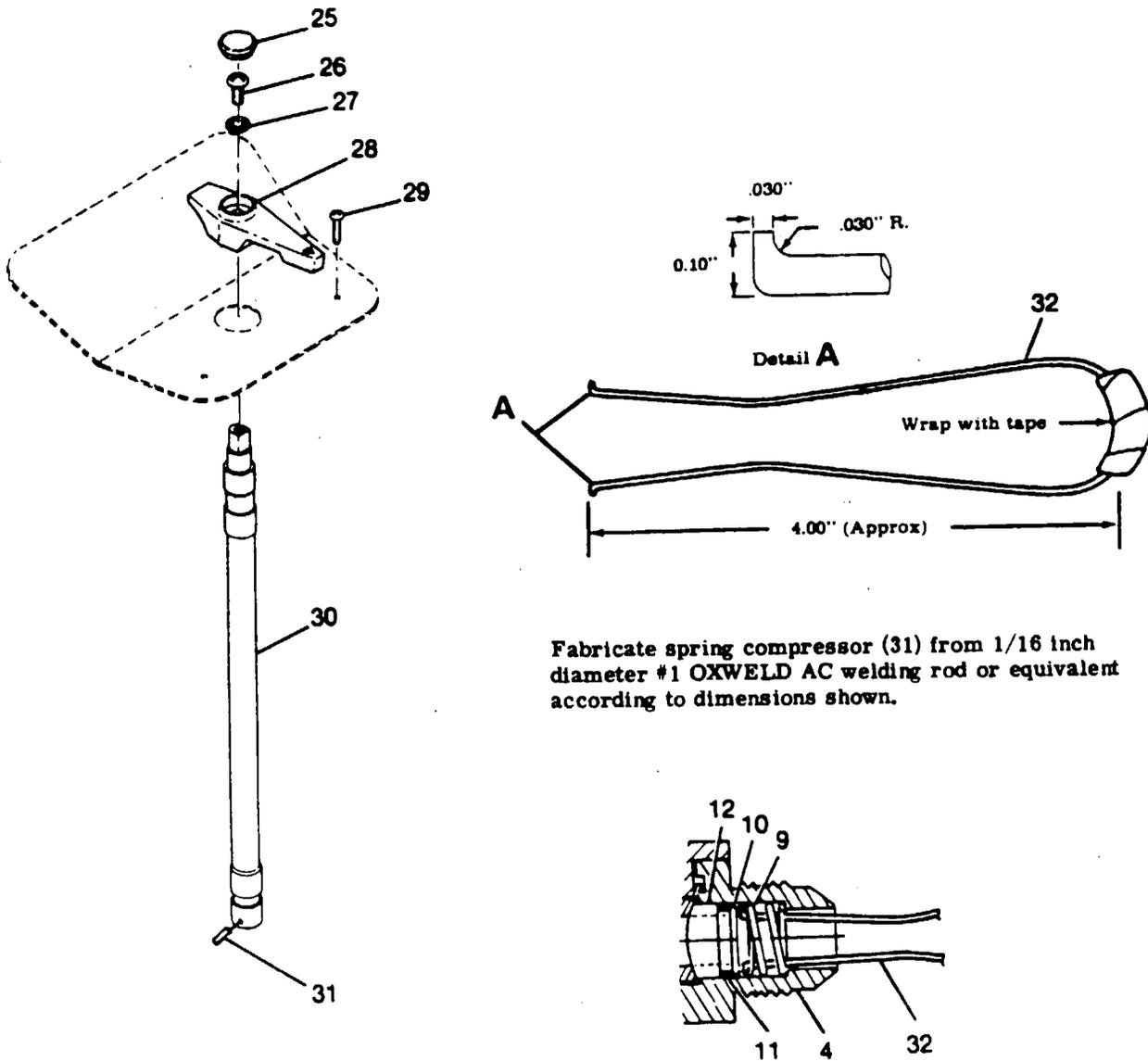
Fabricate spring compressor (31) from 1/16 inch diameter #1 OXWELD AC welding rod or equivalent according to dimensions shown.
