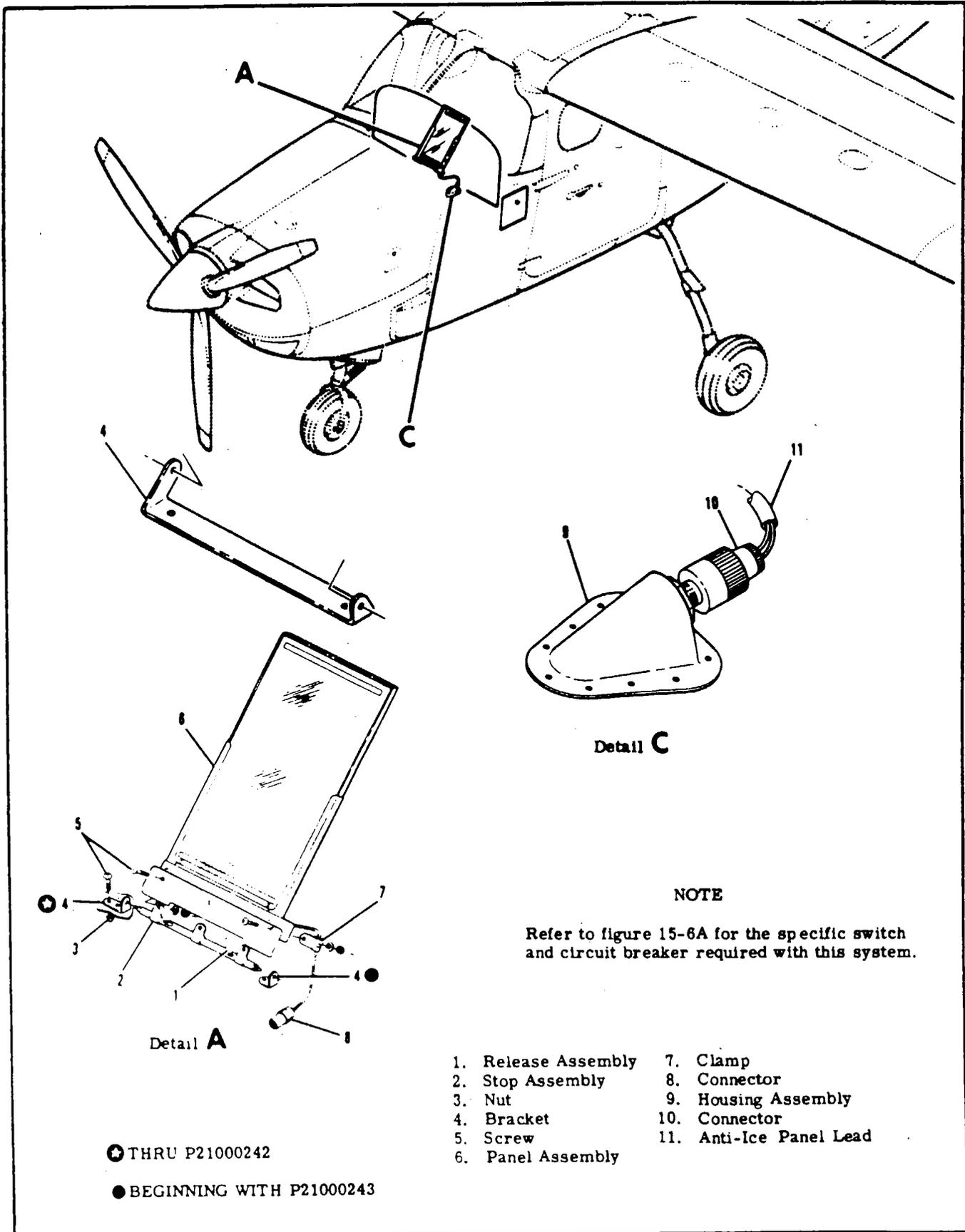
Figure 15-6B. Windshield Anti-Ice Panel Installation (Removable)
