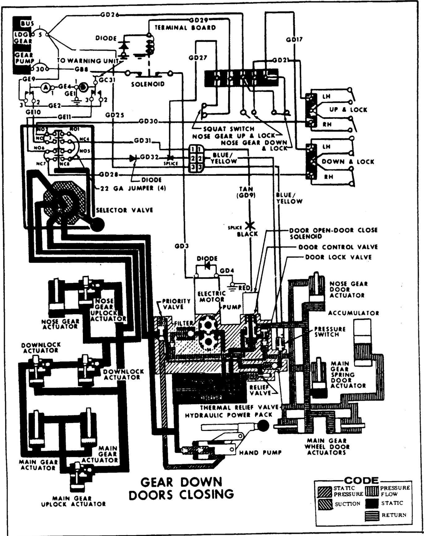
Figure 5-38. Hydraulic and Electrical System Schematic (Sheet 5 of 7)
