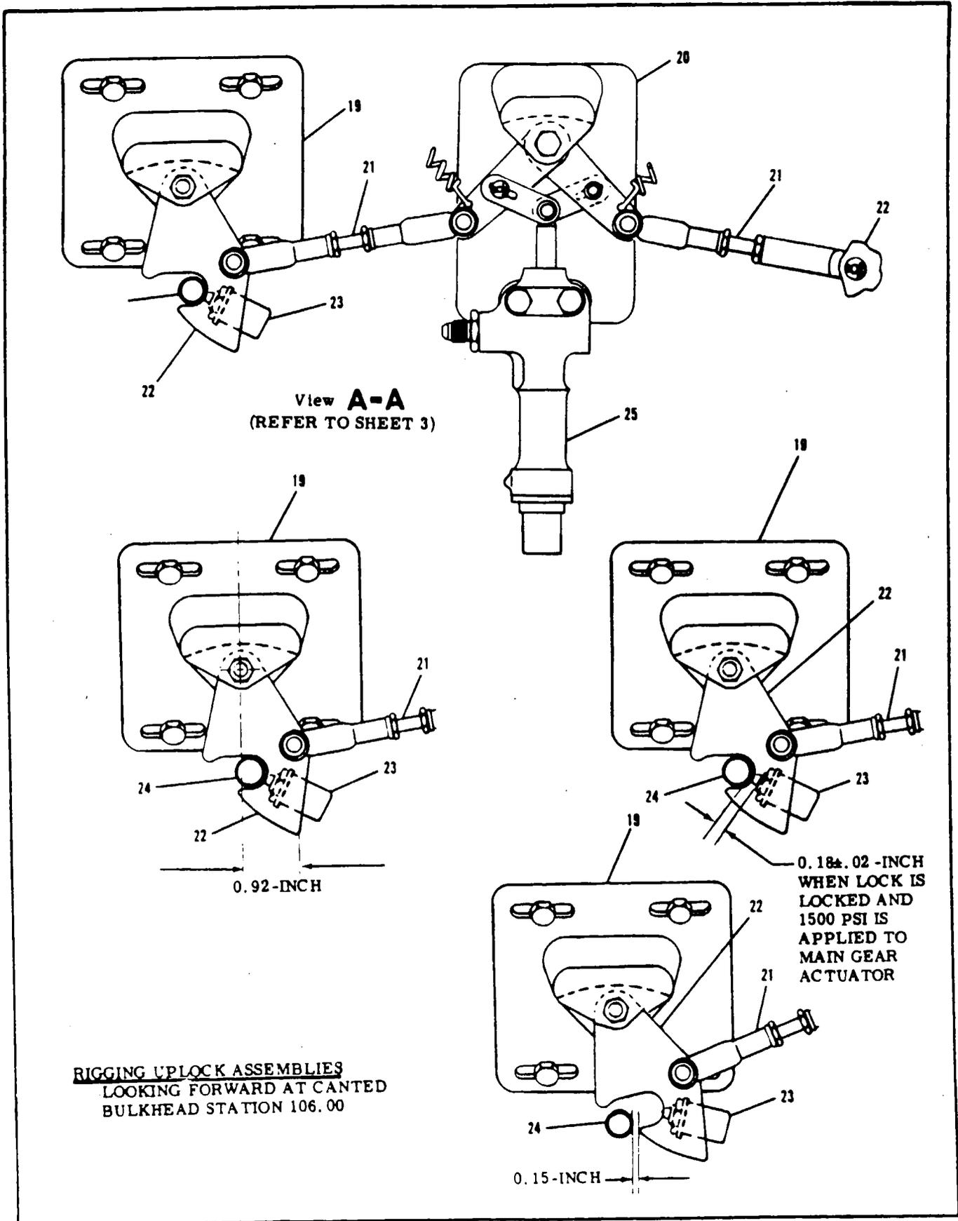
Figure 5-36. Rigging Main Landing Gear (Sheet 4 of 4)
