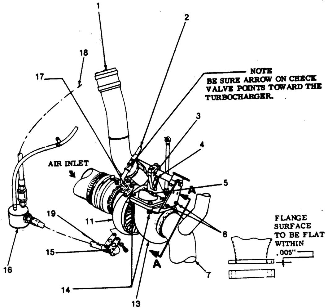
1. Turbocharger Discharge Duct
