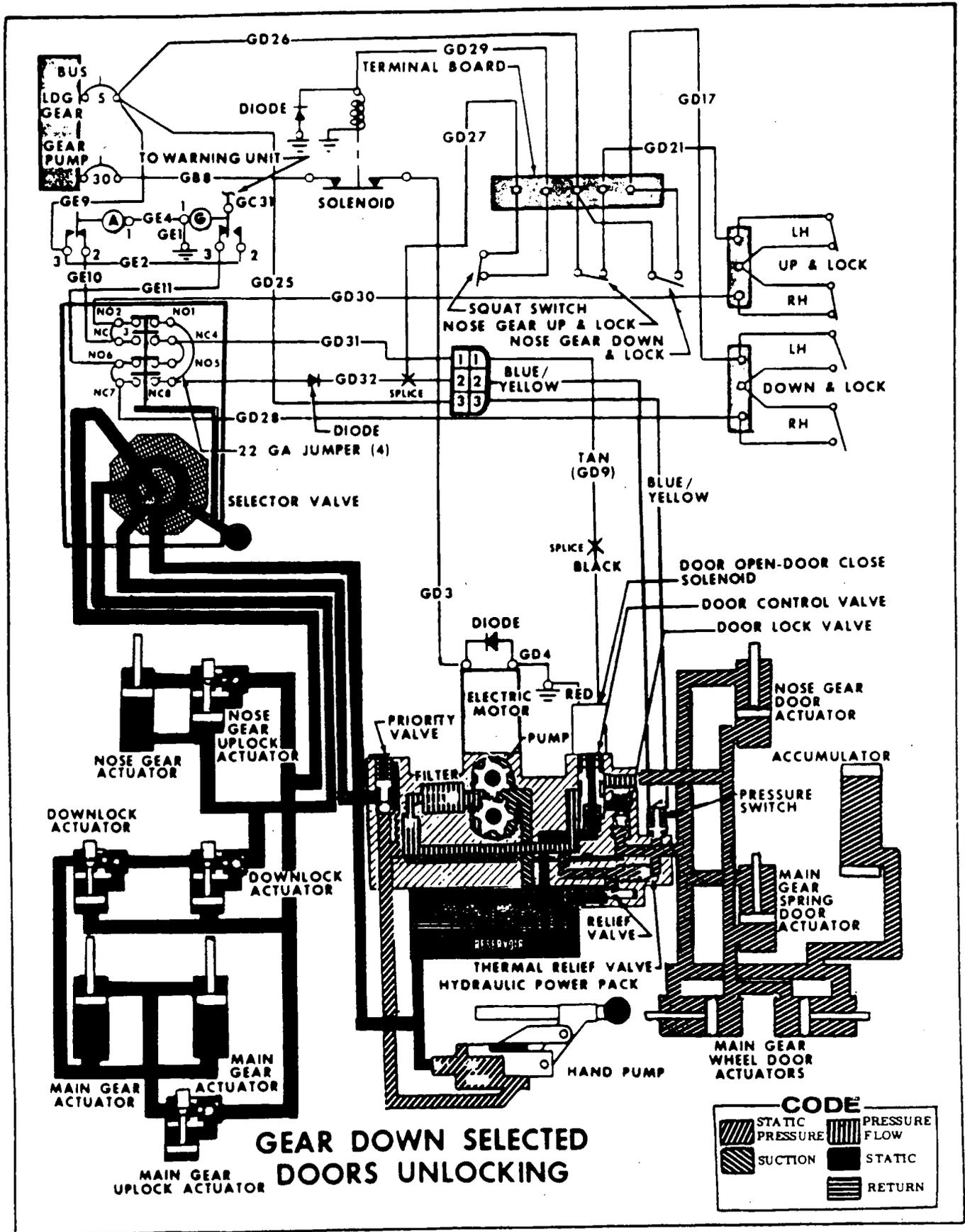
Figure 5-38. Hydraulic and Electrical System Schematic (Sheet 1 of 7)
