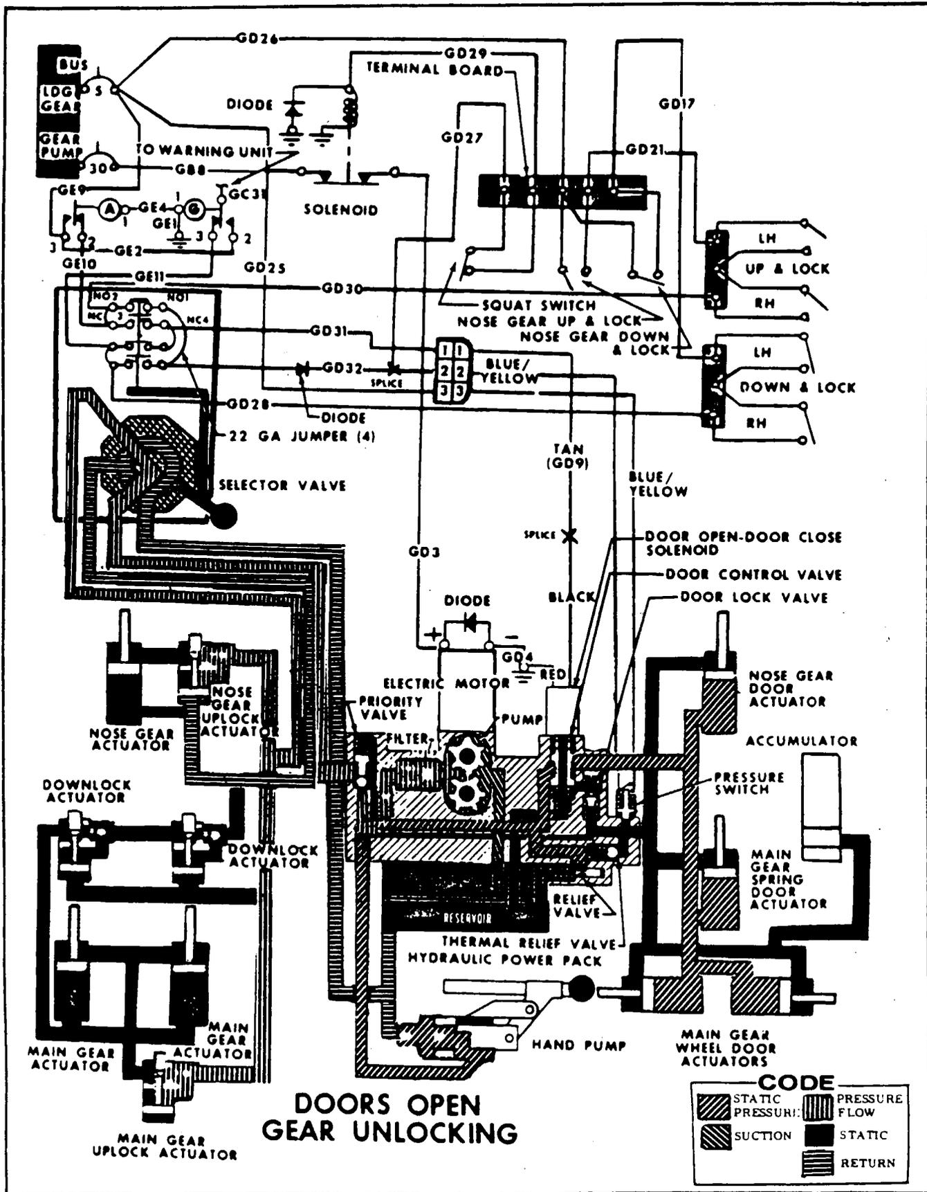
Figure 5-38. Hydraulic and Electrical System Schematic (Sheet 3 of 7)
