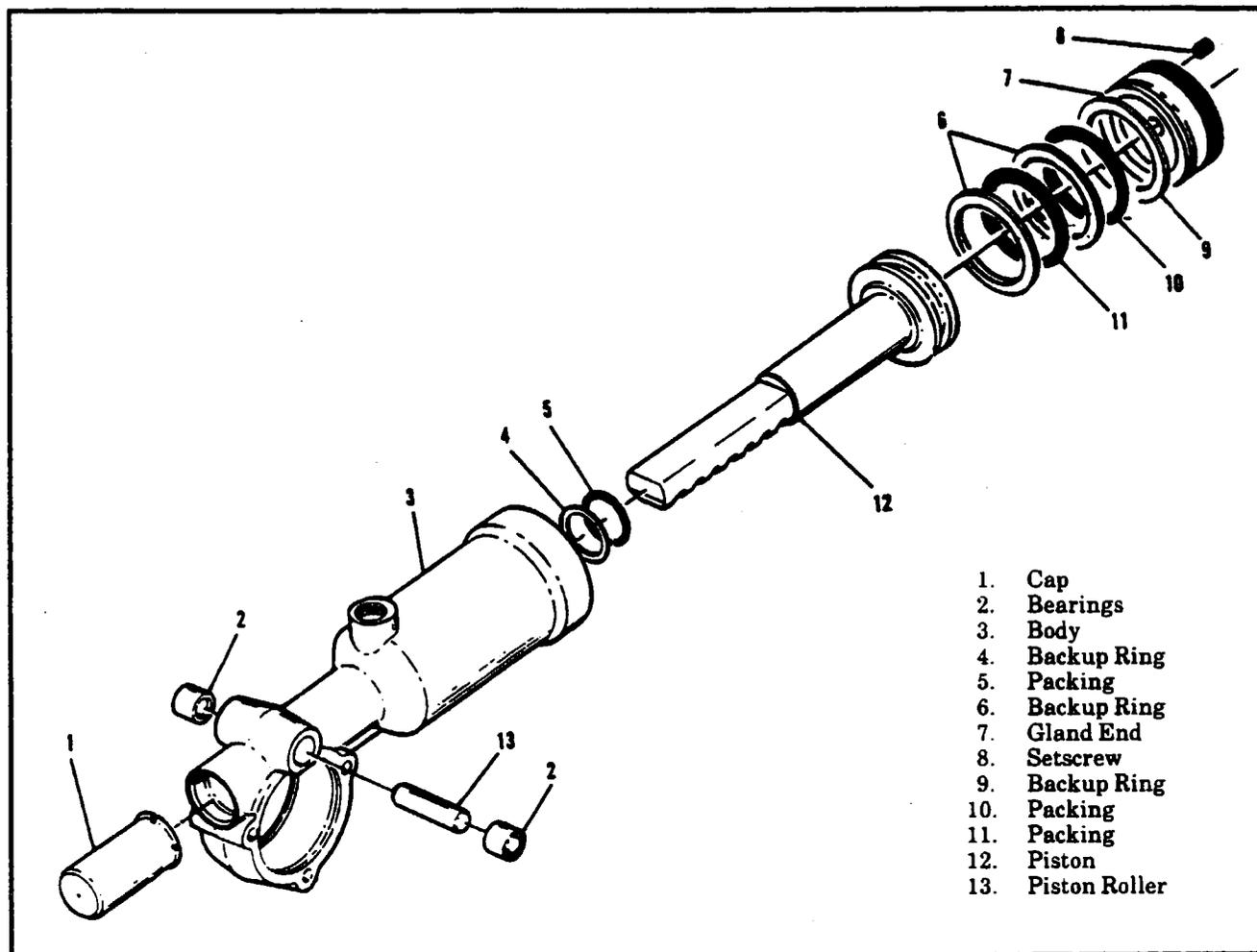
Figure 5A-12. Main Landing Gear Actuator
