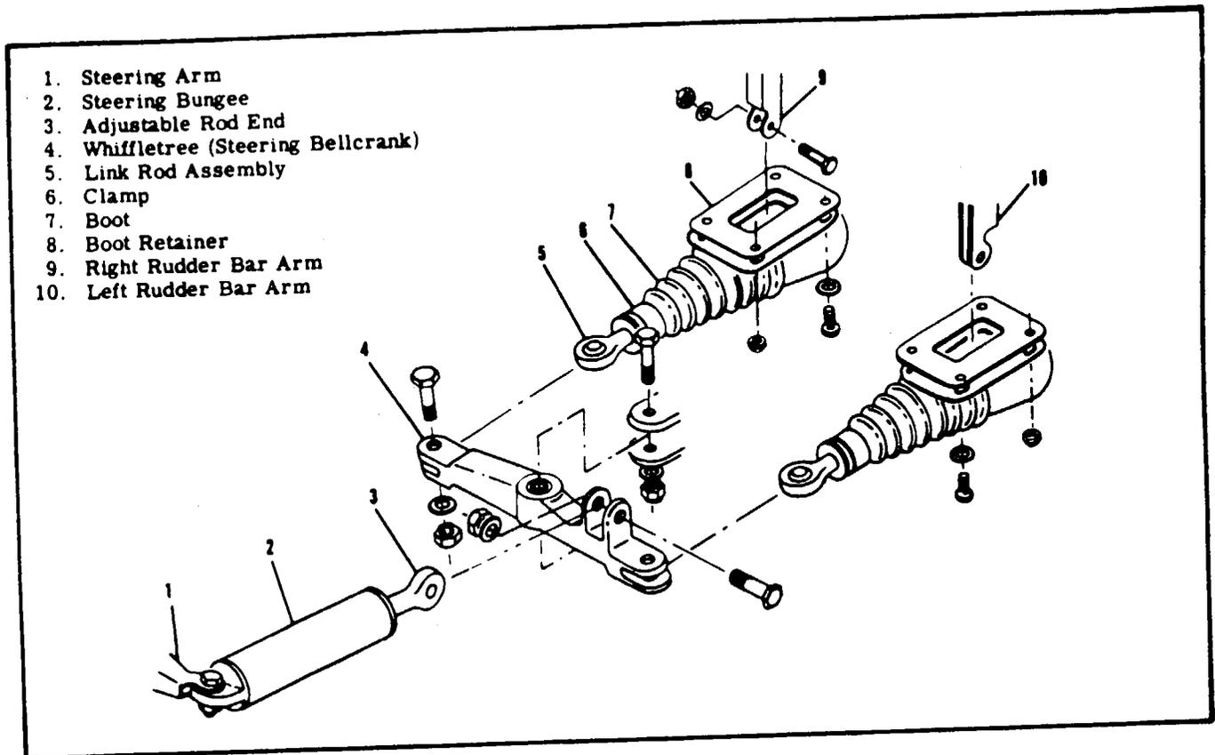
Figure 10-3. Nose Gear Steering Installation
