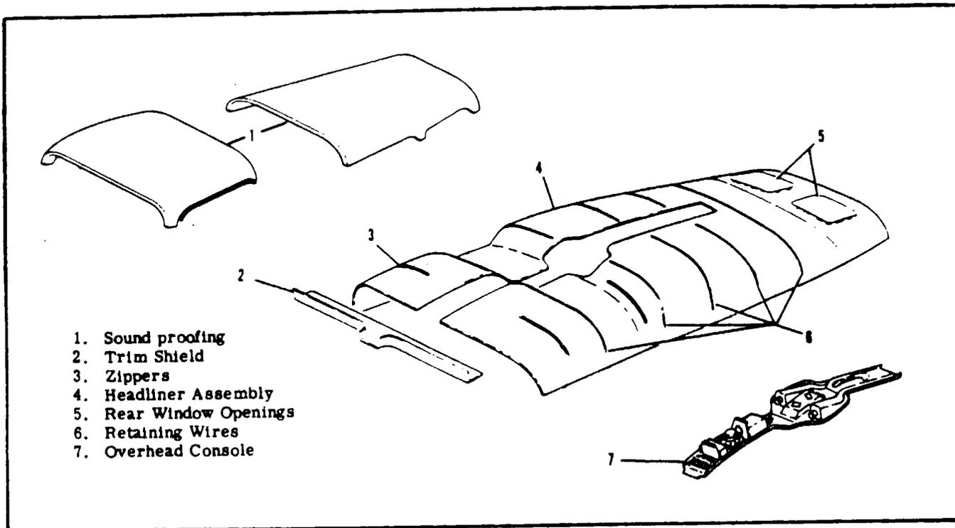
Figure 3-9. Cabin Headliner Installation
