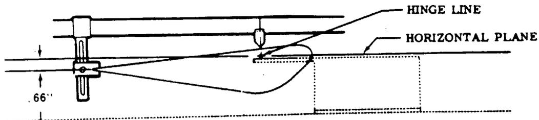
Balance aileron inverted, with trailing edge at point opposite cut-out for middle hinge .66" below hinge line horizontal plane.
