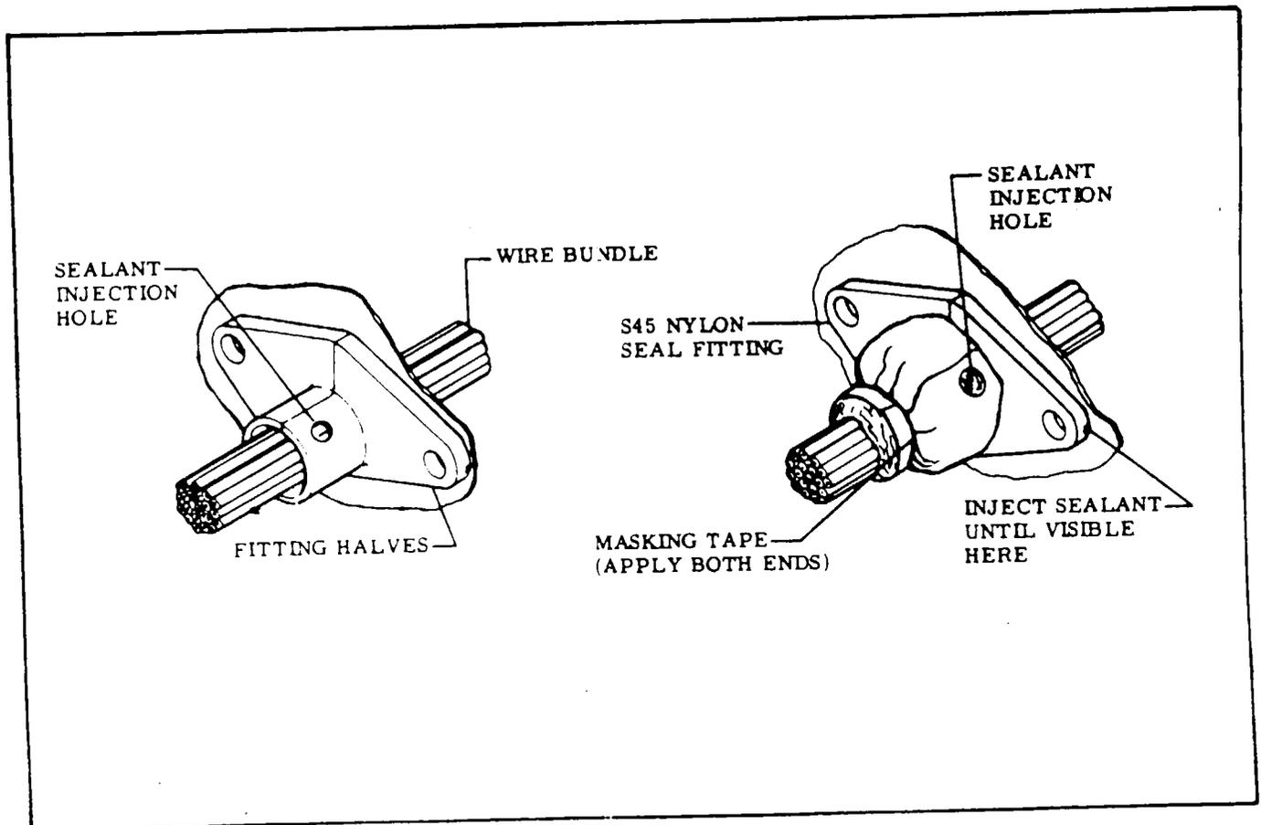
Figure 18-10. Electrical Sealing
