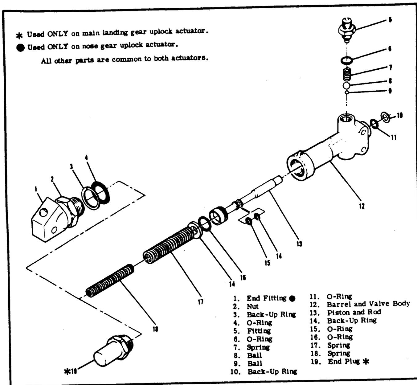
Figure 5-5. Lock and Unlock Actuators
