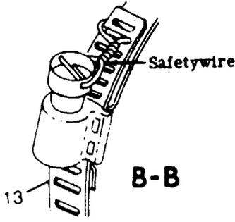
Hose clamp (13) screw housings to be installed 180° apart to maintain balance. Length of brushes from the slip ring to the brush block housing to be .063 ± .015 "
