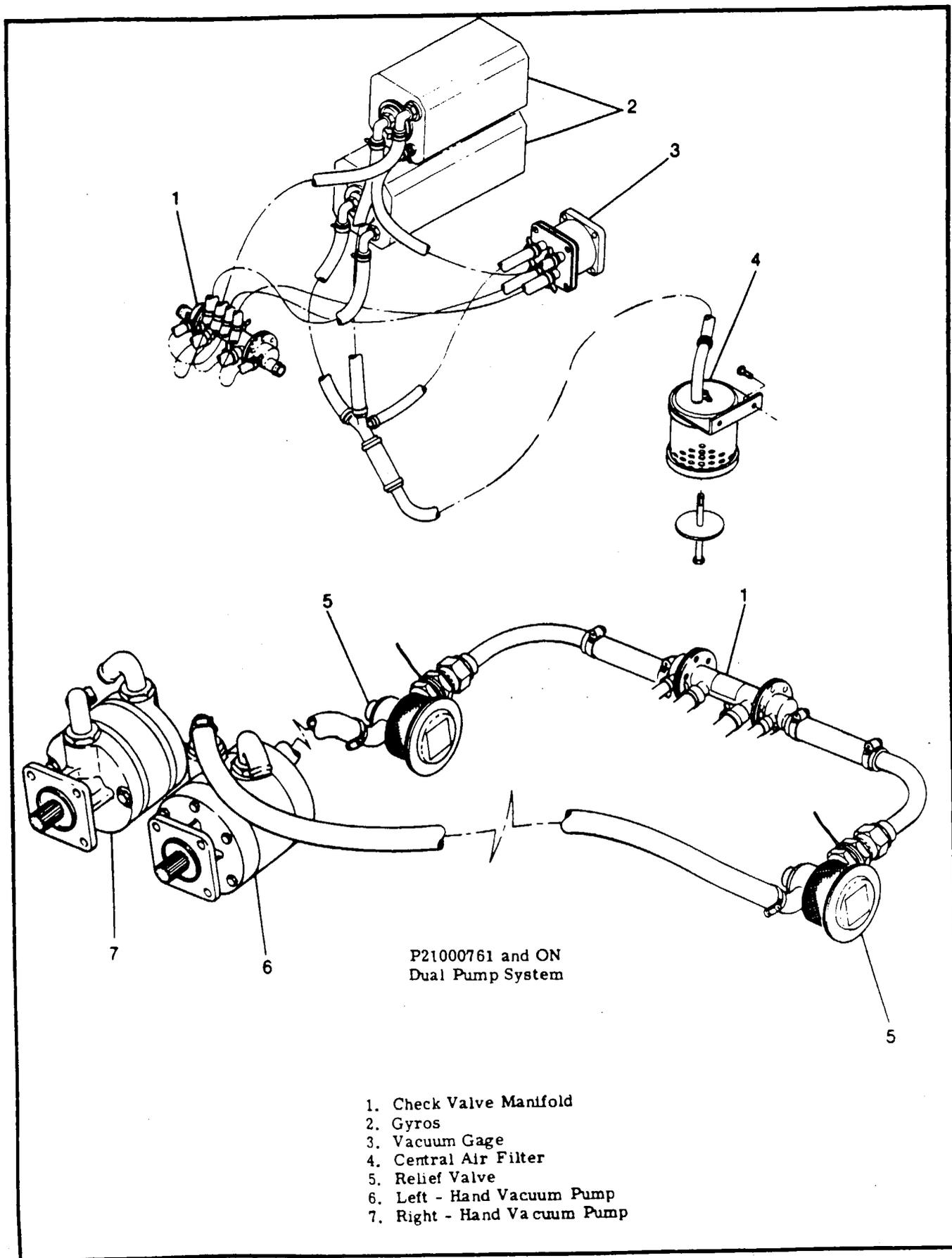
Figure 16-4. Vacuum System (Sheet 3 of 3)
