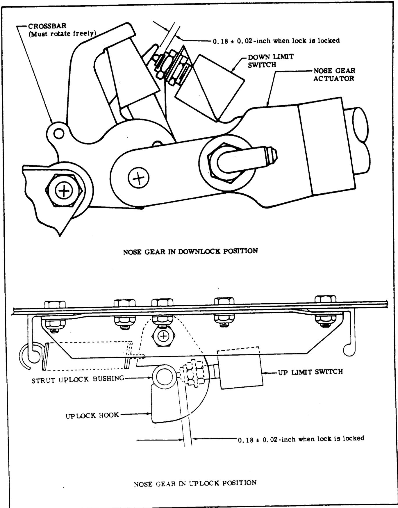
Figure 5-37. Rigging Nose Landing Gear
