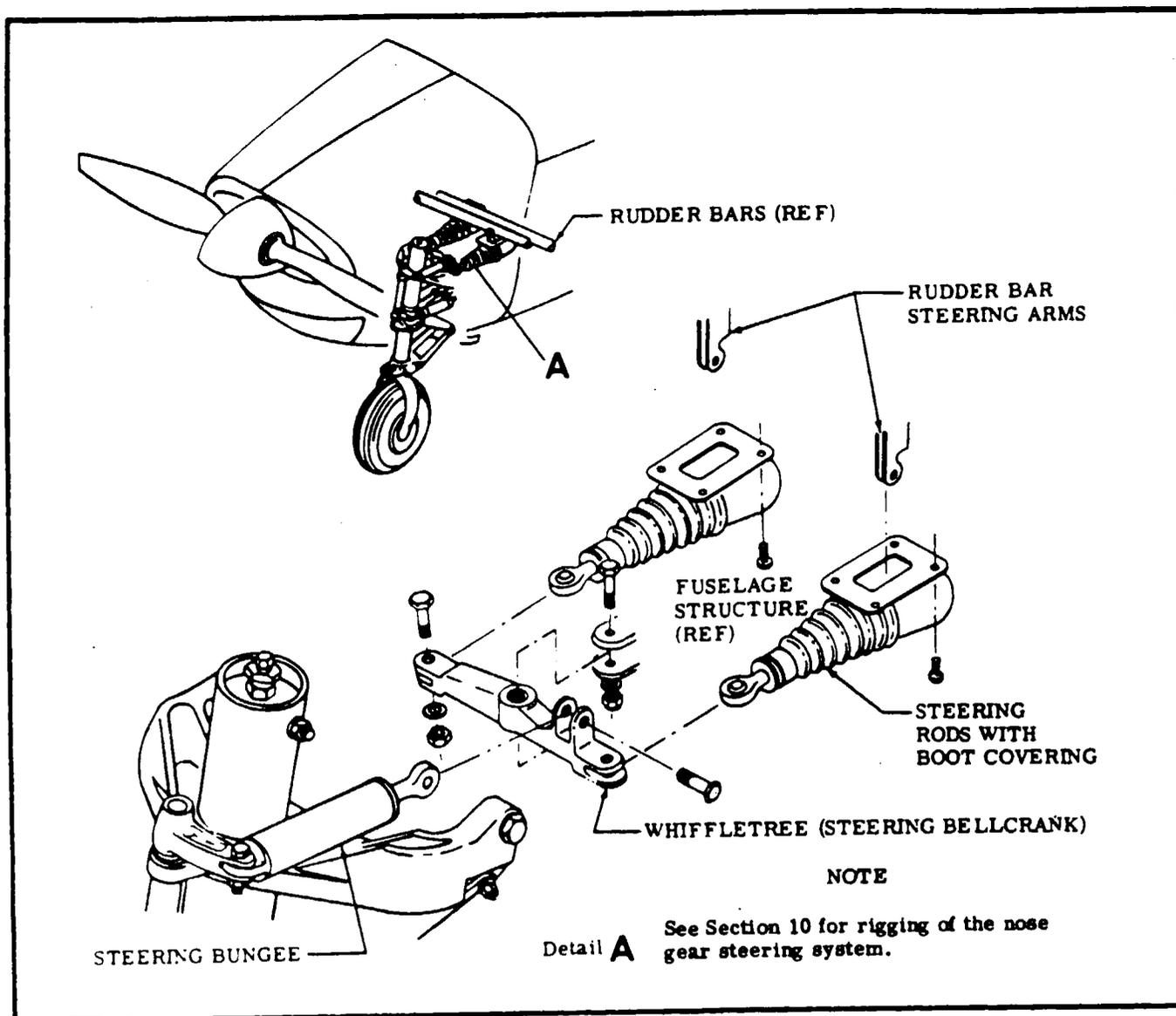
Figure 5-23. Nose Wheel Steering System
