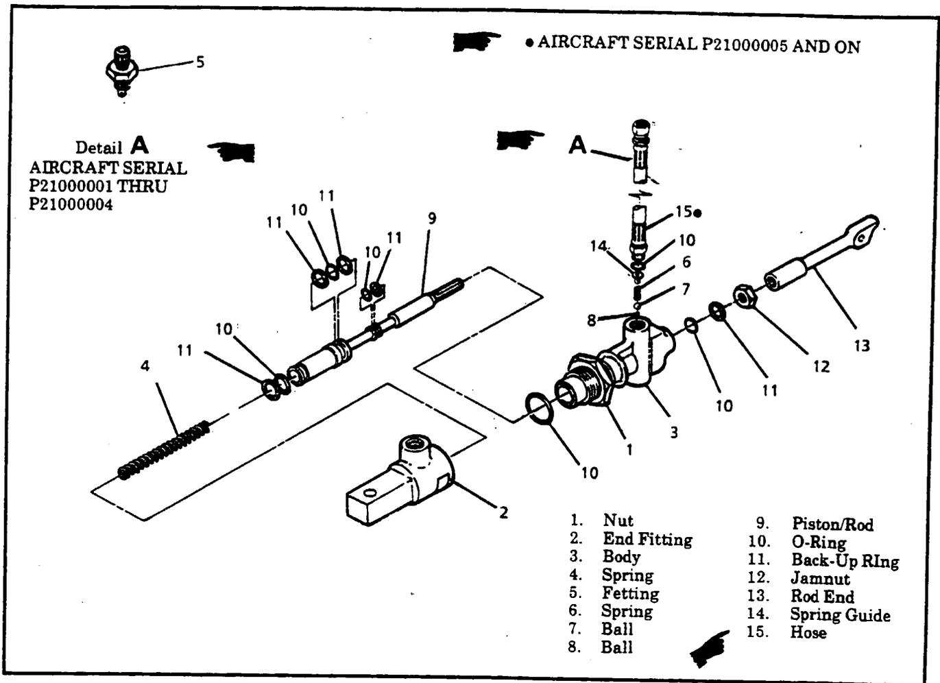
Figure 5-6A. Main Landing Gear Downlock Actuator.
