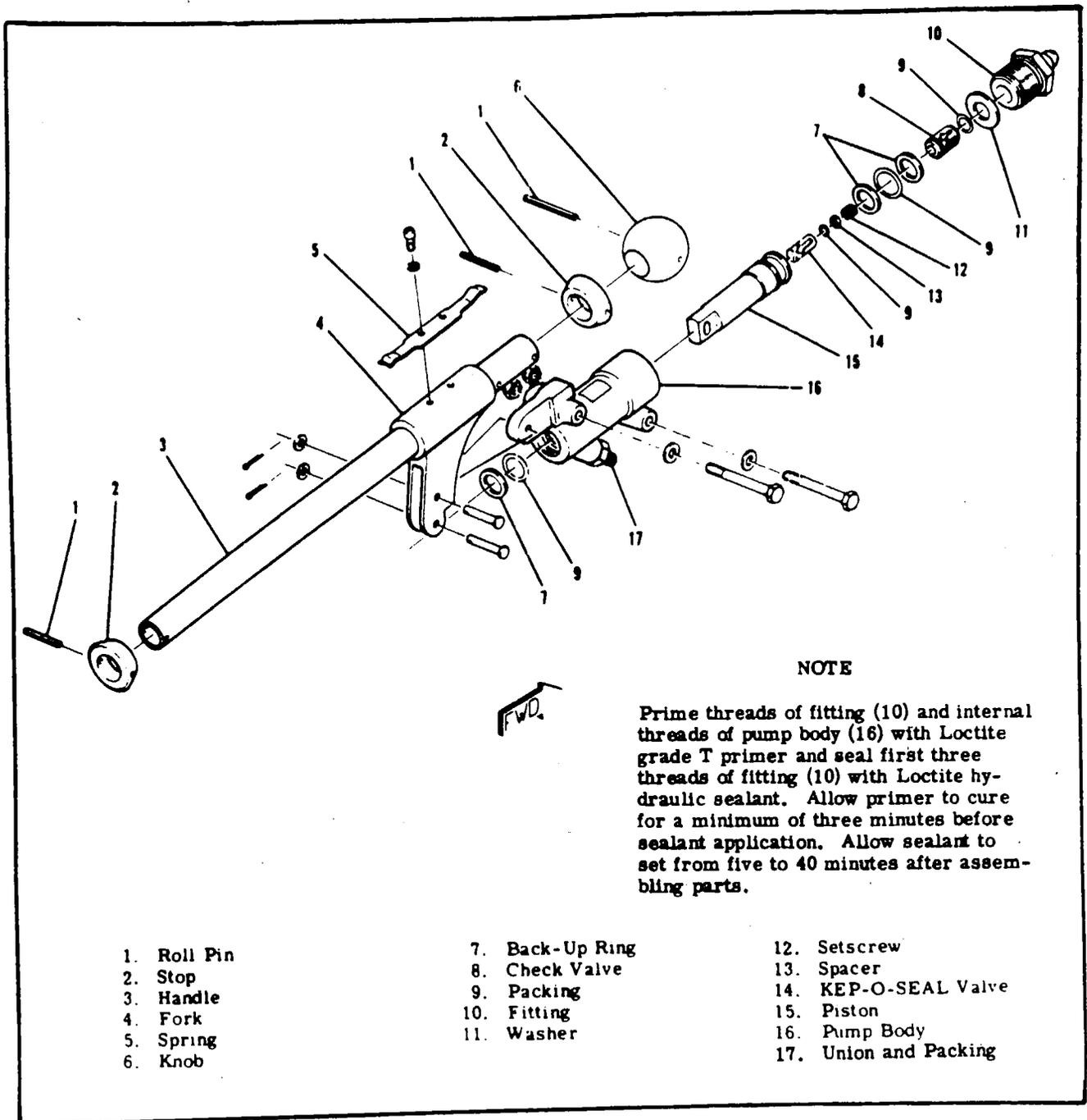
Figure 5A-6. Emergency Hand Pump Disassembly
