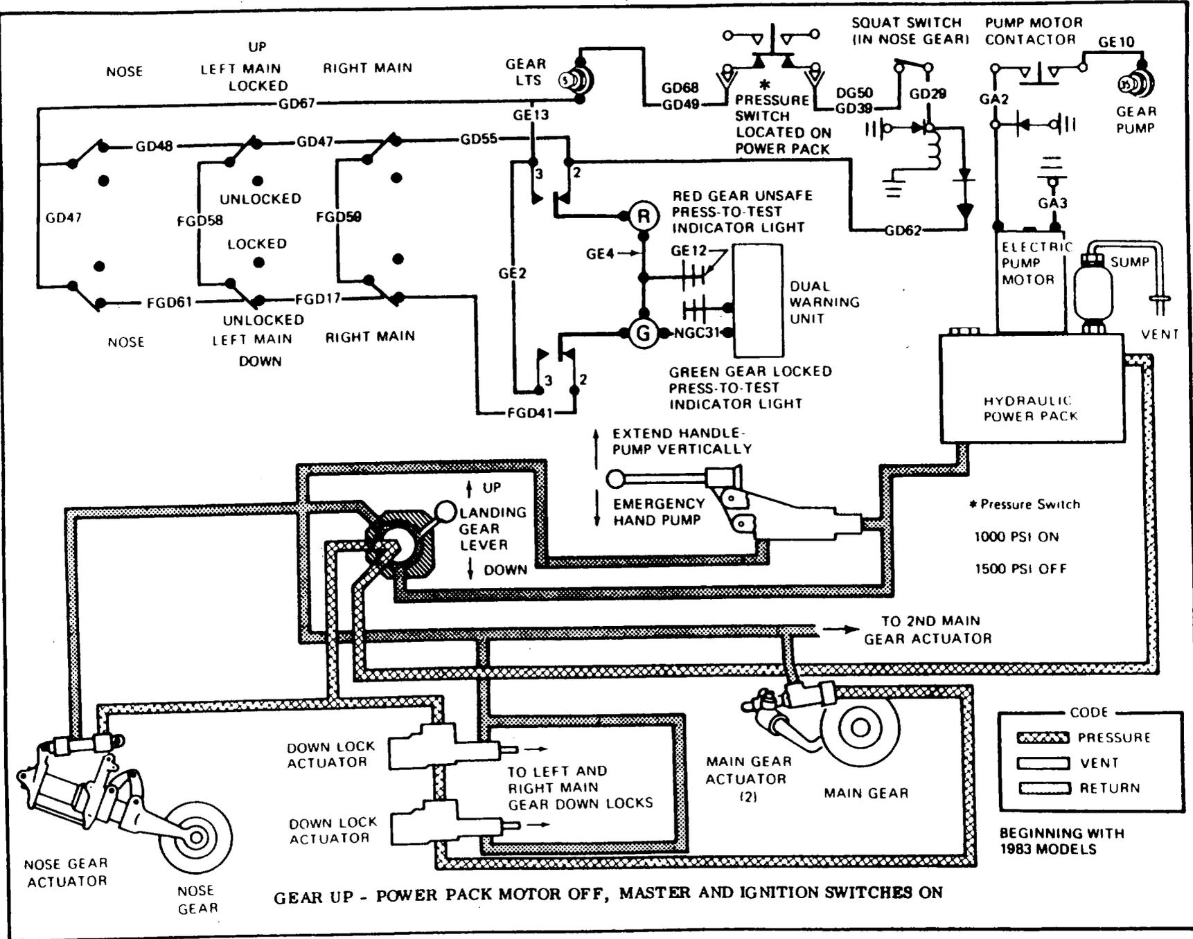
Figure 5A-1. Landing Gear Schematic (Sheet 4 of 4)
