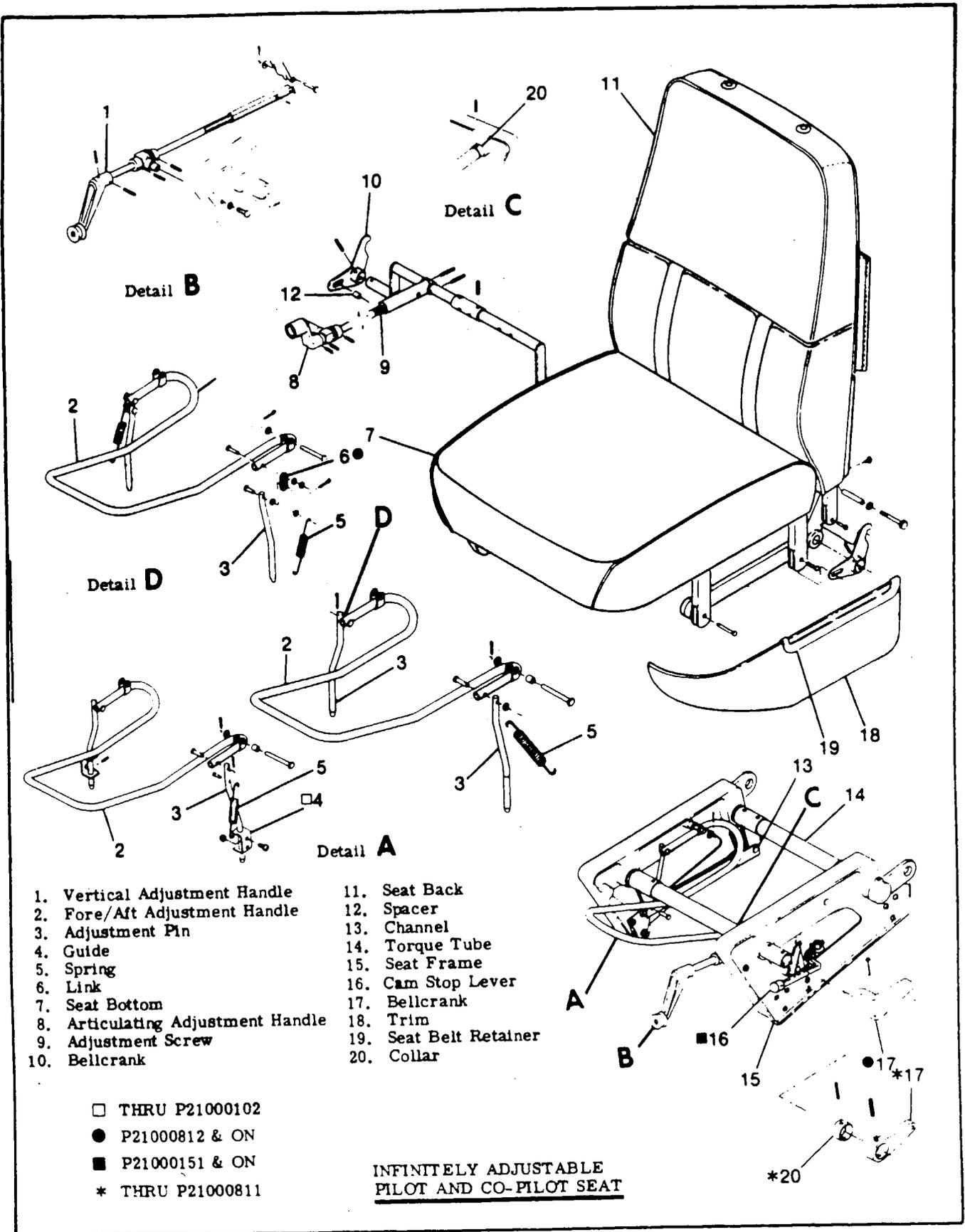
Figure 3-8. Seat Installation (Sheet 1 of 3)
