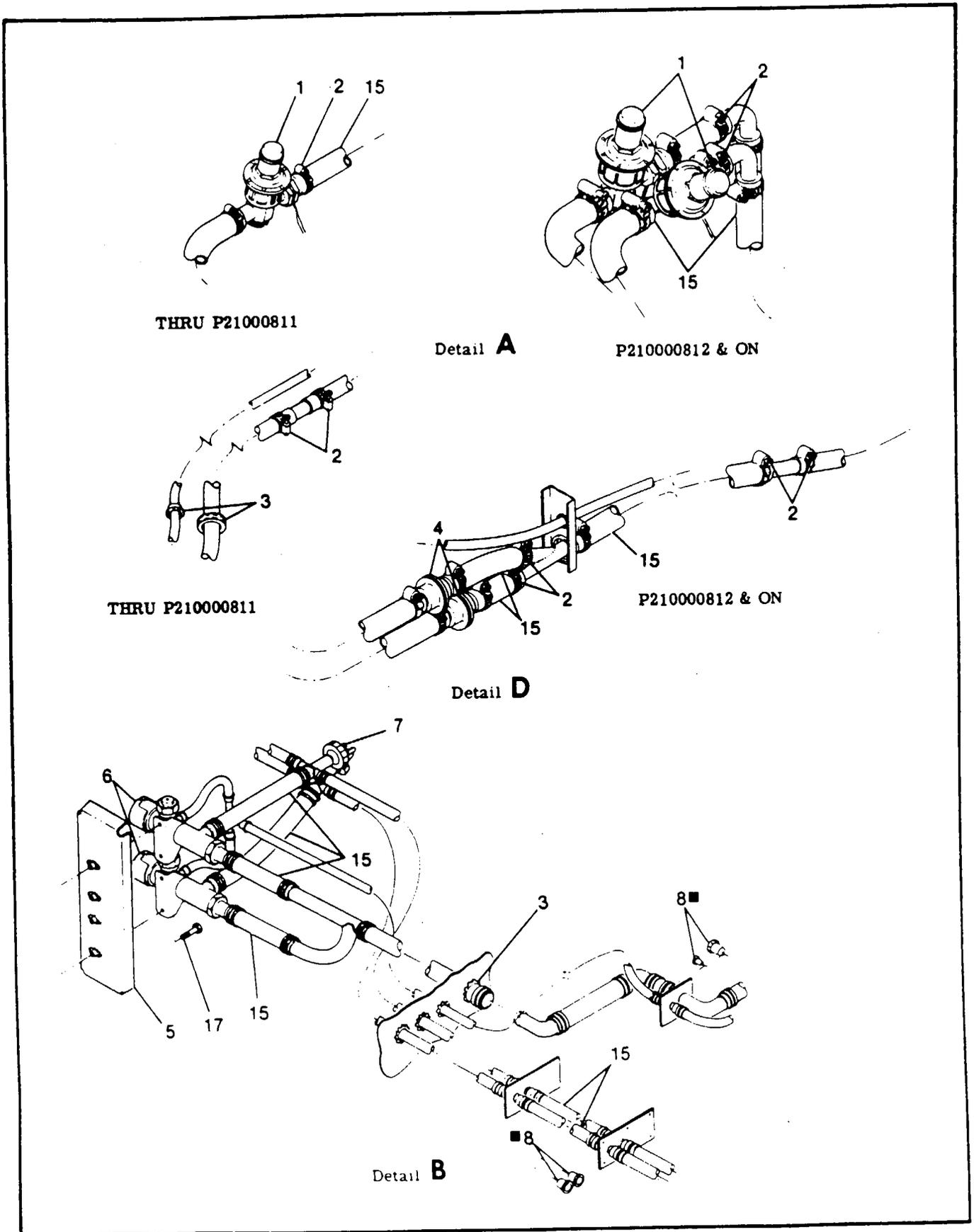
Figure 15-4A. Wing, Horizontal Stabilizer and Vertical Fin De-Icing System (Sheet 4 of 5)
