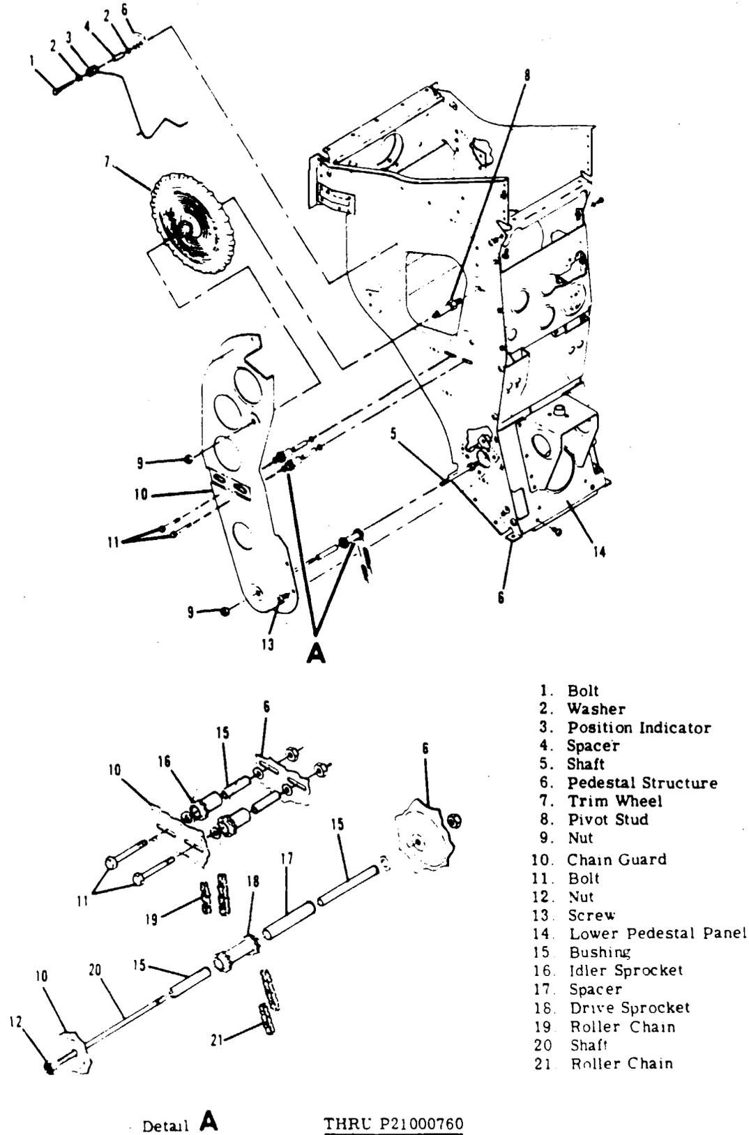
Figure 9-4. Elevator Trim Wheel Installation (Sheet 1 of 2)
