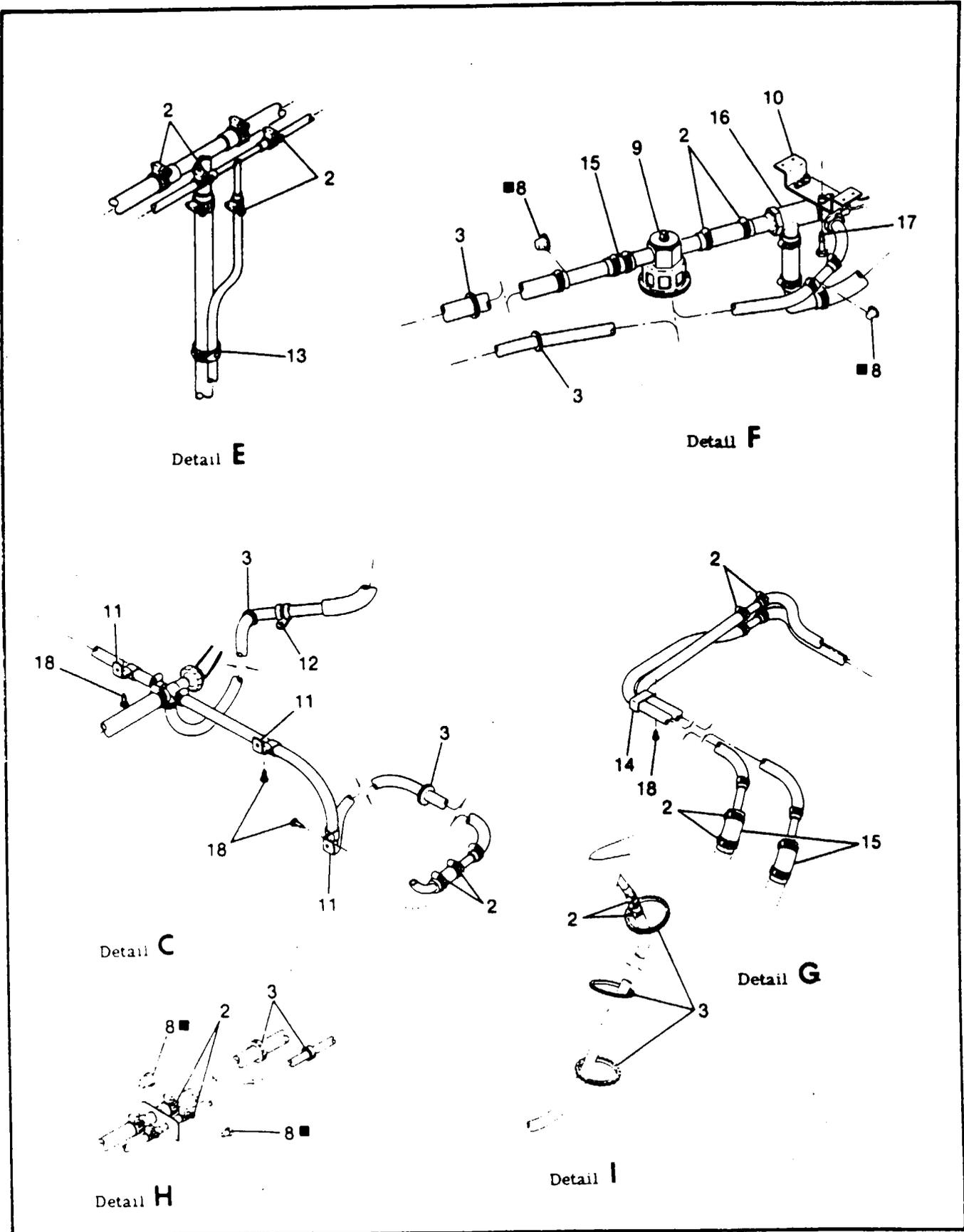
Figure 15-4A. Wing, Horizontal Stabilizer and Vertical Fin De-Icing System (Sheet 5 of 5)
