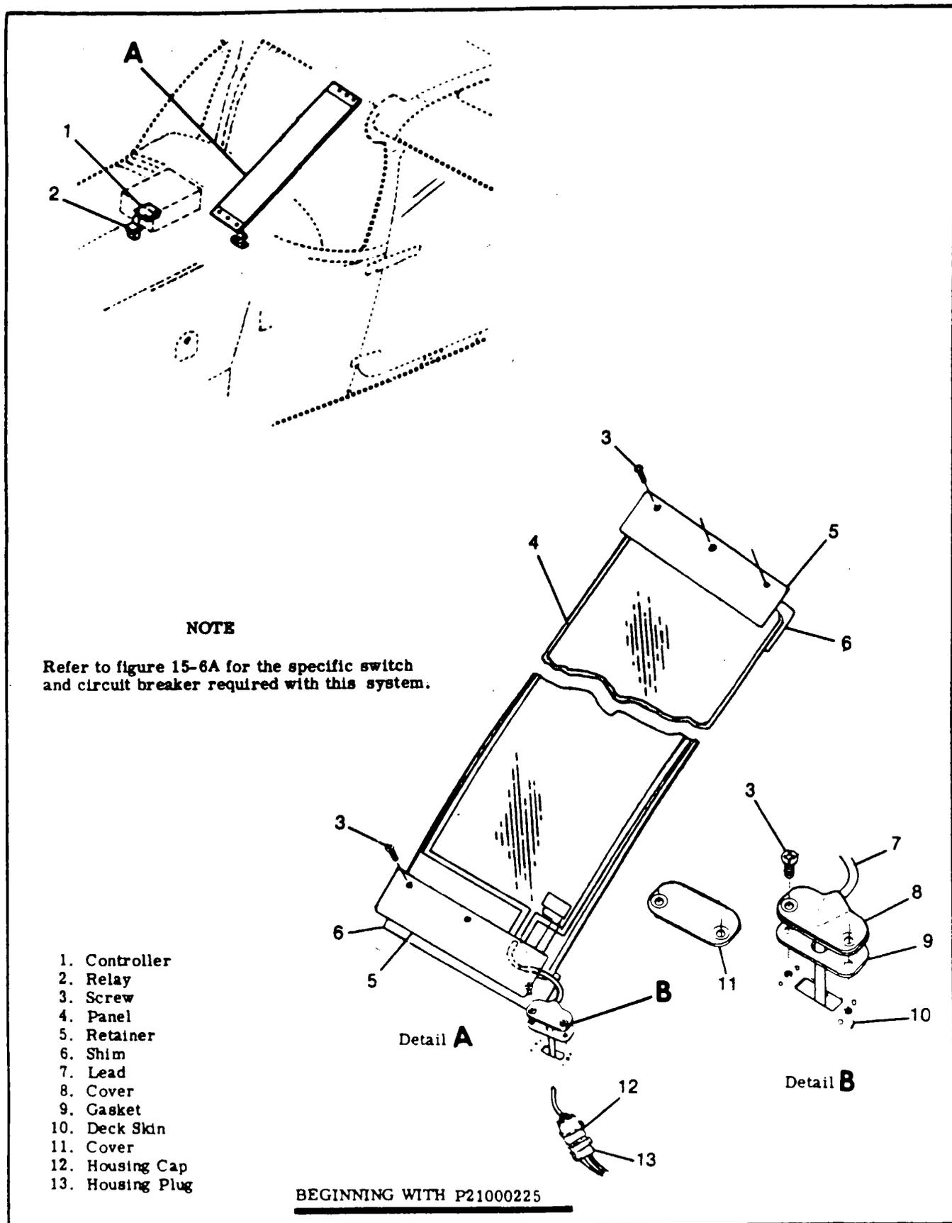
Figure 15-6C. Windshield Anti-Ice Panel Installation (Fixed)
