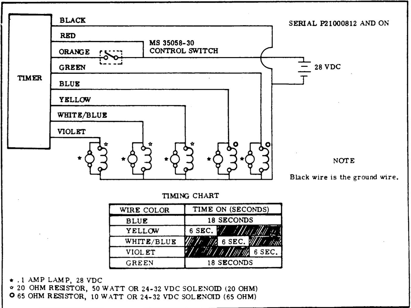
Figure 15-4E. Wing, Horizontal Stabilizer and Vertical Fin De-Ice System Timer.
