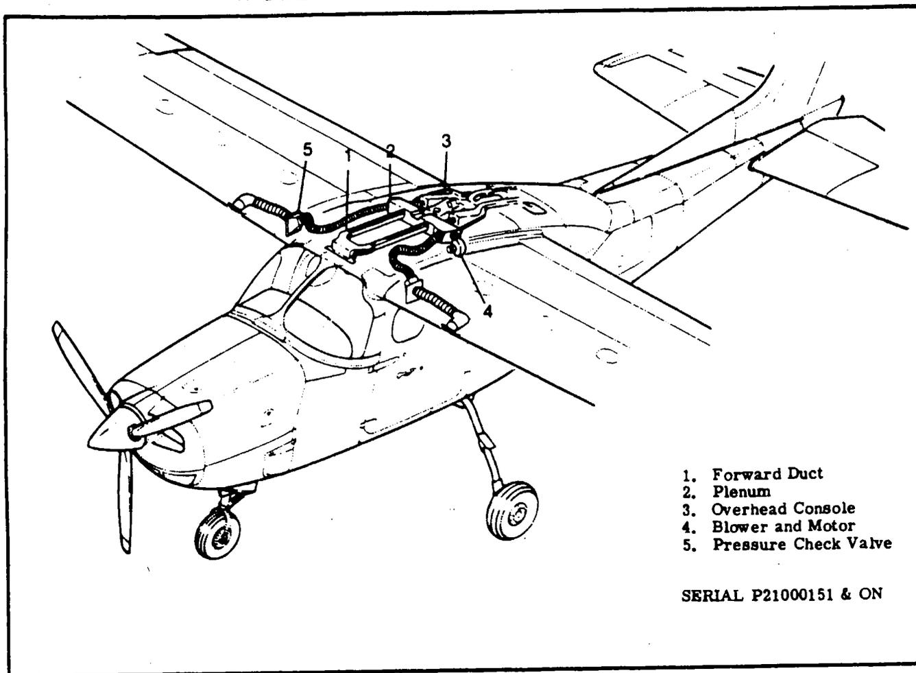
Figure 3-10. Ventilation System (Sheet 2 of 2)
