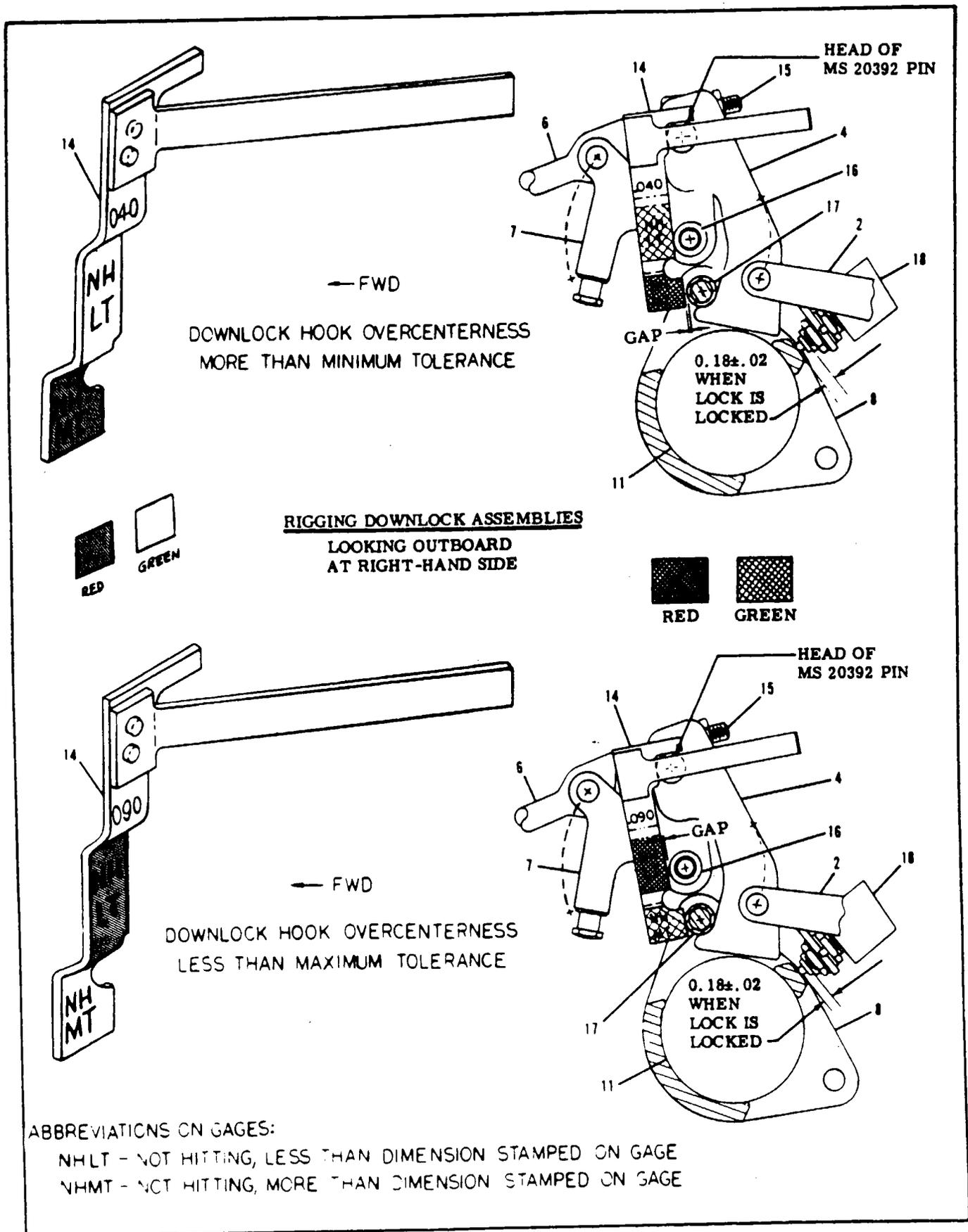
Figure 5-38. Rigging Main Landing Gear (Sheet 2 of 4)
