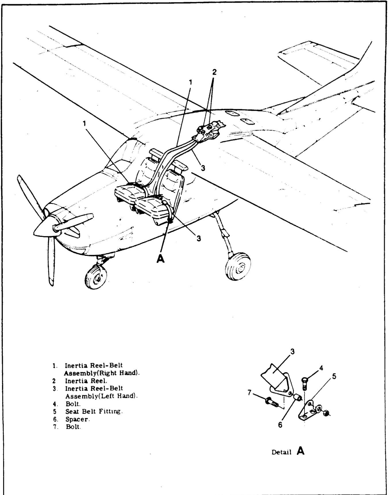
Figure 3-9B. Inertia Reel Harness
