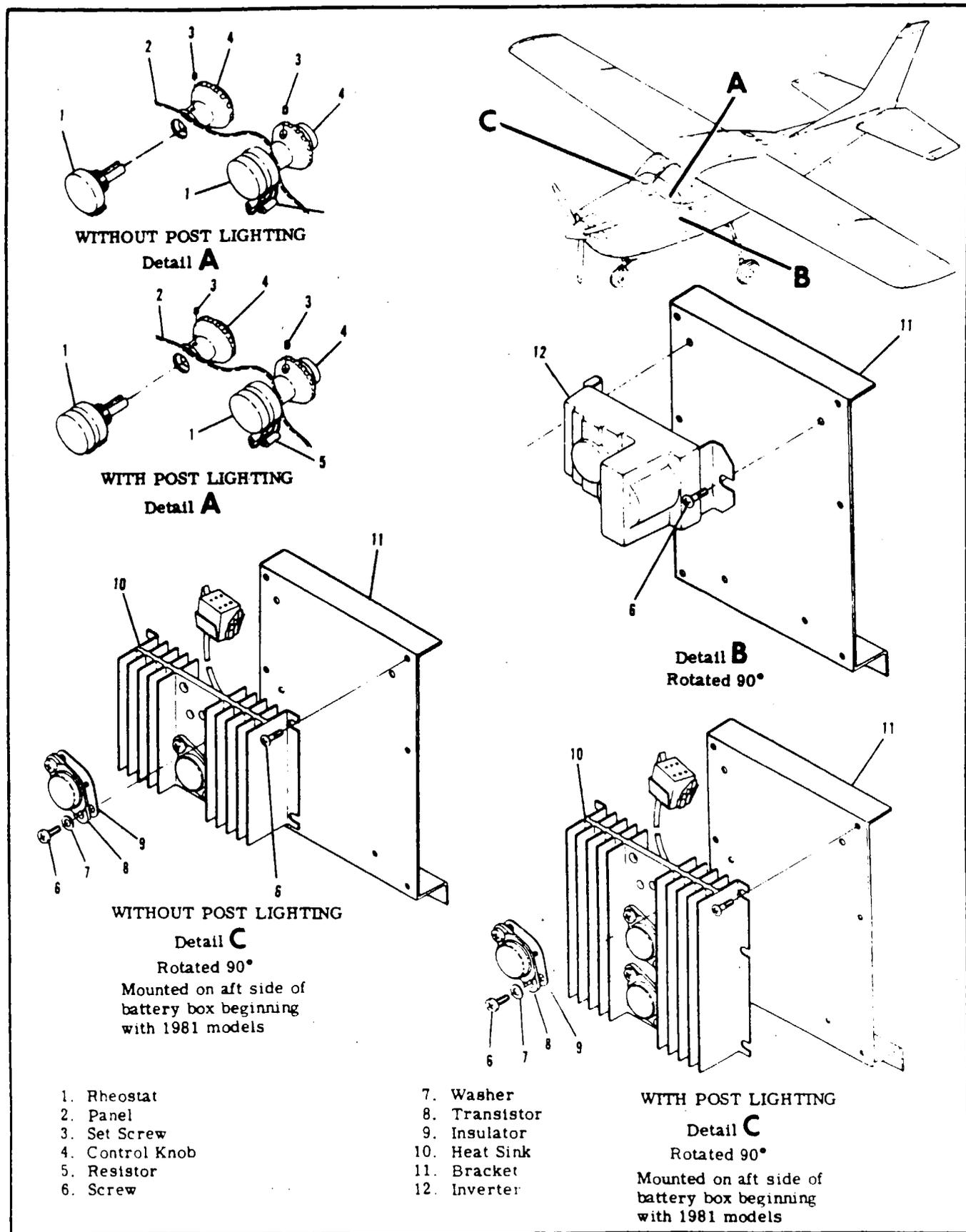
Figure 17-12. Transistorized Light Dimming and Electroluminescent Inverter Installation
