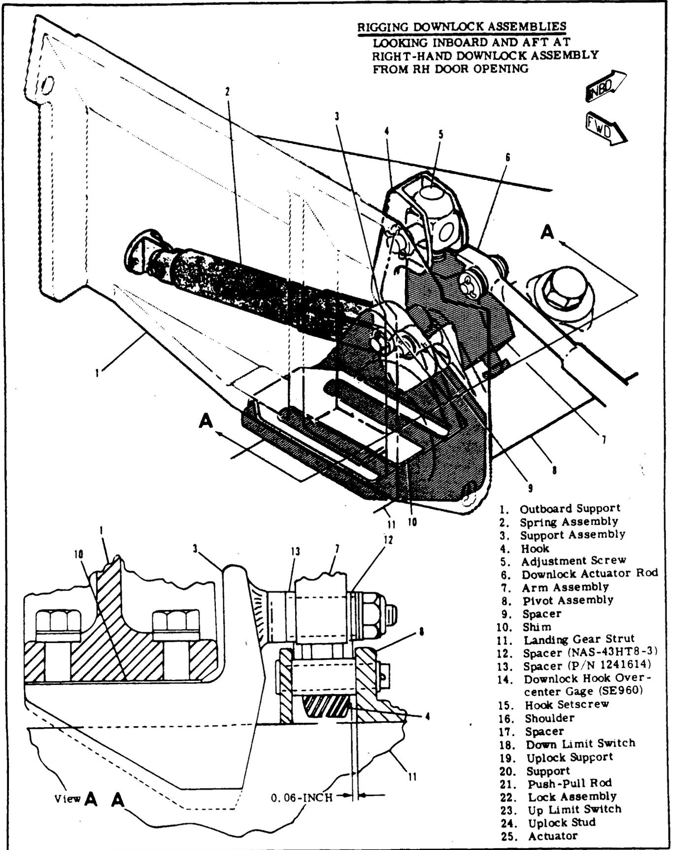
Figure 5-36. Rigging Main Landing Gear (Sheet 1 of 4)
