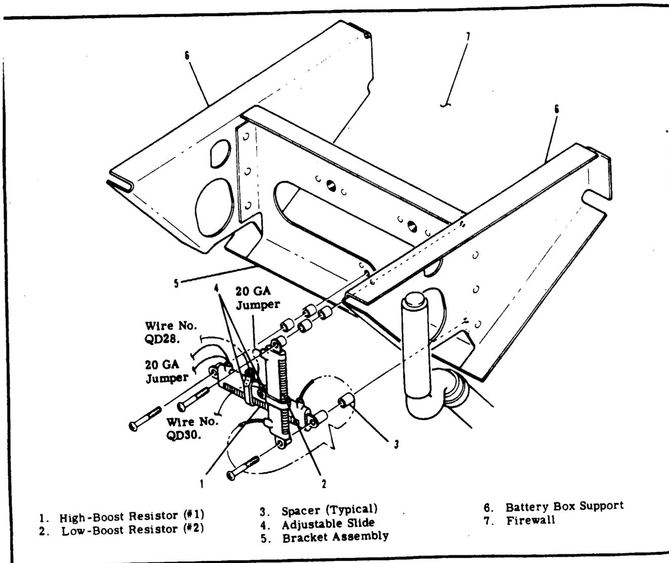
Figure 13-8. Auxiliary Fuel Pump Resistors
