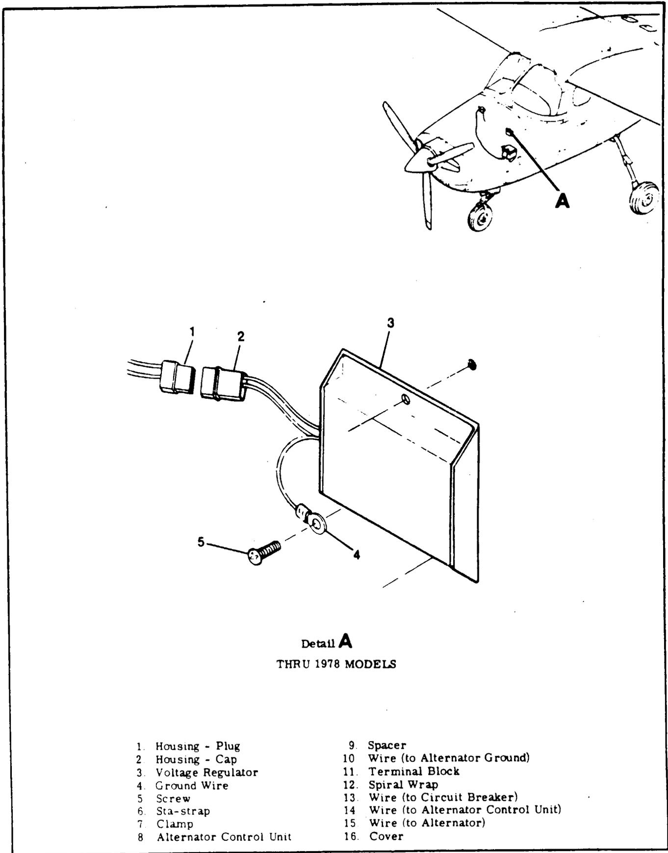
Figure 17-5. Voltage Regulator/Alternator Control Unit Installation (Sheet 1 of 3)
