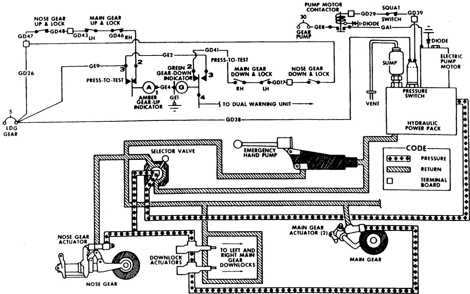
Figure 5A-1. Landing Gear Schematic (Sheet 2 of 4)
