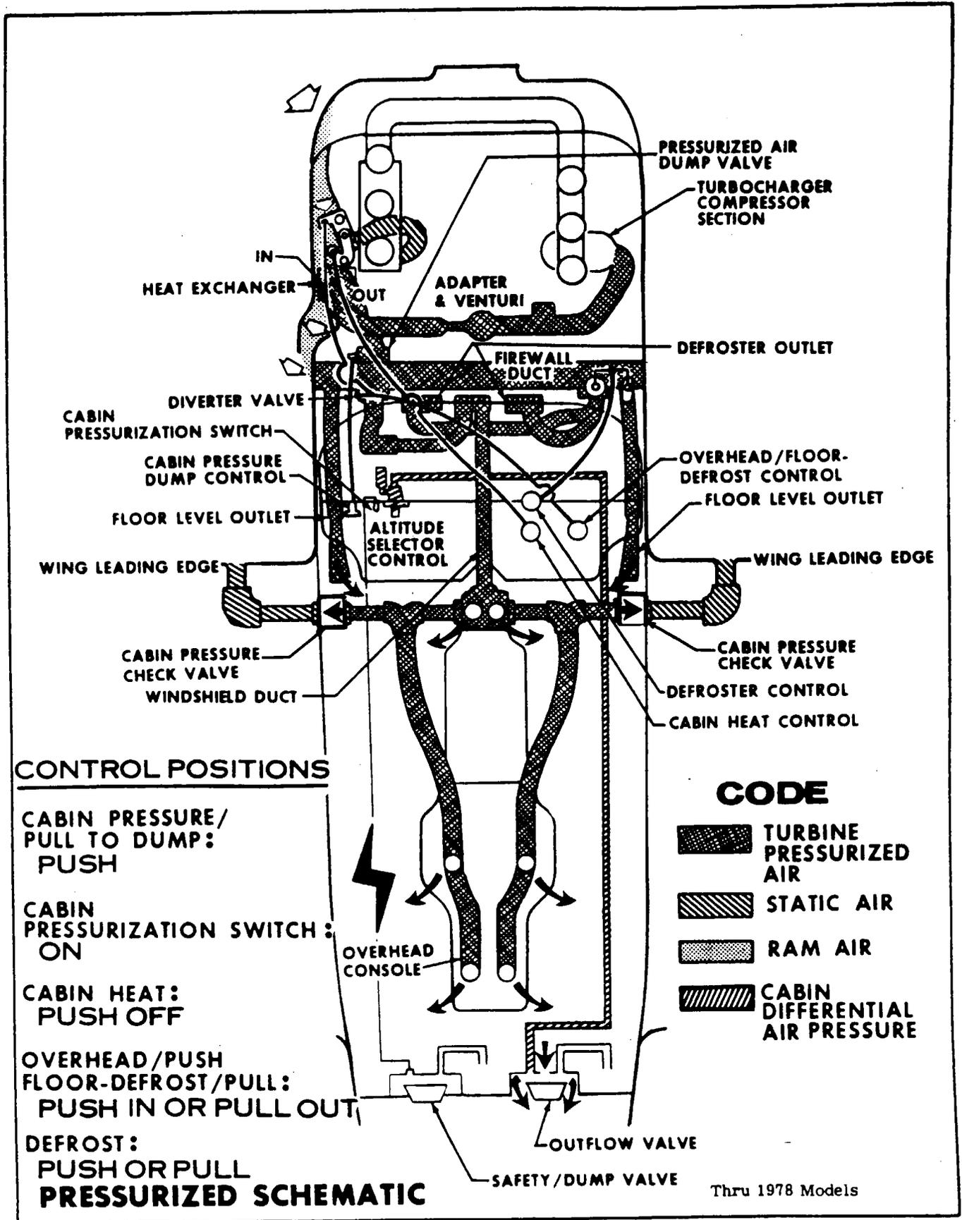
Figure 15-2. Cabin Air Flow Schematic (Sheet 2 of 6)
