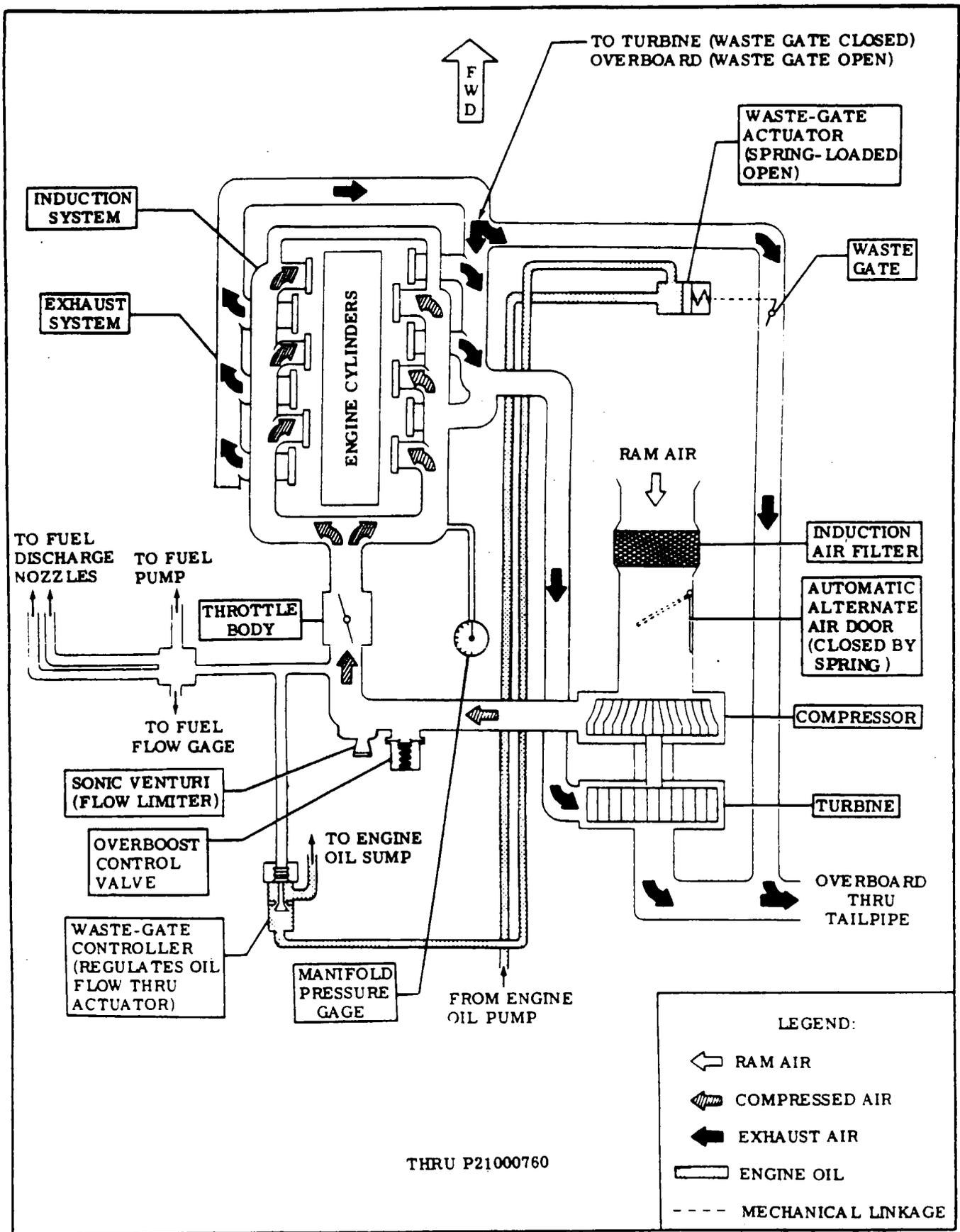
Figure 12-14. Turbocharger System Schematic ( Sheet 1 of 2 )
