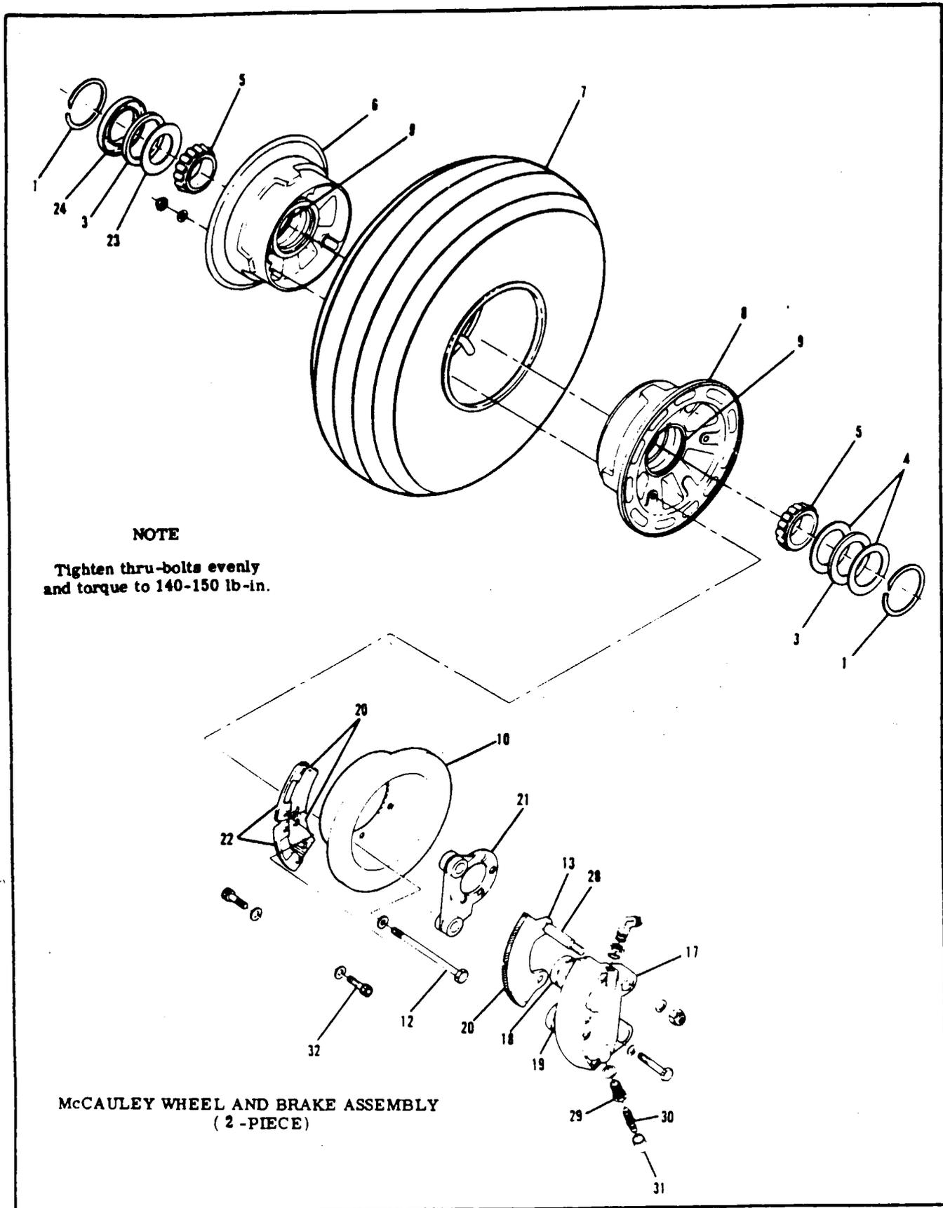
Figure 5-10 Main Landing Gear, Tire and Brake Assembly ( Sheet 2 of 3 )
