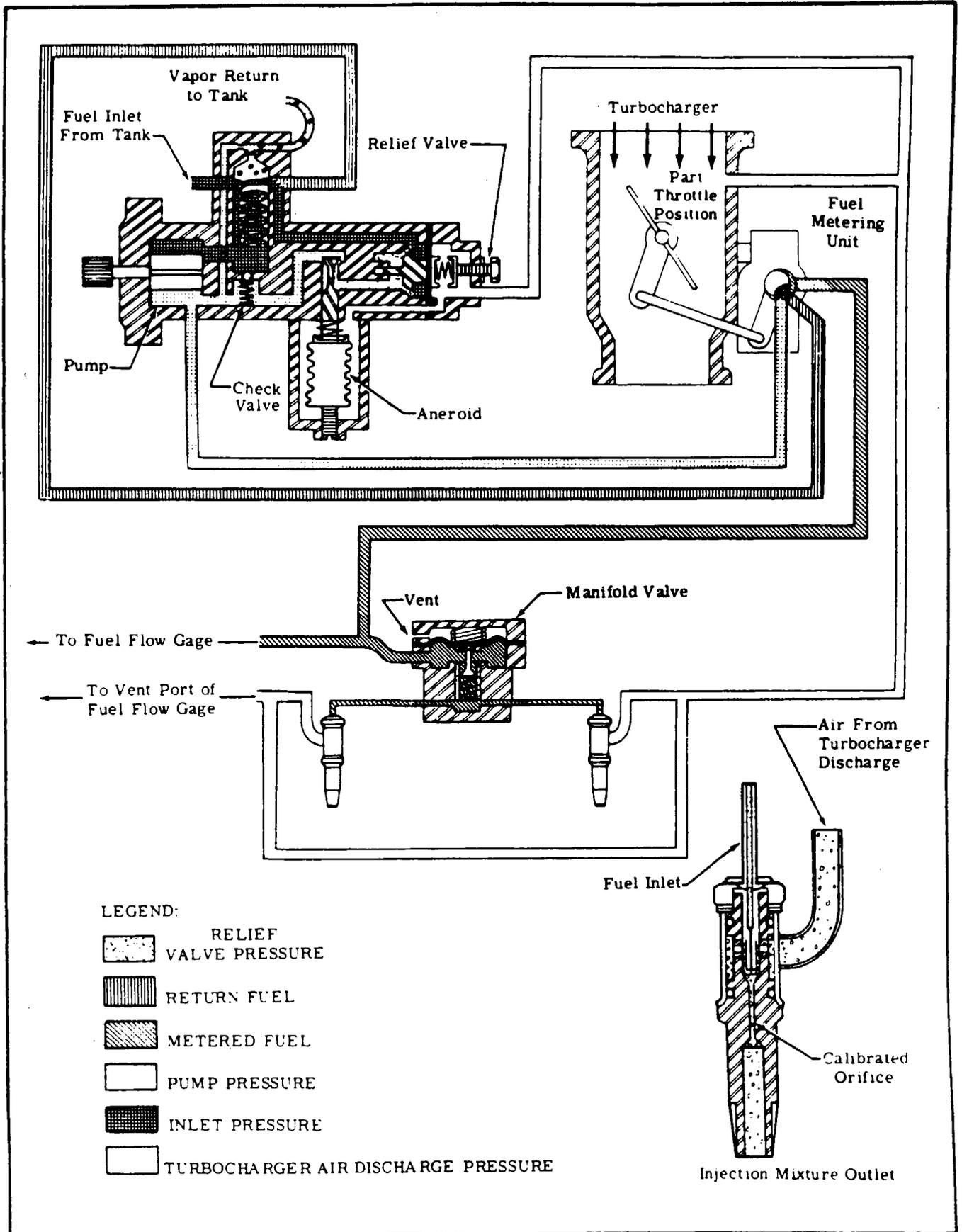
Figure 12-6. Fuel System Schematic
