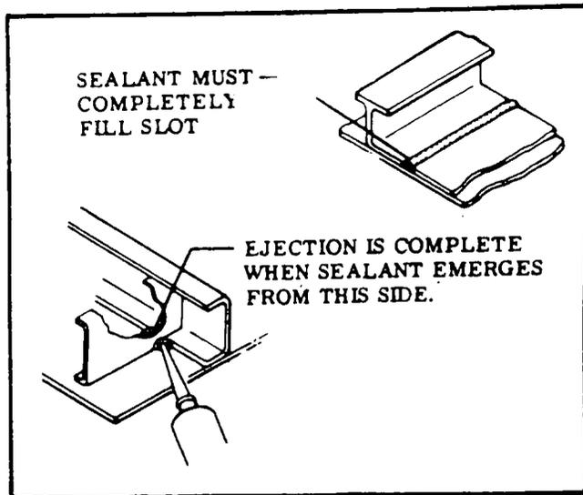
Figure 18-6. Injection Sealing
