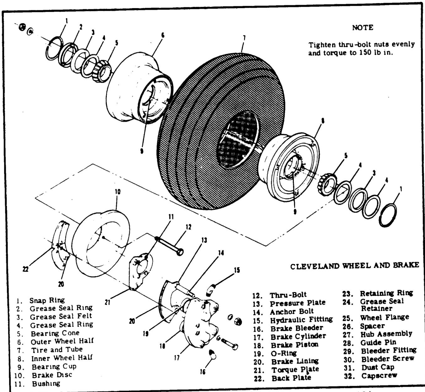
Figure 5-10 Main Landing Gear Wheel, Tire and Brake Assembly ( Sheet 1 of 3 )
