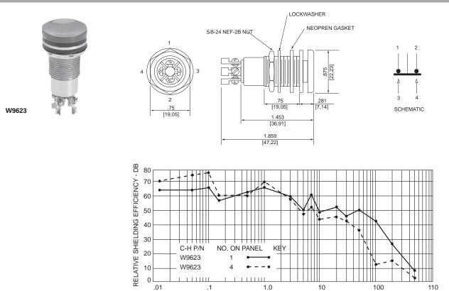
Graphic illustration defines relative shielding efficiency of RFI shielded component/ components over unshielded device.
