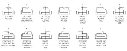
Figures A thru P do not represent details of construction. They schematically illustrate locking function.
