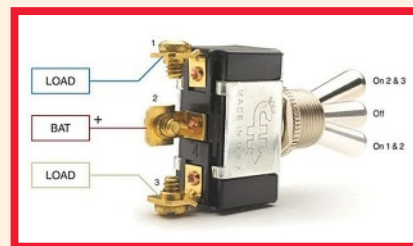
SPDT On-Off-On Only one of the loads can be energized at a time.
